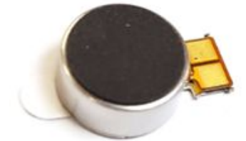
ELEC/MECH, VIBRATOR, MPLUS, LINEAR 1040, FPC TYPE, LV1040SC, 5a G710-02255-01
