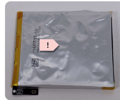
Swelling or electrolyte leakage
