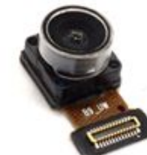
Rear Camera FPC Module Assembly, 5a (16M) G949-00146-01
