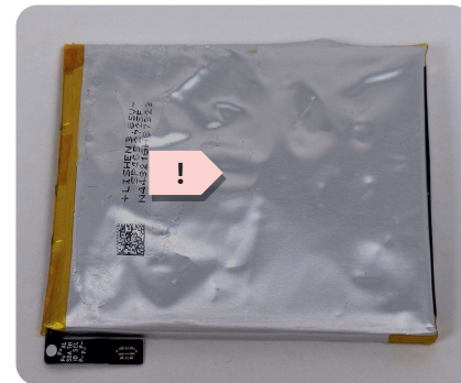
Swelling or electrolyte leakage
