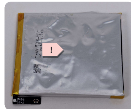
Swelling or electrolyte leakage
