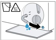
8. Firmly press on the sealing cap.
