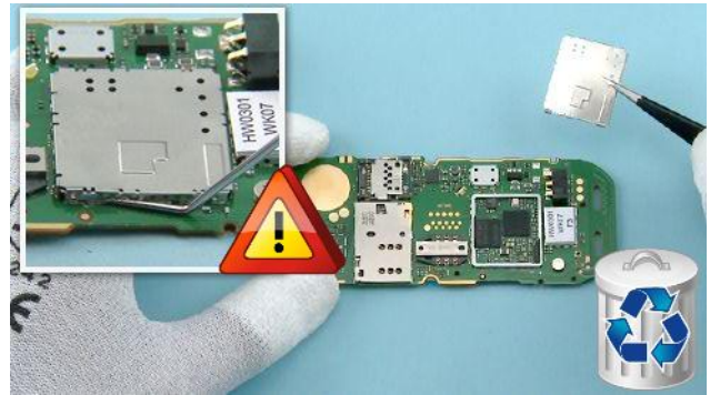
20) Lever out the BB SHIELDING LID with the dental tool and remove it with tweezers. Do not use it again. Discard it.
