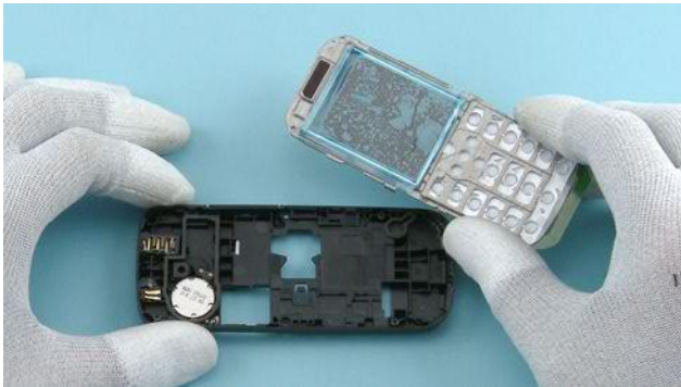
13) The ENGINE BOARD and the D-COVER can now be separated.
