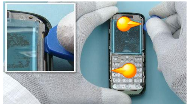
12) Open the two shown clips with the SRT-6 to release the ENGINE BOARD.
