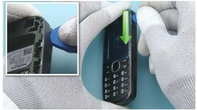
8) Release also the other side of the A-COVER with the SRT-6.
