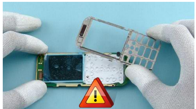
16) Separate the UI SHIELDING. Note that the DISPLAY is attached to the ENGINE BOARD only with the DISPLAY flex. Be careful not to damage the DISPLAY FLEX.
