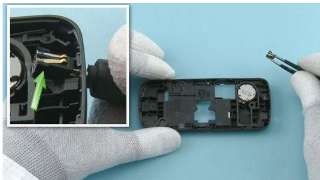
23) Lift up the DC JACK with a DC plug. Remove it with tweezers.
