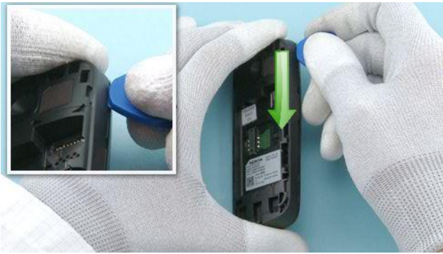
7) Use the SRT-6 to release the A-COVER. Start from the shown place and slide the SRT-6 towards the bottom end to release the side of the A-COVER.
