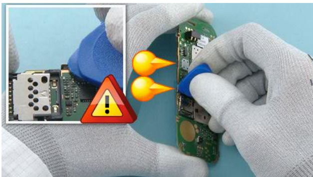
15) Open also the two shown clips on the other side. Be careful not to damage the small components on the ENGINE BOARD.
