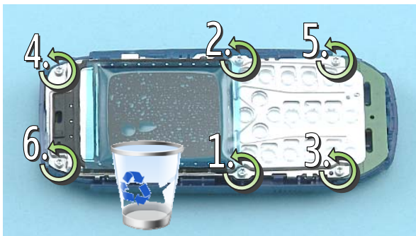
9) Unscrew the six TORX+ size 6 screws in the order shown. Do not use them again. Discard them.
