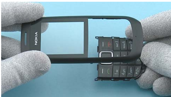
17) Separate the KEYMAT ASSY and the A-COVER ASSY by pushing out the KEYMAT ASSY.
