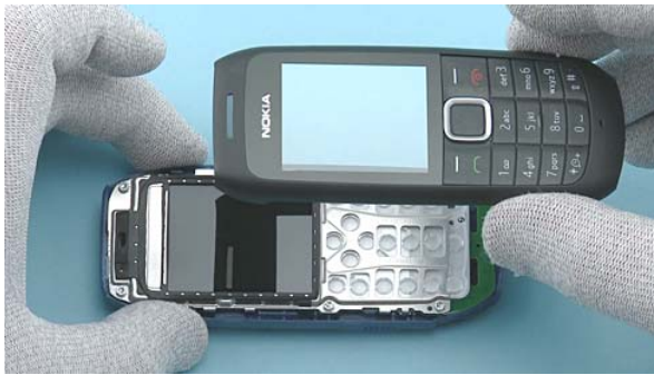
7) Remove the A-COVER ASSY.
