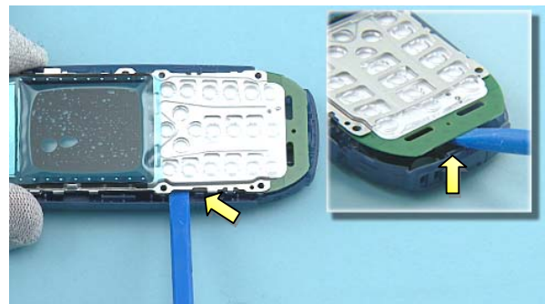
10) Lever out the ENGINE BOARD with the SS-93. Start from the left side of the device and continue on the bottom side.
