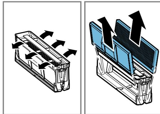
**2. Place the individual components of the grease filter loosely in the dishwasher and do not jam them in.**
