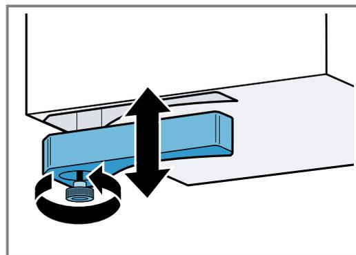
**2. Empty the overflow container and rinse it out.****3. If required, unscrew the screw and clean the overflow container without the screw in the dishwasher.**
