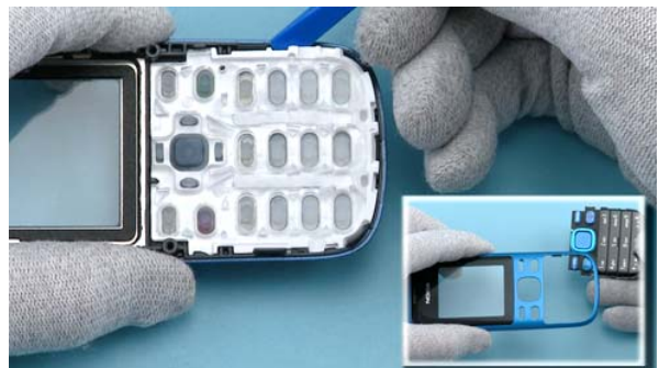
12) Use the SS-93 to separate the KEYMAT from the A-COVER.
