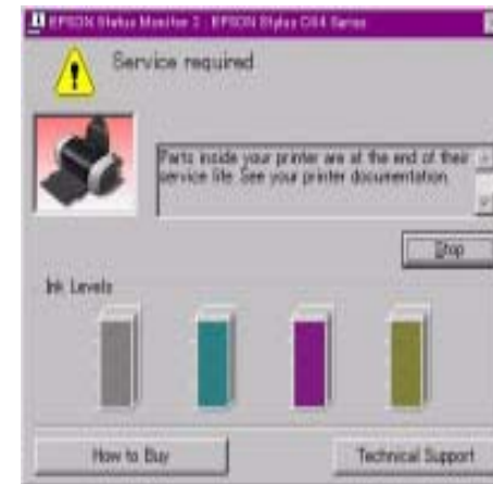
Figure 3-3. Maintenance error indication in STM3
