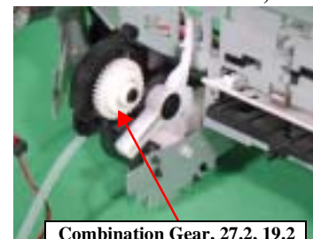
Figure 2-17. "Spur Gear, 36.8" and "Combination Gear, 27.2, 19.2"
