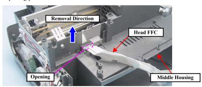
Figure 4-80. Removing the Middle Housing (2)
