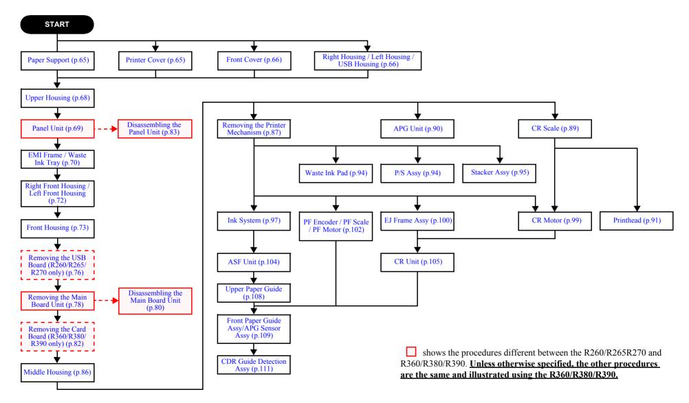
Flowchart 4-1. R260/R265/R270 & R360/R380/R390 Disassembly Flowchart
