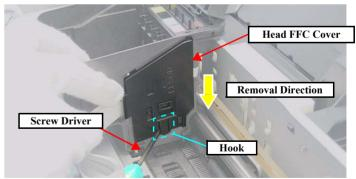
Figure 4-95. Removing the Head FFC Cover
