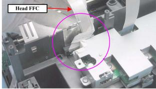
Figure 4-66. Routing the Head FFC (1)
