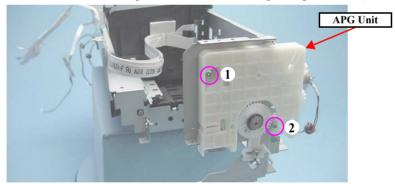
Figure 4-90. Removing the APG Unit
