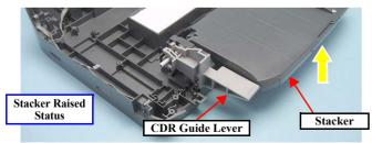
Figure 4-83. Cautions on Removing the Printer Mechanism
