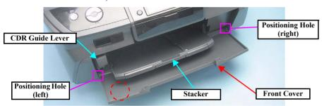
Figure 4-15. Removing the Front Cover (1)
