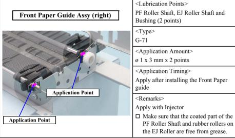
Figure 6-5. Lubrication of Front Paper Guide Assy (2)
