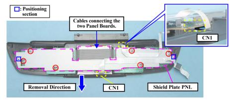
Figure 4-69. Removing the Panel Board (2)
