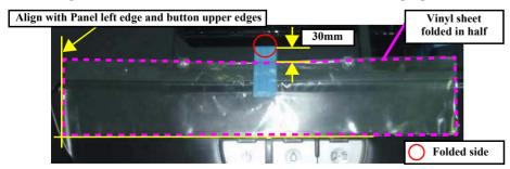
Figure 4-6. Protecting the Panel Unit (R260/R265/R270 only)
