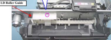
Figure 4-139. Removing the LD Roller Guide (1)
