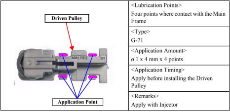
Figure 6-1. Lubrication of Driven Pulley (1)
