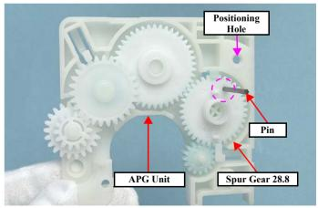
Figure 4-92. Reinstalling the APG Unit (2)
