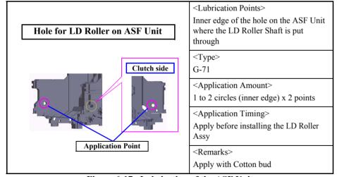
Figure 6-17. Lubrication of the ASF Unit
