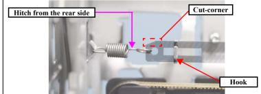
Figure 4-89. Reinstalling the CR Scale
