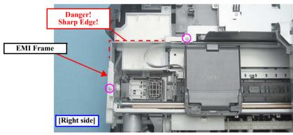
Figure 4-26. Removing the EMI Frame
