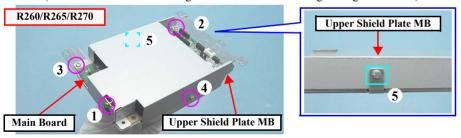
Figure 4-62. Removing the Upper Shield Plate MB (R260/R265/R270)
