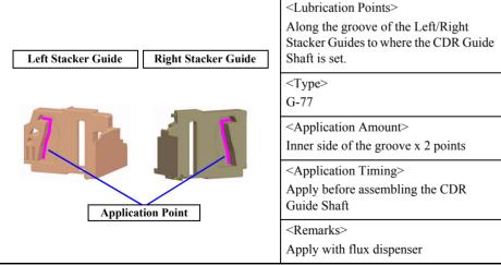
Figure 6-21. Lubrication of the Stacker Guides
