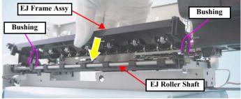
Figure 4-131. Reinstalling the EJ Frame Assy
