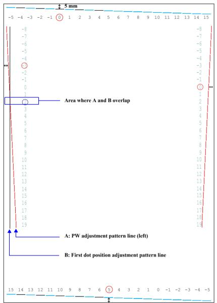
Figure 5-5. Left Right margin adjustment Pattern Printing
