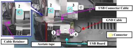
Figure 4-44. Removing the USB Board
