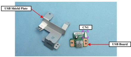
Figure 4-45. Disassembling the USB Board
