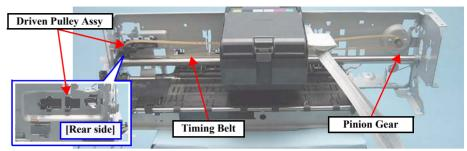
Figure 4-122. Removing the CR Motor (1)
