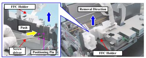
Figure 4-47. Removing the FFC Holder (1)
