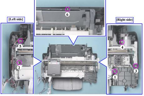
Figure 4-86. Removing the Screws (Printer Mechanism)
