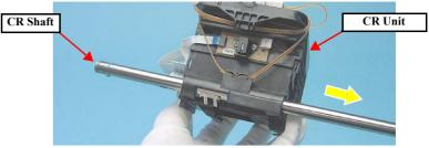
Figure 4-148. Removing the CR Unit (4)
