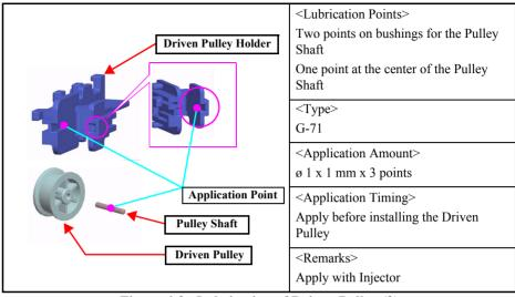
Figure 6-2. Lubrication of Driven Pulley (2)
