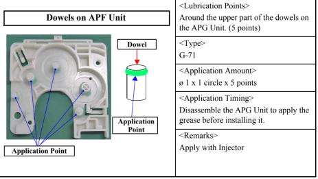
Figure 6-15. Lubrication of the APG Unit (1)
