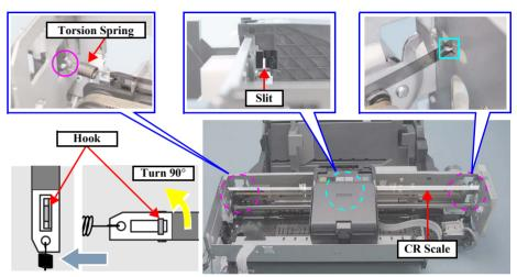
Figure 4-88. Removing the CR Scale
