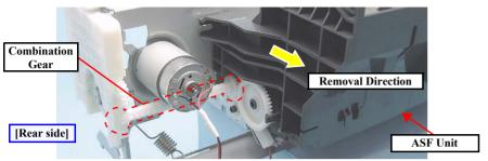
Figure 4-143. Removing the ASF Unit
