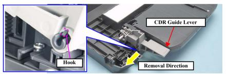
Figure 4-108. Removing the CDR Guide Lever
