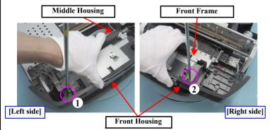
Figure 4-41. Reinstalling the Front Housing (2)
