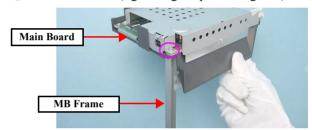
Figure 4-59. Removing the MB Frame
