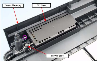
Figure 4-107. Removing the P/S Assy
