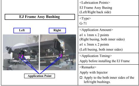
Figure 6-6. Lubrication of EJ Frame Assy
