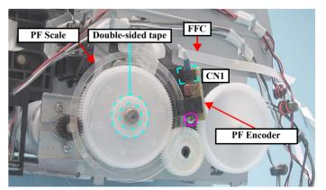
Figure 4-135. Removing the PF Encoder/PF Scale
