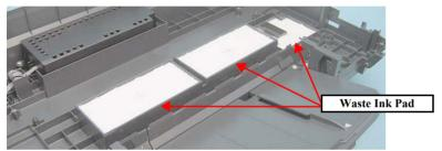
Figure 4-104. Removing the Waste Ink Pad
