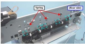
Figure 4-154. Removing the Upper Paper Guide (1)
