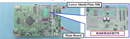
Figure 4-63. Removing the Main Board
