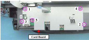
Figure 4-64. Removing the Card Board
