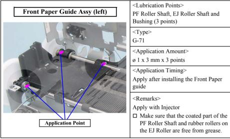
Figure 6-4. Lubrication of Front Paper Guide Assy (1)
