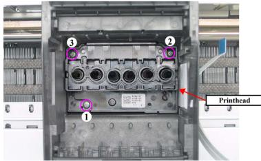
Figure 4-102. Removing the Printhead (1)
