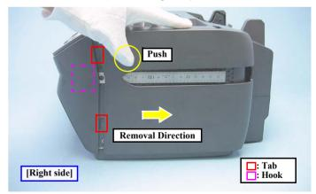
Figure 4-17. Removing the Right/Left Housings (2)
