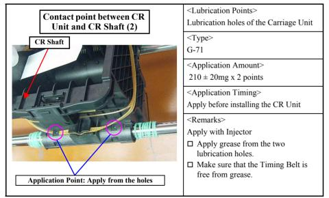
Figure 6-13. Lubrication of the CR Shaft (2)
