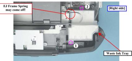
Figure 4-30. Removing the Waste Ink Tray (1)
