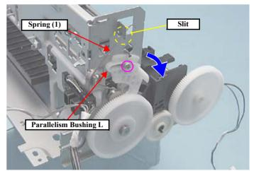
Figure 4-145. Removing the CR Unit (1)
