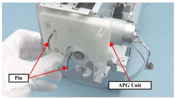
Figure 4-93. Reinstalling the APG Unit (3)
