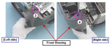
Figure 4-42. Reinstalling the Front Housing (3)
