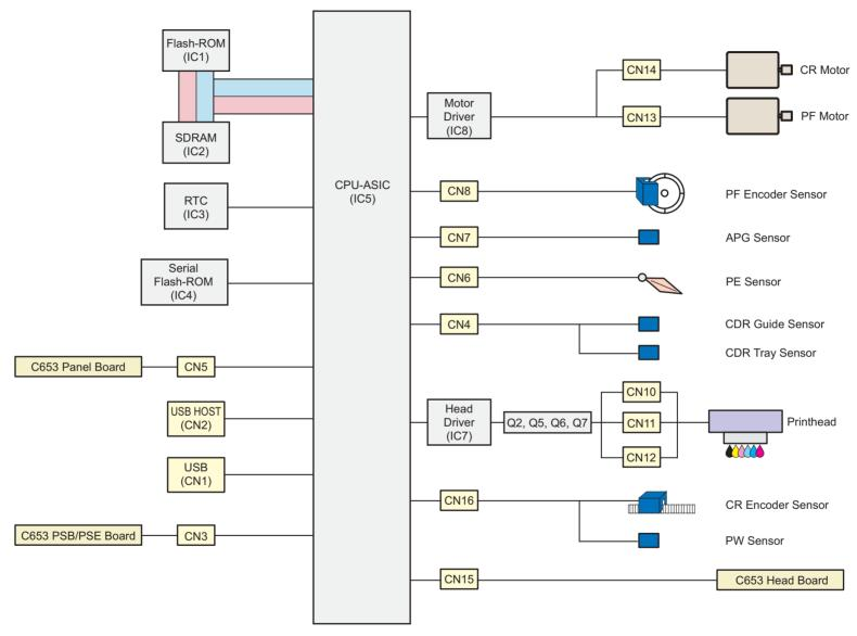
Figure 2-4. Circuit Block Diagram for R260/R265/R270
