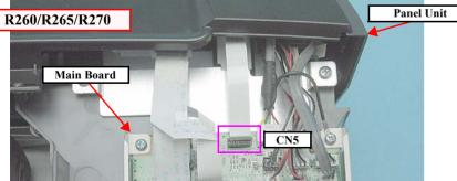
Figure 4-23. Removing the Connectors (Panel Unit)
