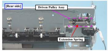
Figure 4-121. Removing the Extension Spring
