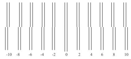
Figure 5-2. Head angular adjustment Pattern Printing (1)
