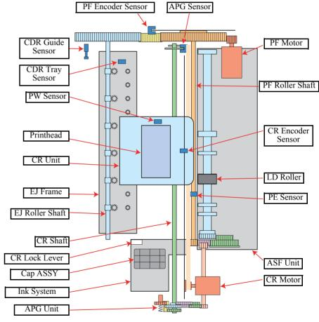
Figure 2-1. Printer Mechanism Diagram
