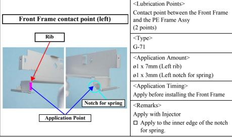
Figure 6-7. Lubrication of the Front Frame (1)
