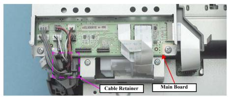
Figure 4-51. Removing the Cables (R360/R380/R390 Main Board)
