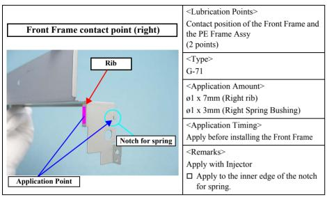
Figure 6-8. Lubrication of the Front Frame (2)
