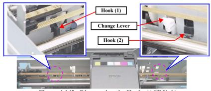
Figure 4-142. Disengaging the Hooks (ASF Unit)
