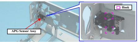
Figure 4-160. Removing the APG Sensor
