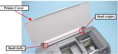
Figure 4-13. Removing the Printer Cover (1)
