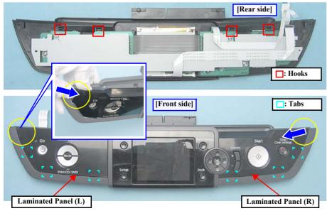
Figure 4-67. Removing the Left/Right Laminated Panels
