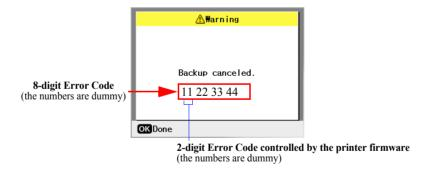
Figure 1-3. Backup Error Message and Error Code
