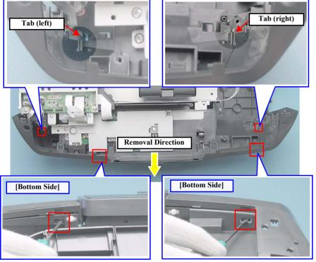
Figure 4-37. Removing the Front Housing (2)
