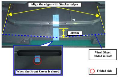
Figure 4-5. Protecting the Front Cover
