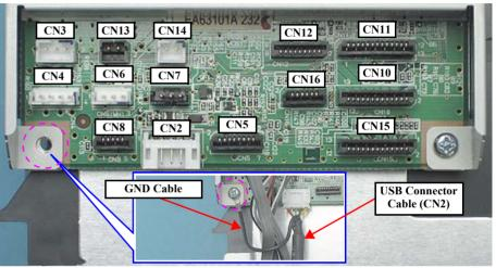
Figure 4-53. R260/R265/R270 Main Board Table 4-5. List of Connectors and their Destinations
