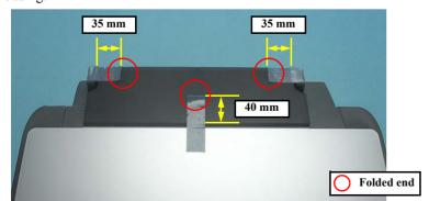
Figure 4-2. Securing the Paper Support
