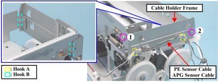
Figure 4-128. Removing the Cable Holder Frame
