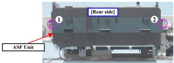
Figure 4-141. Removing the Screws (ASF Unit)
