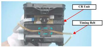
Figure 4-149. Removing the CR Unit (5)
