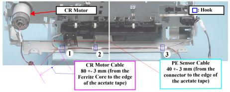
Figure 4-123. Removing the CR Motor (2)
