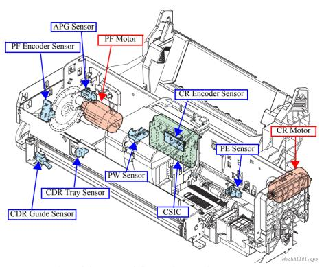
Figure 2-2. Motors & Sensors in the Printer Mechanism
