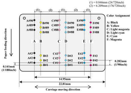
Figure 1-2. Nozzle Configuration
