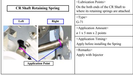
Figure 6-11. Lubrication for the CR Shaft Retaining Spring
