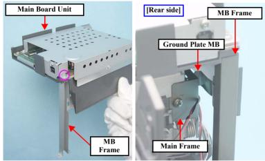
Figure 4-57. Reinstalling the Main Board Unit(1)
