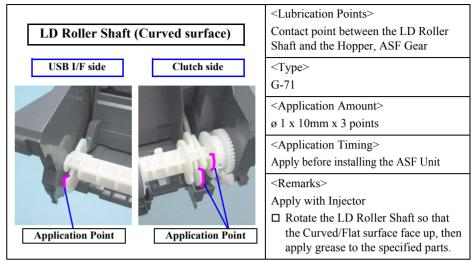
Figure 6-18. Lubrication of the LD Roller Shaft (1)
