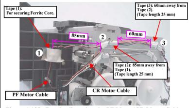
Figure 4-138. Routing/Securing the PF Motor/CR Motor Cables
