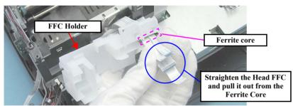
Figure 4-48. Removing the FFC Holder (2)
