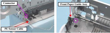
Figure 4-157. Removing the PE Sensor Cable
