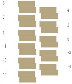
Figure 5-6. PF adjustment (Standard Area) Pattern Printing
