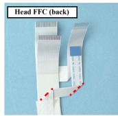
Figure 4-50. Routing the Head FFC (2)
