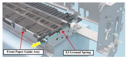
Figure 4-158. Removing the EJ Ground Spring
