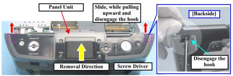
Figure 4-24. Removing the Panel Unit
