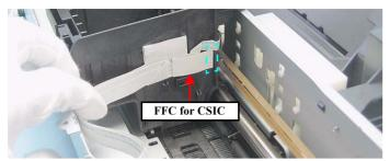
Figure 4-96. Removing the FFC for CSIC
