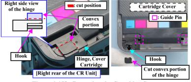
Figure 4-153. Removing the Cartridge Cover
