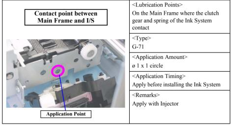
Figure 6-14. Lubrication of the I/S
