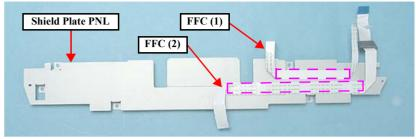
Figure 4-73. Removing the FFC
