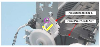
Figure 4-156. Removing the Parallelism Bushing L
