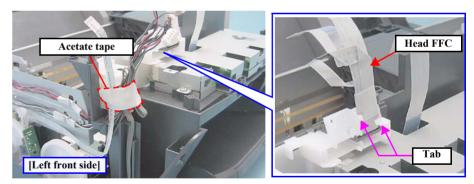
Figure 4-46. Removing the Cables
