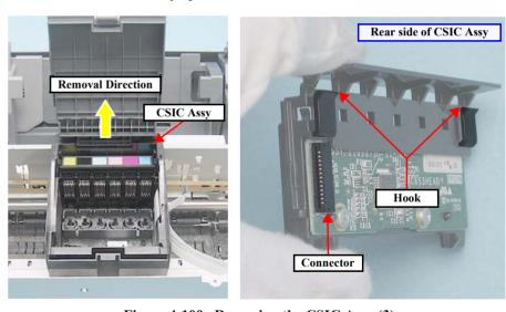
Figure 4-100. Removing the CSIC Assy (3)
