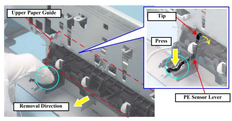
Figure 4-155. Removing the Upper Paper Guide (2)
