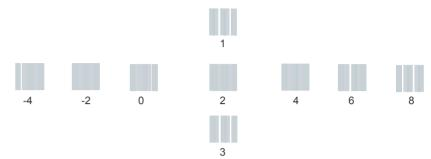
Figure 5-4. Bi-D adjustment Pattern Printing
