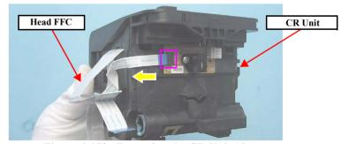
Figure 4-150. Removing the CR Unit (6)
