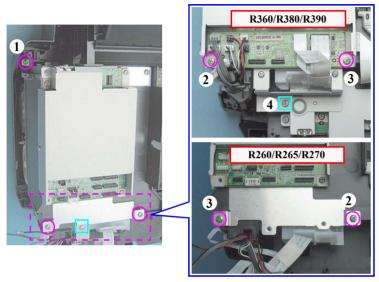
Figure 4-54. Removing the Main Board (1)
