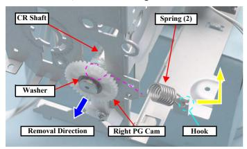
Figure 4-146. Removing the CR Unit (2)
