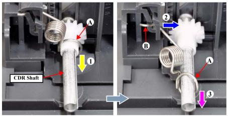
Figure 4-110. Removing the CDR Guide Lever Spring (2)
