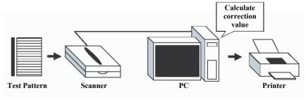
Figure 5-11. System Configuration
