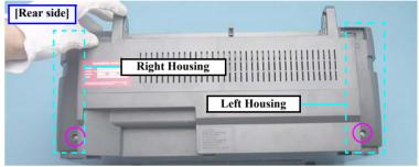
Figure 4-16. Removing the Right/Left Housings (1)
