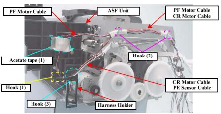
Figure 4-136. Removing the Harness Holder
