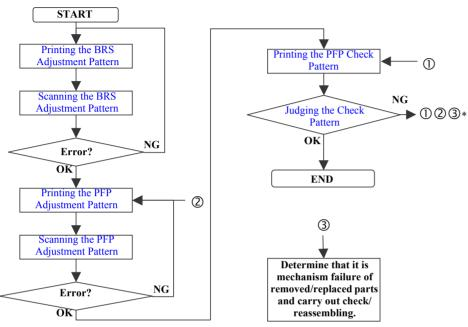
Figure 5-12. BRS/PFP Adjustment Flow
