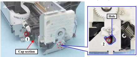
Figure 4-116. Removing the Ink System (1)
