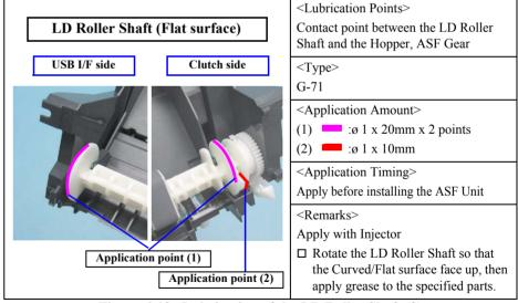
Figure 6-19. Lubrication of the LD Roller Shaft (2)
