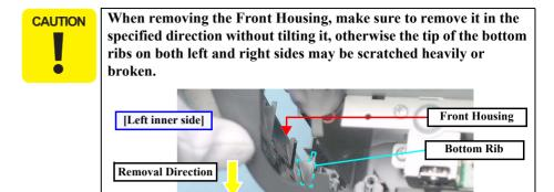
Figure 4-38. Caution as to Removing the Front Housing
