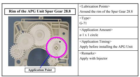
Figure 6-16. Lubrication of the APG Unit (2)
