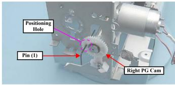
Figure 4-91. Reinstalling the APG Unit (1)
