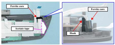
Figure 4-68. Removing the Panel Board (1)
