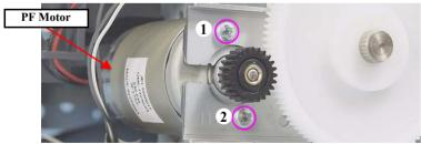
Figure 4-137. Removing the PF Motor
