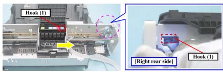
Figure 4-98. Removing the CSIC Assy (1)
