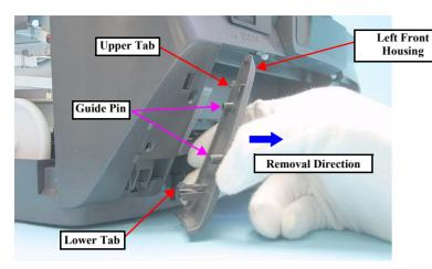
Figure 4-34. Tabs of the Right/Left Front Housings
