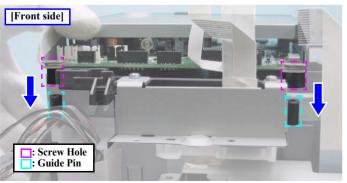
Figure 4-58. Reinstalling the Main Board Unit (2)
