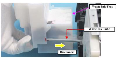
Figure 4-31. Removing the Waste Ink Tray (2)
