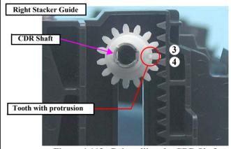
Figure 4-113. Reinstalling the CDR Shaft
