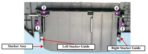
Figure 4-111. Removing the Stacker Assy
