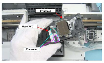
Figure 4-103. Removing the Printhead (2)
