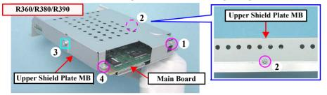
Figure 4-61. Removing the Upper Shield Plate MB (R360/R380/R390)
