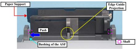
Figure 4-11. Removing the Paper Support
