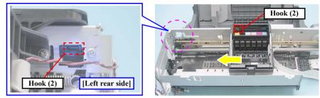
Figure 4-99. Removing the CSIC Assy (2)
