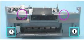
Figure 4-40. Reinstalling the Front Housing (1)
