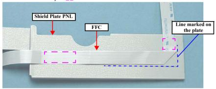
**Figure 4-77.** Removing the FFC (R260/R265/R270)
