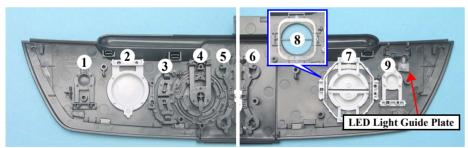
Figure 4-72. Removing the SW Buttons
