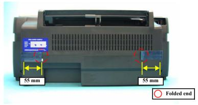
Figure 4-3. Securing the Middle Housing on its rear
