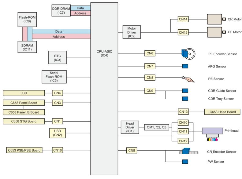
Figure 2-3. Circuit Block Diagram for R360/R380/R390
