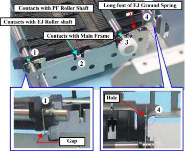
Figure 4-162. Attaching the EJ Ground Spring
