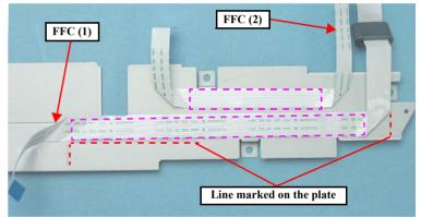
Figure 4-78. Attaching the FFC (1), FFC (2) (R360/R380/R390)
