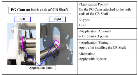
Figure 6-10. Lubrication of the CR Shaft PG Cam
