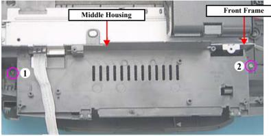
Figure 4-79. Removing the Middle Housing (1)
