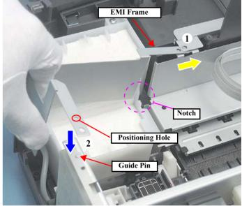
Figure 4-27. Reinstalling the EMI Frame
