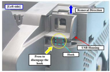
Figure 4-20. Removing the USB Housing
