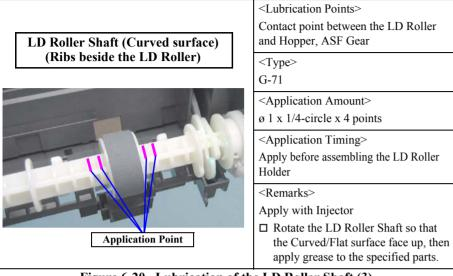
Figure 6-20. Lubrication of the LD Roller Shaft (3)
