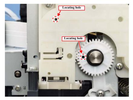
Figure 5-8. PG Position at PG Adjustment
