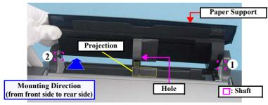
Figure 4-12. Reinstalling the Paper Support
