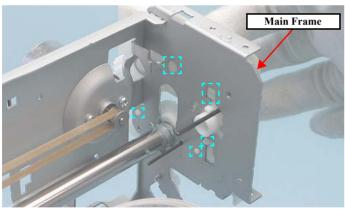
Figure 4-94. Reinstalling the APG Unit (4)
