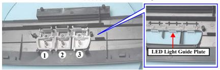
Figure 4-76. Removing the SW Buttons (R260/R265/R270)
