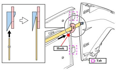
Figure 4-18. Disengaging the Hook and Tabs
