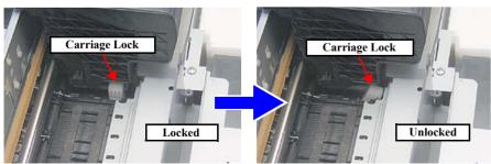
Figure 4-8. How to Unlock the Carriage
