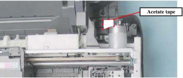
Figure 4-85. Removing the Ferrite Core (Printer mechanism)
