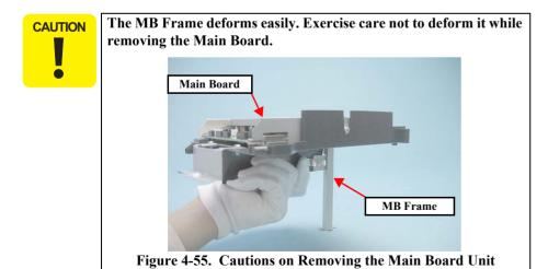
5. Remove the Main Board, taking extra care not to get the FFC caught on the opening of the CB Support Shield Plate. (R360/R380/R390 only)
