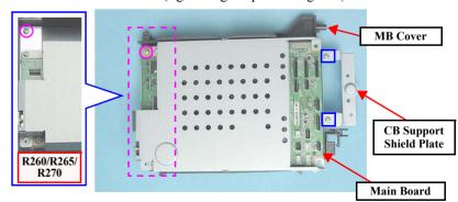
Figure 4-60. Removing the MB Cover/CB Shield Plate Support
