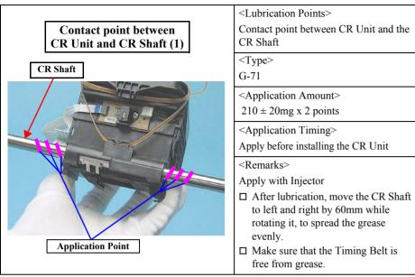
Figure 6-12. Lubrication of the CR Shaft (1)
