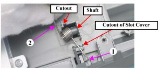
Figure 4-43. Reinstalling the Torsion Spring (R360/R380/R390 only)
