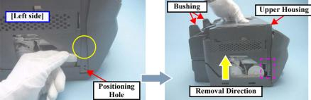
Figure 4-22. Removing the Upper Housing (2)
