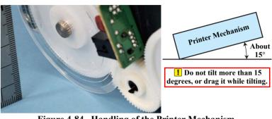
Figure 4-84. Handling of the Printer Mechanism
