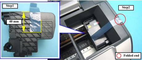
Figure 4-1. Securing the Carriage
