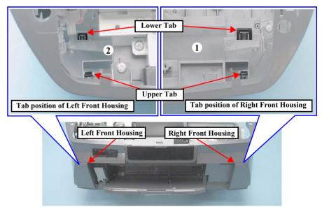
Figure 4-33. Removing Left/Right Front Housings (1)
