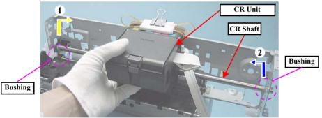
Figure 4-147. Removing the CR Unit (3)
