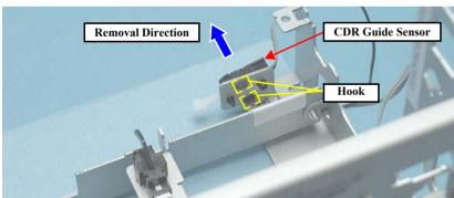
Figure 4-164. Removing the CDR Guide Sensor
