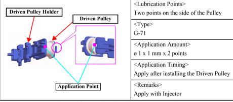
Figure 6-3. Lubrication of Driven Pulley (3)
