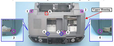
Figure 4-21. Removing the Upper Housing (1)
