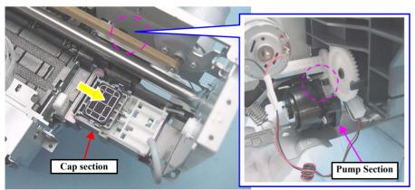
Figure 4-117. Removing the Ink System (2)
