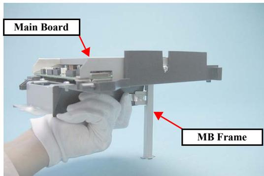
Figure 4-55. Cautions on Removing the Main Board Unit
