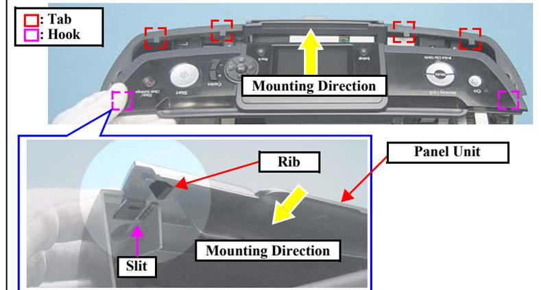
Figure 4-25. Reinstalling the Panel Unit
