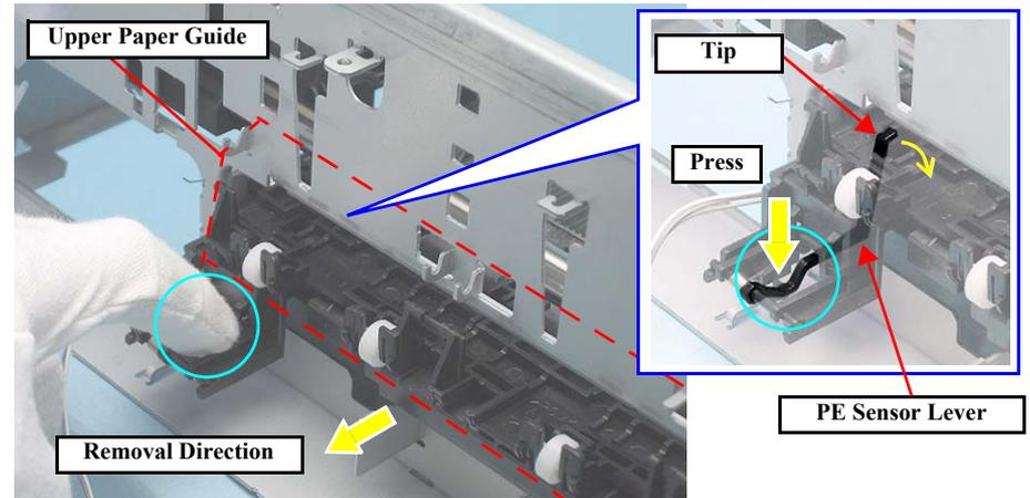
Figure 4-155. Removing the Upper Paper Guide (2)
