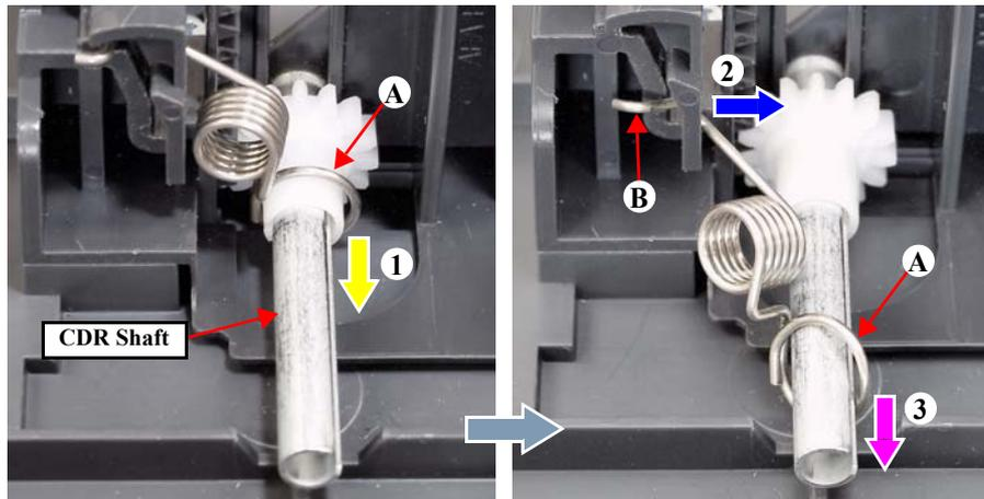
Figure 4-110. Removing the CDR Guide Lever Spring (2)
