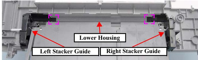
Figure 4-114. Reinstalling the Stacker Assy
