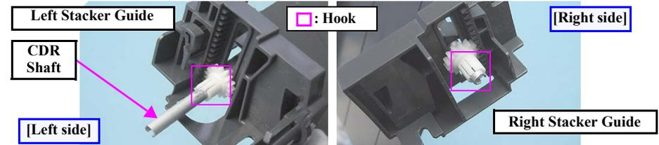
Figure 4-112. Removing the CDR Shaft
