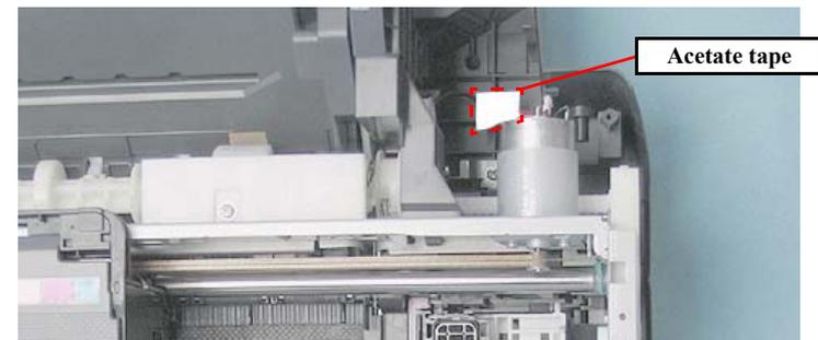
Figure 4-85. Removing the Ferrite Core (Printer mechanism)
