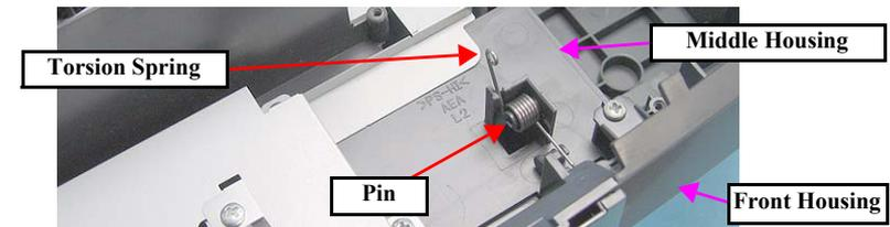
Figure 4-35. Removing the Torsion Spring (R360/R380/R390 only)
