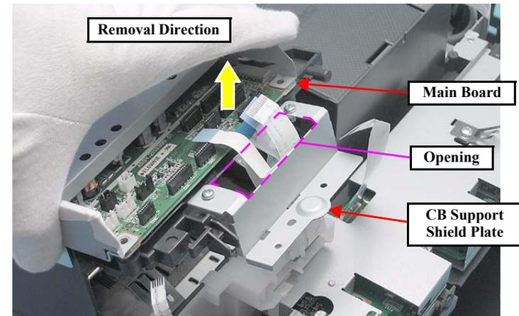
Figure 4-56. Removing the Main Board Unit (2)
