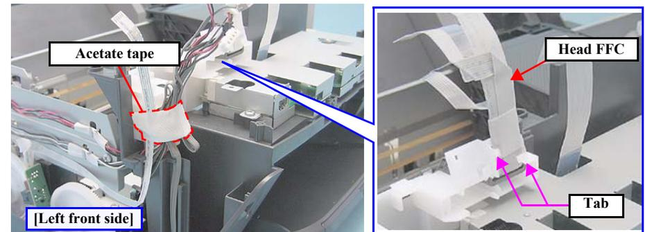
Figure 4-46. Removing the Cables
