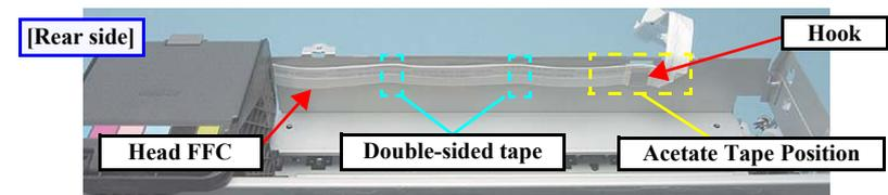
Figure 4-127. Removing the Head FFC
