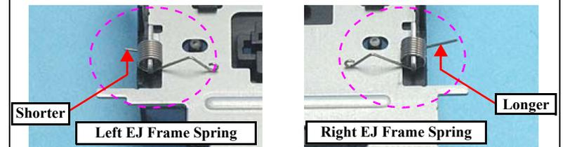
Figure 4-132. Reinstalling the Front Frame (1)
