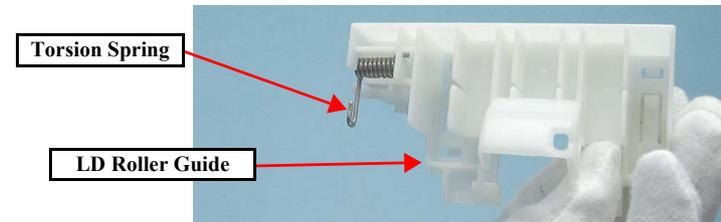
Figure 4-140. Removing the LD Roller Guide (2)
