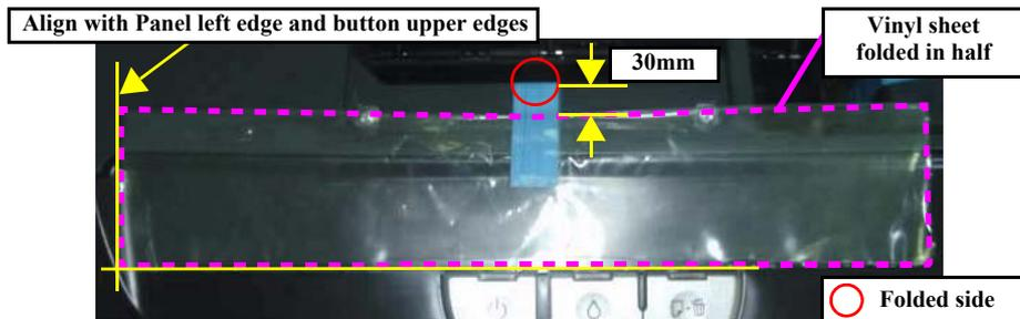
Figure 4-6. Protecting the Panel Unit (R260/R265/R270 only)
