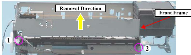
Figure 4-129. Removing the Front Frame
