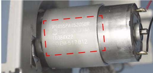
Figure 4-125. Reinstalling the CR Motor
