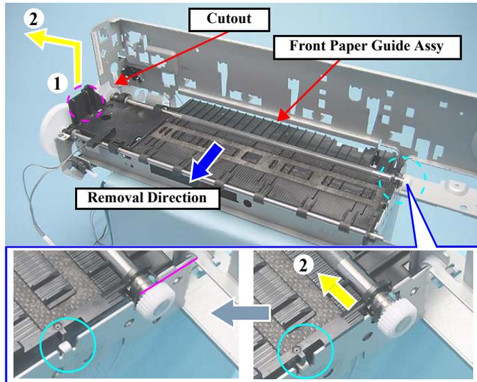
Figure 4-159. Removing the Front Paper Guide Assy
