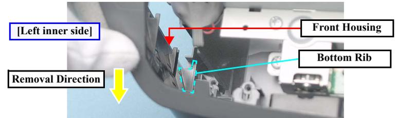
Figure 4-38. Caution as to Removing the Front Housing
