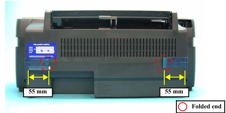
Figure 4-3. Securing the Middle Housing on its rear
