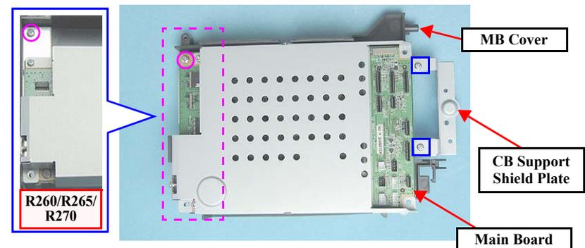
Figure 4-60. Removing the MB Cover/CB Shield Plate Support
