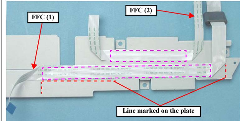
Figure 4-78. Attaching the FFC (1), FFC (2) (R360/R380/R390)
