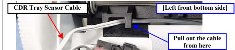
Figure 4-161. Routing the CDR Tray Sensor Cable
