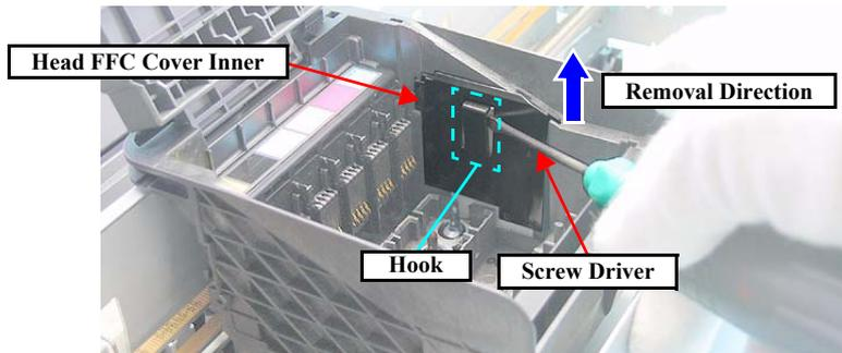
Figure 4-97. Removing the Head FFC Cover Inner
