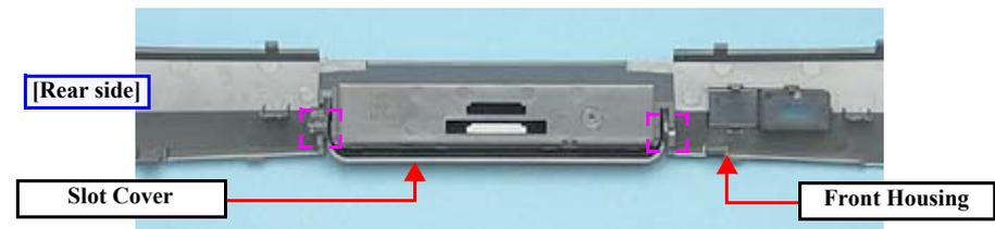
Figure 4-39. Removing the Slot Cover
