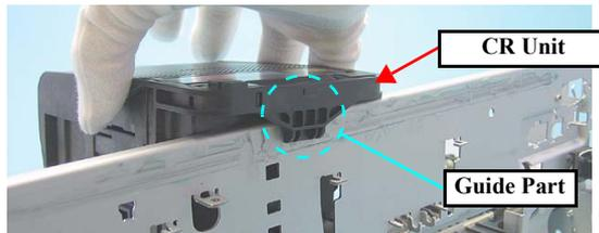
Figure 4-152. Reinstalling the CR Unit
