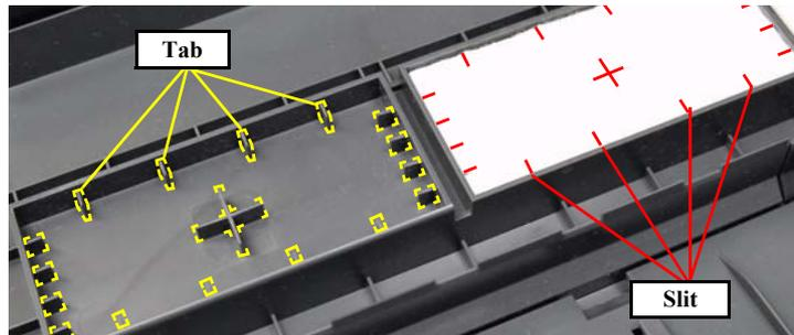
Figure 4-105. Reinstalling the Waste Ink Pads
