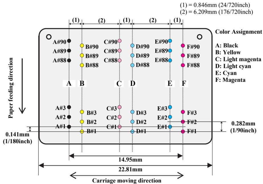
Figure 1-2. Nozzle Configuration
