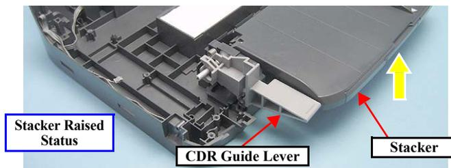
Figure 4-83. Cautions on Removing the Printer Mechanism
