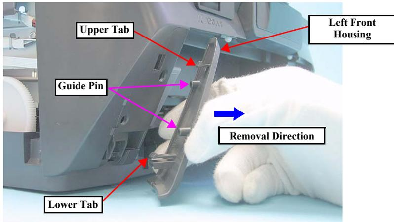
Figure 4-34. Tabs of the Right/Left Front Housings
