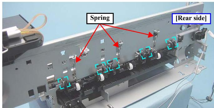
Figure 4-154. Removing the Upper Paper Guide (1)
