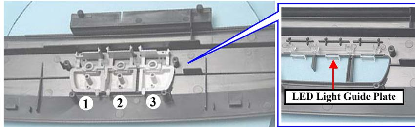
Figure 4-76. Removing the SW Buttons (R260/R265/R270)
