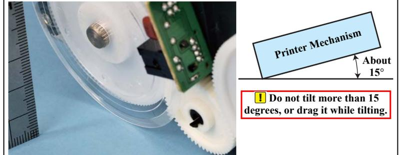
Figure 4-84. Handling of the Printer Mechanism
