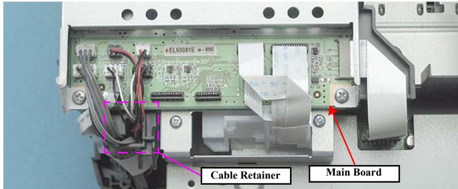
Figure 4-51. Removing the Cables (R360/R380/R390 Main Board)
