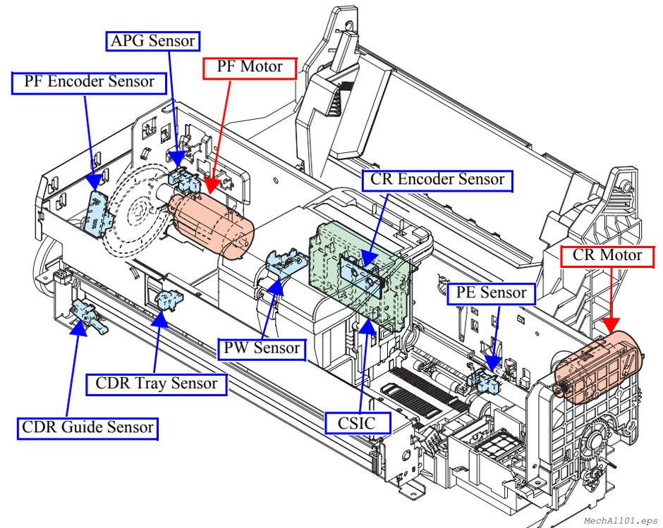
Figure 2-2. Motors & Sensors in the Printer Mechanism
