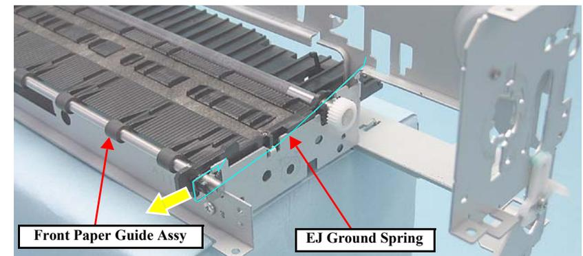
Figure 4-158. Removing the EJ Ground Spring
