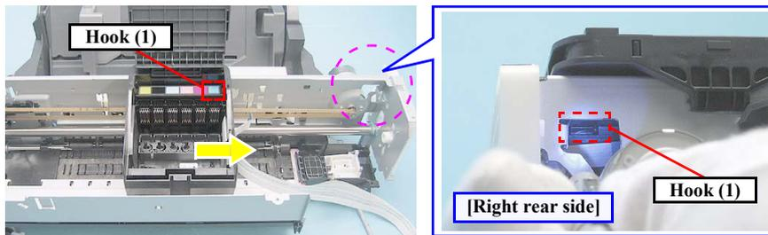
Figure 4-98. Removing the CSIC Assy (1)
