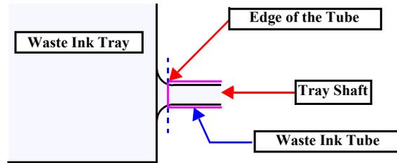
Figure 4-32. Cautions of installing the Waste Ink Tray
