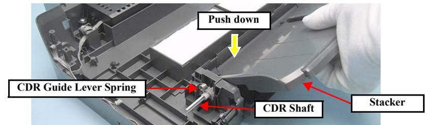
Figure 4-109. Removing the CDR Guide Lever Spring (1)
