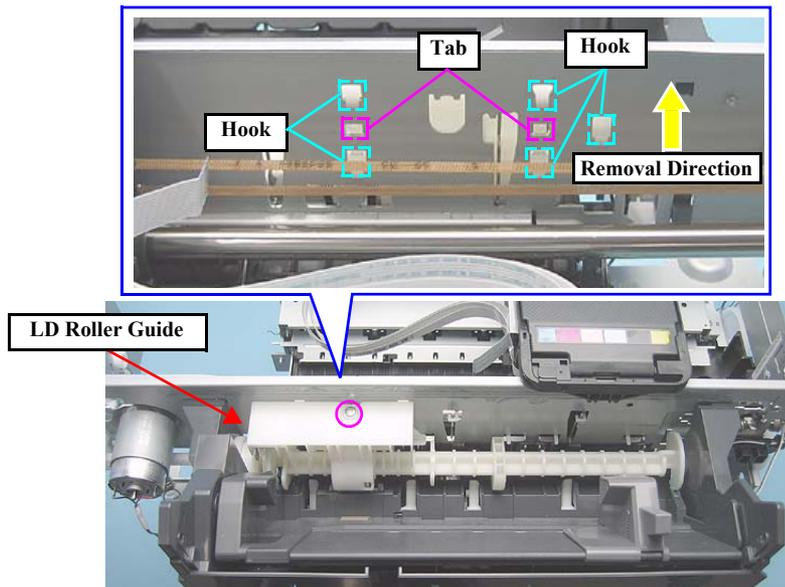
Figure 4-139. Removing the LD Roller Guide (1)
