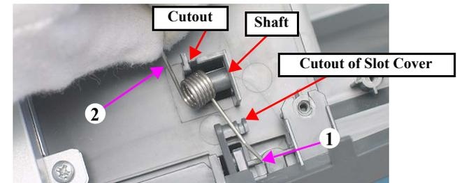
Figure 4-43. Reinstalling the Torsion Spring (R360/R380/R390 only)
