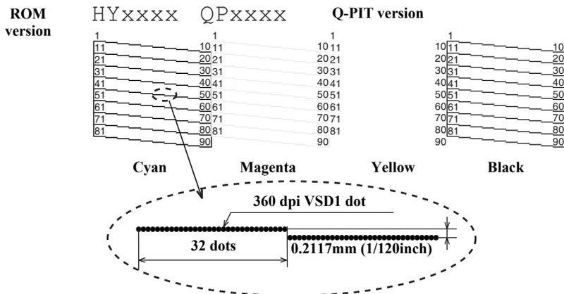
Note : The numbers shown in the figure are nozzle numbers. The numbers and the color names are not printed on an actual nozzle check pattern. The ROM version sample shown in the figure is one for the CX8300 series. “ELxxxx” is printed for CX7300 series. “ERxxxx” is printed for TX200 series. “HRxxxx” is printed for TX400 series.
