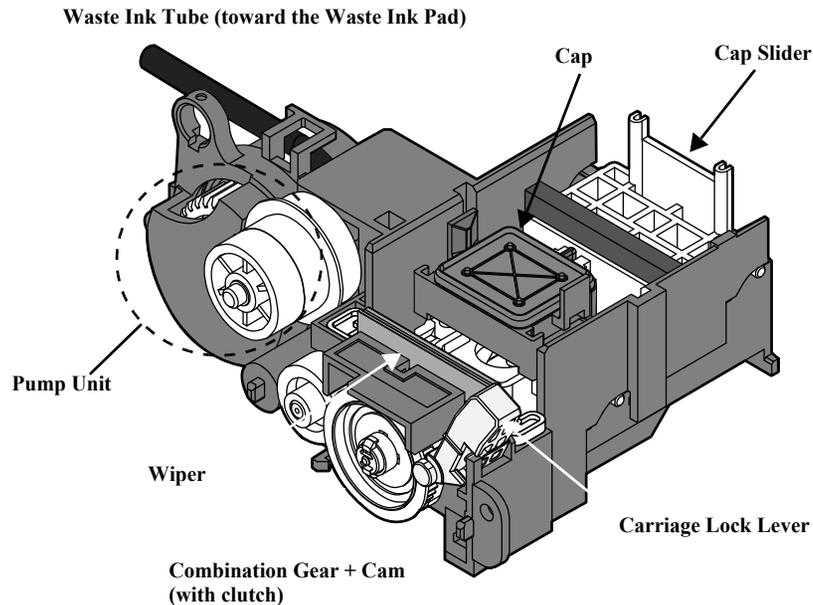
**Figure 2-14. Ink System Mechanism**
