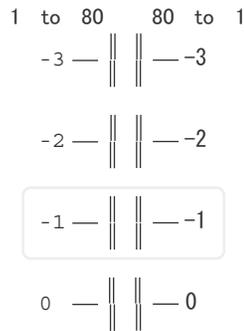
Figure 5-3. Head Angular Adjustment Printout Pattern (1)
