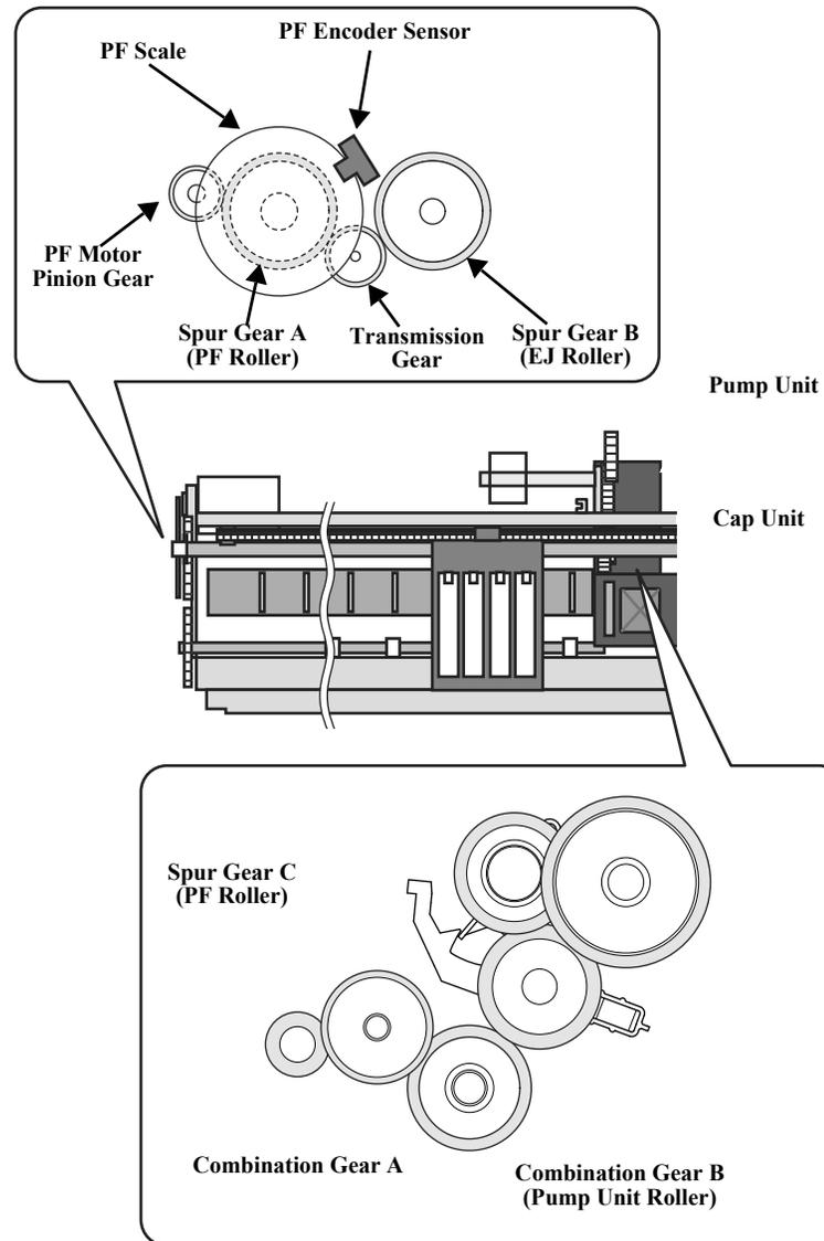
**Figure 2-19. PF Motor Drive Transmission to Pump Unit**
