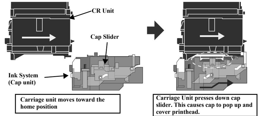
**Figure 2-15. Capping Mechanism**
