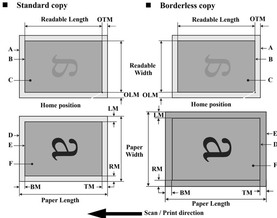
Figure 1-7. Relation Between Original and Copy (Borderless/With Borders)
