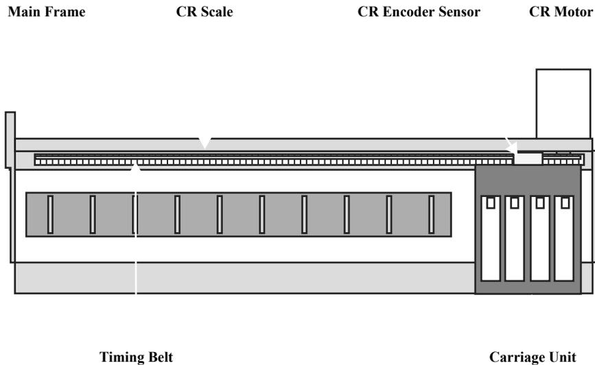
Figure 2-7. Carriage Mechanism
