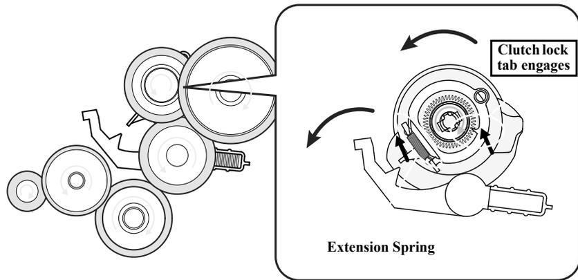
Figure 2-10. Releasing Clutch Lever
