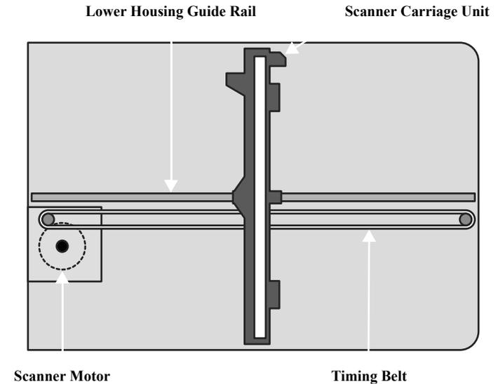
Figure 2-20. Scanner Mechanism
