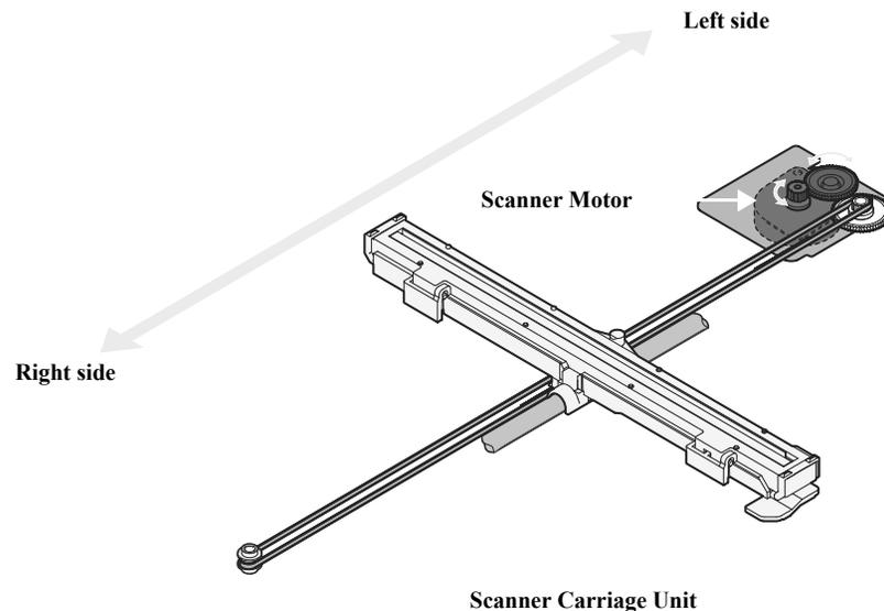
Figure 2-23. Scanner Carriage Unit Mechanism
