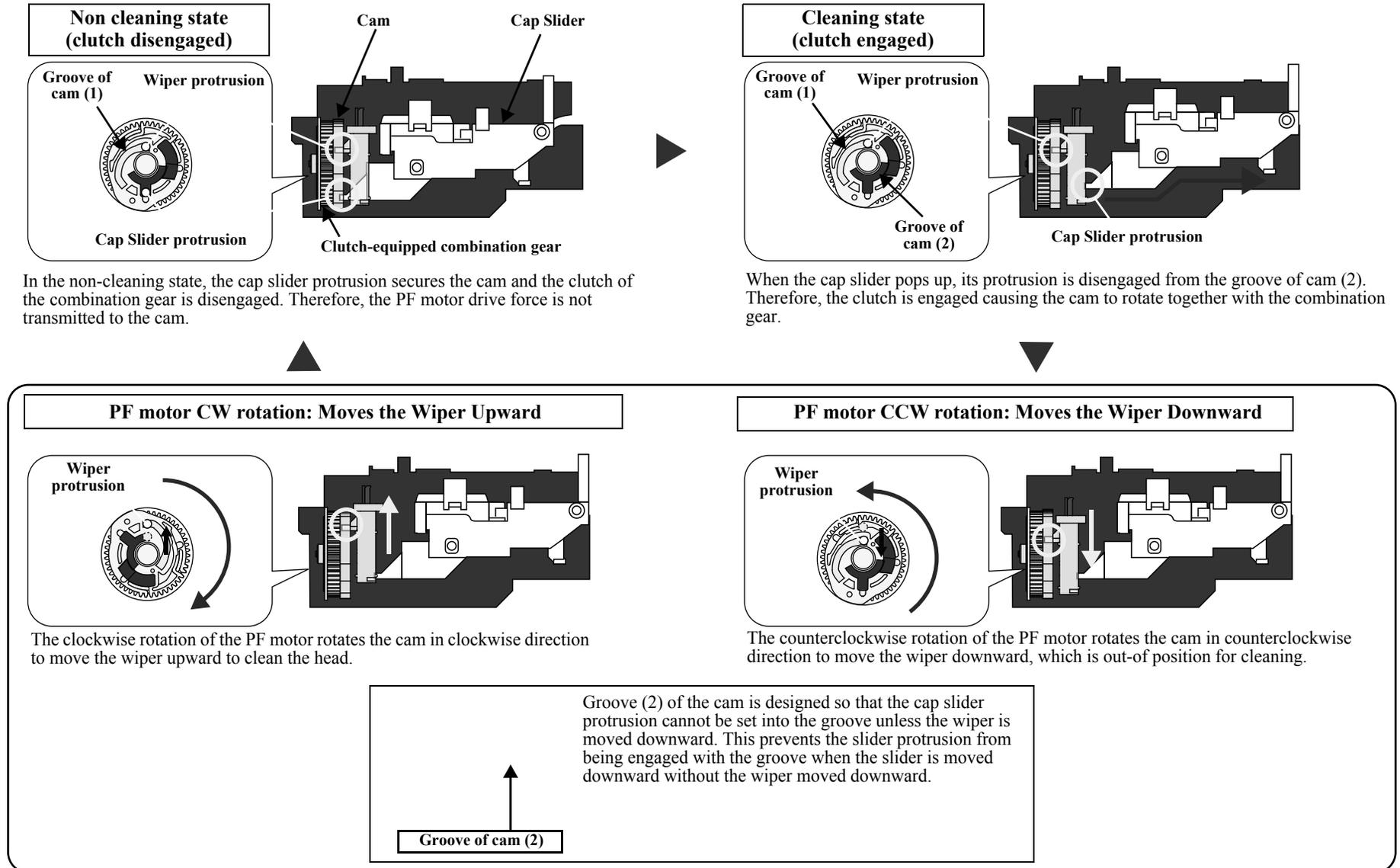
Figure 2-17. Wiping Mechanism
