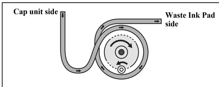
Note : The PF motor rotational direction is as seen from the right side of the printer.
