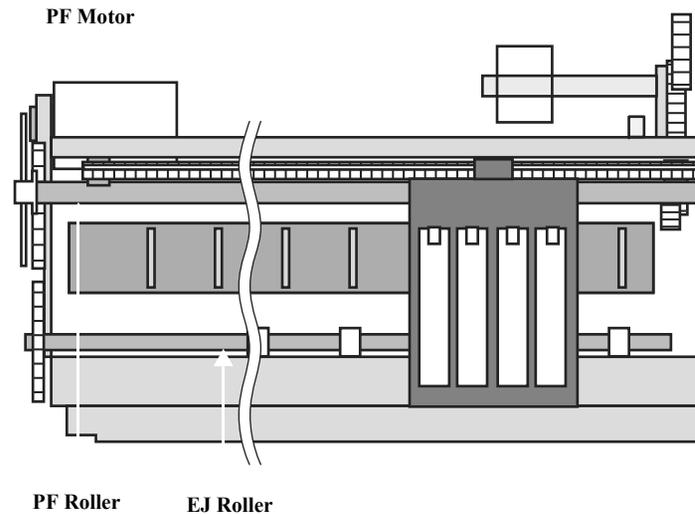
PF Motor Drive Transmission Path (as seen from the left side of the printer)
