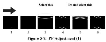
2. Examine the printed patches from the right to the left, and select a value for the patch with least white lines on its lower (bottom) area. If two or more patches are found as the best patch, be sure to select a value for the right most one. If it is difficult to judge, compare the most likely patch with the one on the left.
