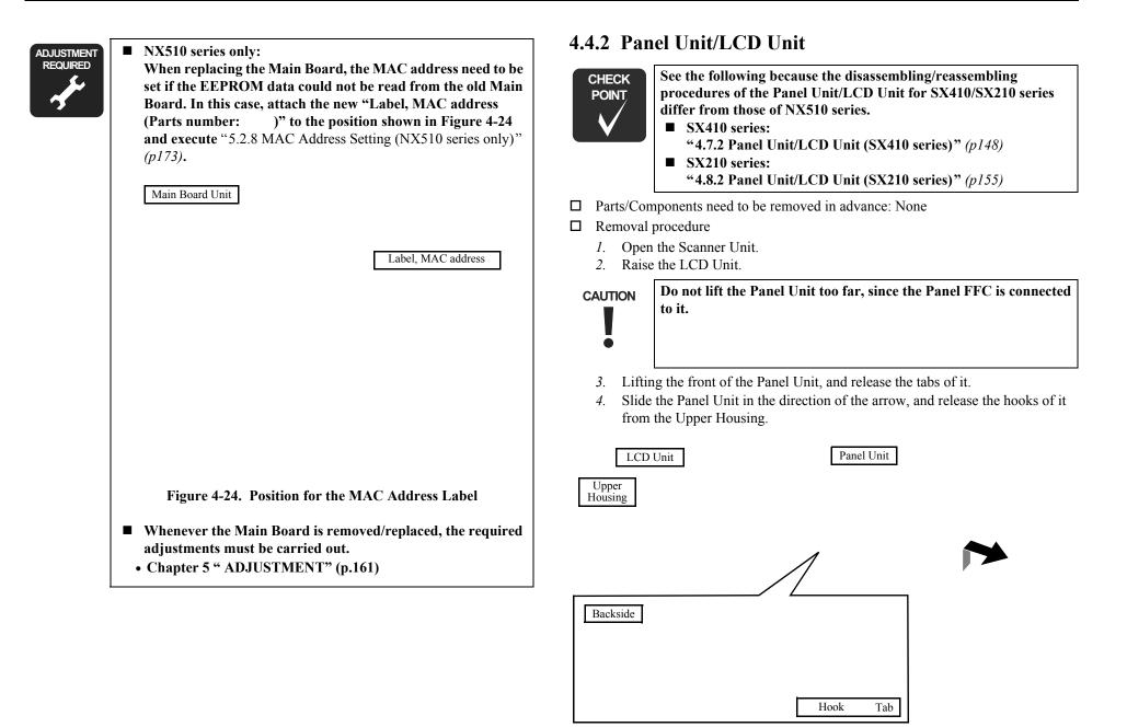
Figure 4-25. Removing the Panel Unit and LCD Unit (1)
