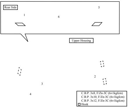
Figure 4-13. Removing the Upper Housing
