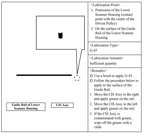
Figure 6-9. Lubrication on the Guide Rail of the Lower Scanner Housing
