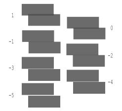
Figure 5-7. PF (standard print area) Adjustment Printout Pattern
