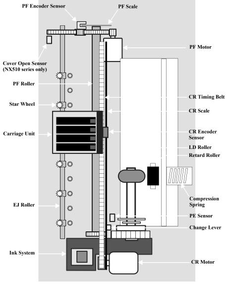
Figure 2-1. Printer Mechanism block diagram
