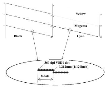
Figure 1-16. SX210 series *O* Nozzle Check Pattern\*
