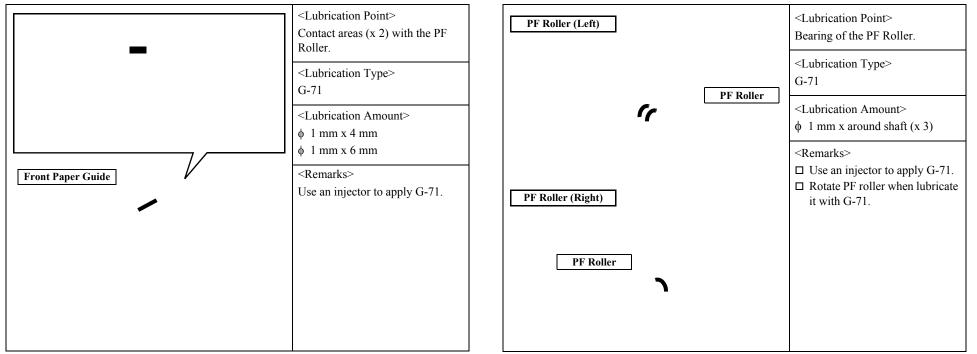
Figure 6-3. Lubrication on Front Paper Guide (2)
