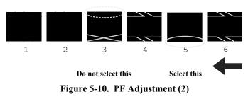
*3.* Input the selected value for each of the top and bottom in the program, and print a PF adjustment check pattern.
