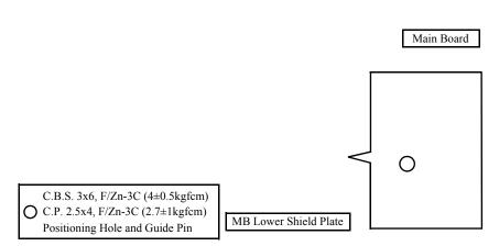
Figure 4-23. Removing the Main Board (2)
