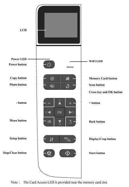
Figure 1-5. NX510 series Control Panel
