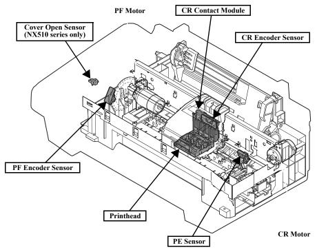
Figure 2-2. Motors & Sensors in Printer Mechanism
