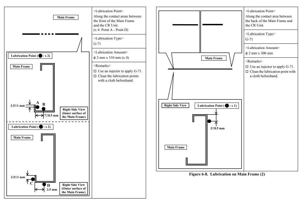
Figure 6-7. Lubrication on Main Frame (1)
