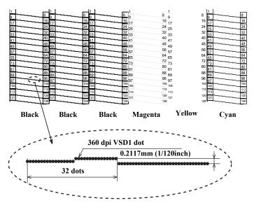
Figure 1-13. Nozzle Check Pattern for NX510 series\*
