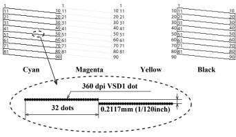
Figure 1-14. Nozzle Check Pattern for SX410 series\*
