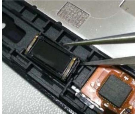
Step 7: remove PTT side key FPC, Volume side key FPC, Power key FPC and speaker from furnished PCBA by using soldering iron (Temperature: Lead-free technology 330°C±10°C, time: 3~5 seconds)
