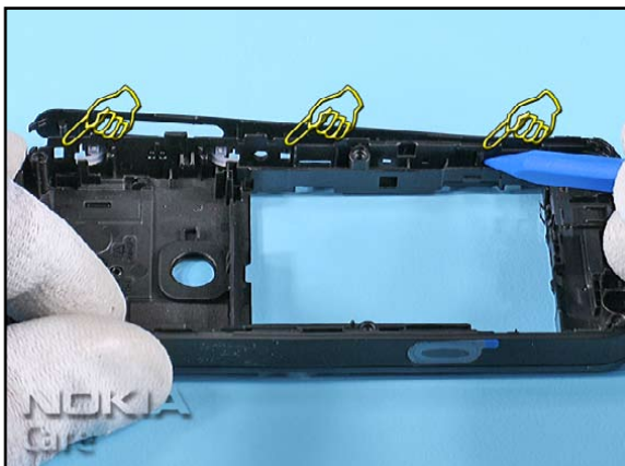
30. Release the clips of the DECO TRIM RIGHT...
