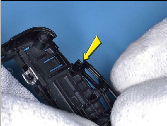
7. First slide the CONNECTOR COVER from top into the guiding from the B-COVER.
