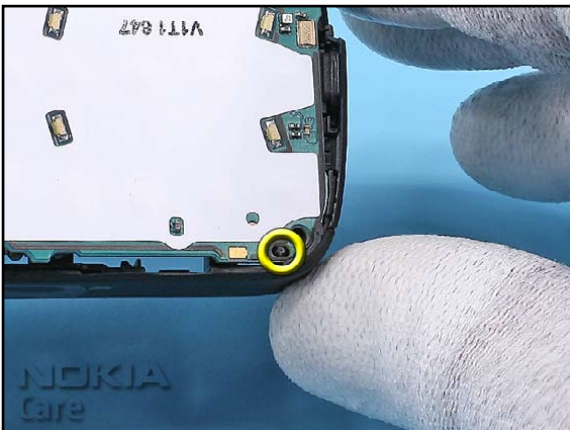
11. Take care to the guide pin of the B-COVER.
