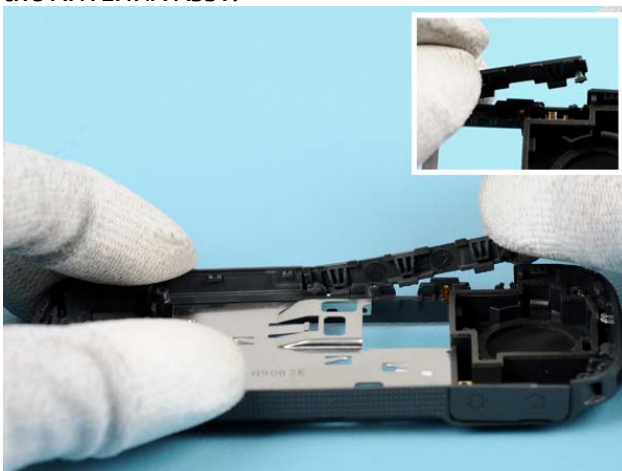
21) Remove the SIDE KEY by pulling it up and out.
