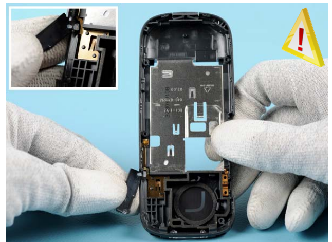
22) Carefully pull the EFII COVER to remove it.
