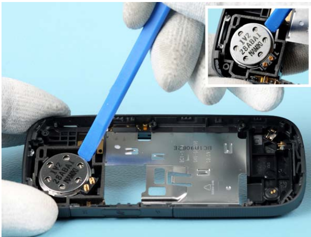
17) Use the SS-93 tool to lift the 3 in 1 MFD and release the 2 clips holding the 3 in 1 MFD.
