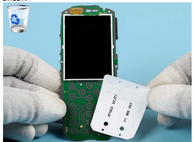
16) Remove the DOME SHEET. Do not use this part again.
