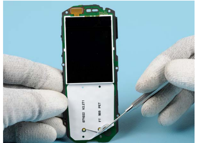
14) Use the dental tool to lift a corner of the DOME SHEET.
