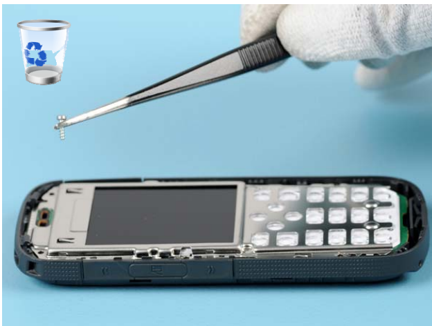
7) Remove the screws with the tweezers. Do not use the screws again.
