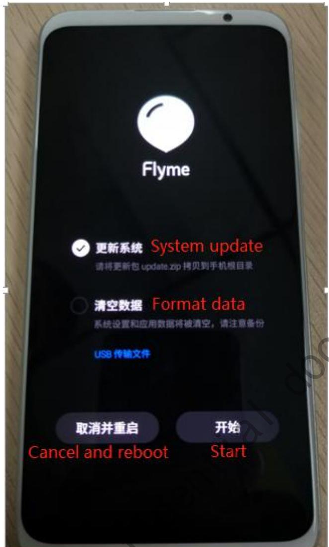
c. Press volume plus ,volume down and power button at the same time.the cellphone will access the USB download mode.**note:the cellphone will not show anything at this moment.** You need to press the power button about 10s.and then the cellphone will boot up.
