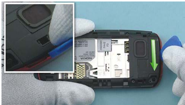
7) To detach the A-COVER, first release the bottom end of the A-COVER with the SRT-6.
