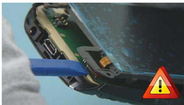
18) Disconnect the DISPLAY CONNECTOR with the SS-93. Be careful not to damage any components nearby.
