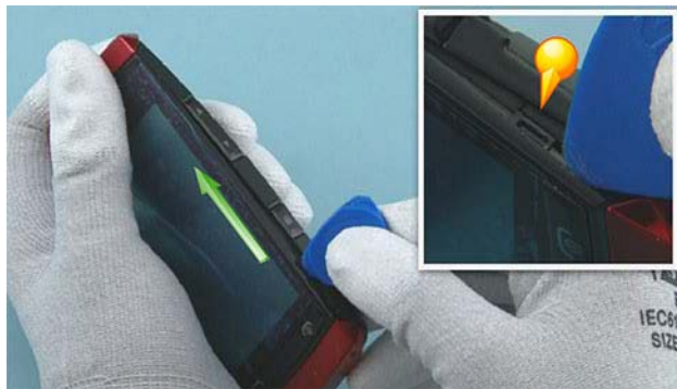
8) Continue to release the A-COVER with the SRT-6 on the VOLUME KEY side.
