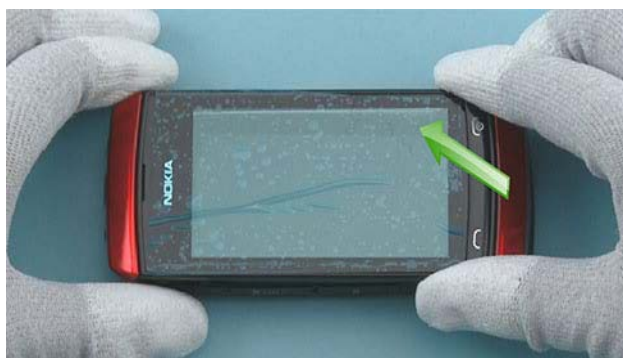
10) To remove the A-COVER, first lift up the bottom end of the A-COVER and then release the top end of the cover.
