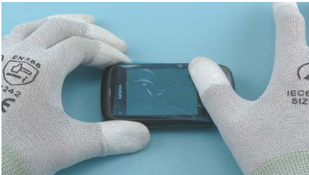
3) Protect the A-COVER TOUCH WINDOW with protective film.
