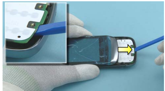
10) Use the SS-93 to release the D-COVER from the shown place.
