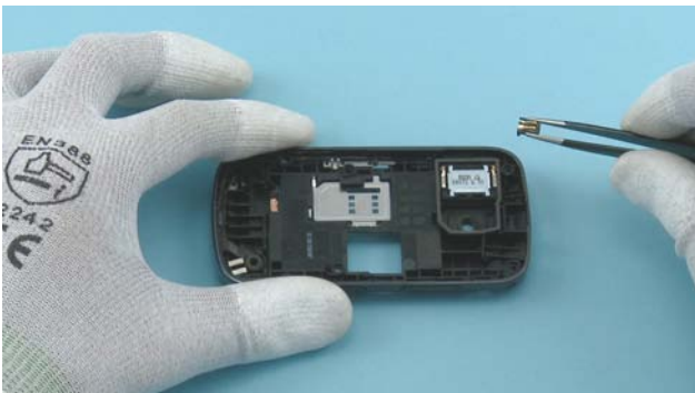
15) Remove the DC JACK with the tweezers.
