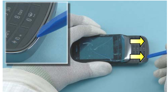
8) Use the SS-93 to release the KEYMAT.
