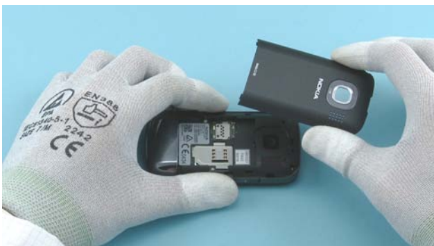
5) Remove the BATTERY COVER.
