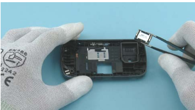
17) Remove the IHF SPEAKER with the tweezers.
