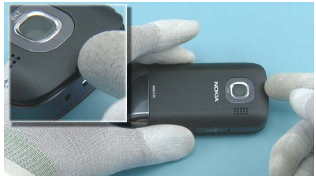
4) Open the BATTERY COVER by using the release notch.
