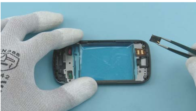
29) Remove the EARPIECE with the tweezers.
