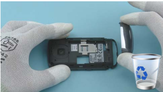
21) Remove the B-COVER DECO. Do not use it again. Discard it.
