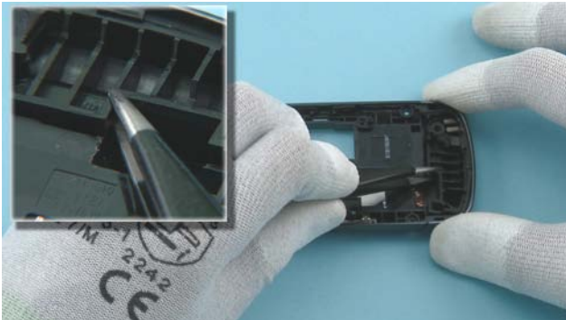
19) Insert the tweezers underneath the ANTENNA MODULE to lift it up and remove it.
