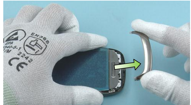
8) Remove the A-COVER CHIN by pulling it into direction shown.
