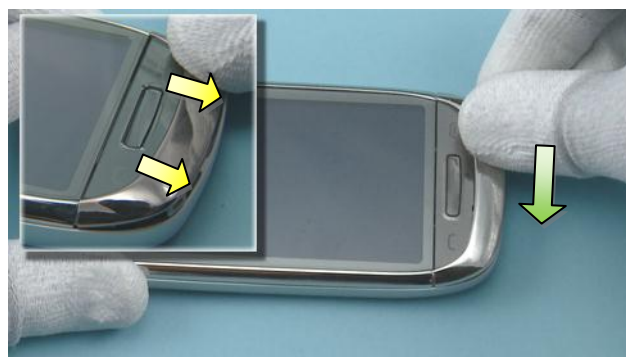
57) Press the A-COVER CHIN from the top to lock the two clips on the bottom end.
