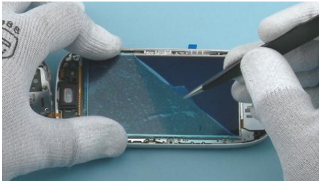
48) Remove the protective film from the DISPLAY with the tweezers.
