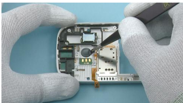
10) Remove the camera lens protective film with the tweezers.
