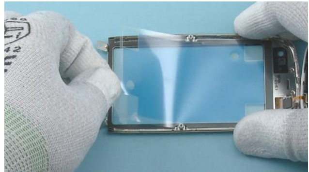
49) Remove the protective film from the A-COVER.
