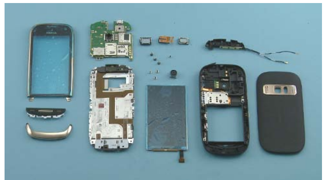
52) Nokia Oro disassembly is now complete.
