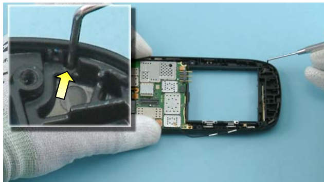
37) Insert the dental tool to the shown place and lever out the MAIN ANTENNA.
