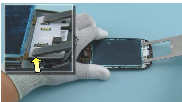
15) Then use the display removal tool SS-250 to release the DISPLAY very carefully. Note the alignment of the display removal tool SS-250.
