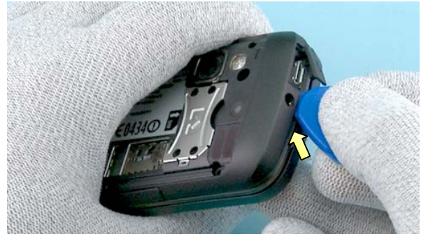
8) Use the SRT-6 to release the clip on the top side of the phone holding the B-COVER.
