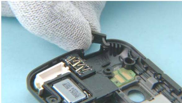
33) Lift up and remove the USB DOOR.
