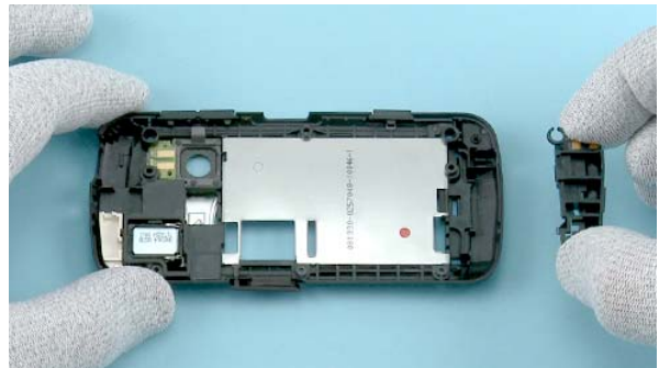
36) Remove the ANTENNA ASSEMBLY.
