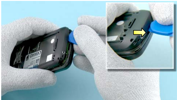
9) Release also the second clip on the bottom end of the phone with the SRT-6.
