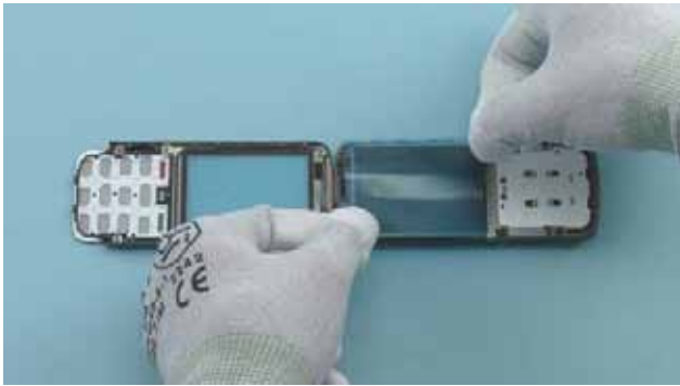
13) Protect the DISPLAY with protective film.
