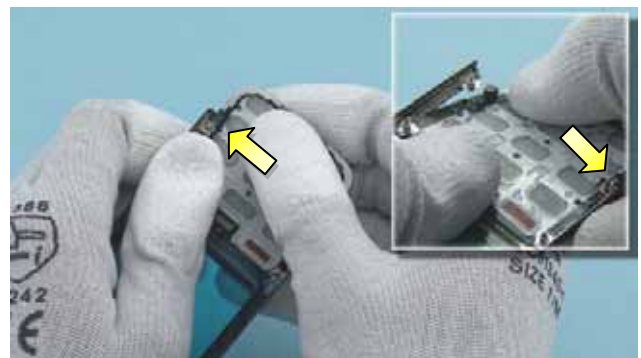
18) Push the corner of the KEYMAT as shown to detach the clip holding it. Release also the clip on the other corner. Pull out the KEYMAT and remove it.
