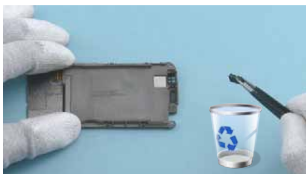
29) Remove the EARPIECE with the tweezers. Discard it.
