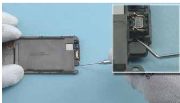
28) Use the dental tool to detach the EARPIECE.
