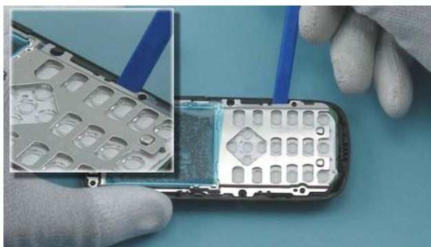
15) Use the SS-93 to release the shown side of the ENGINE BOARD.
