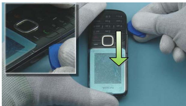
8) Release the other side of the A-COVER from the D-COVER by sliding the SRT-6 to direction shown.
