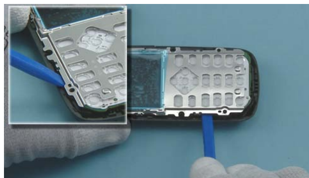
16) Release also the other side with the SS-93.
