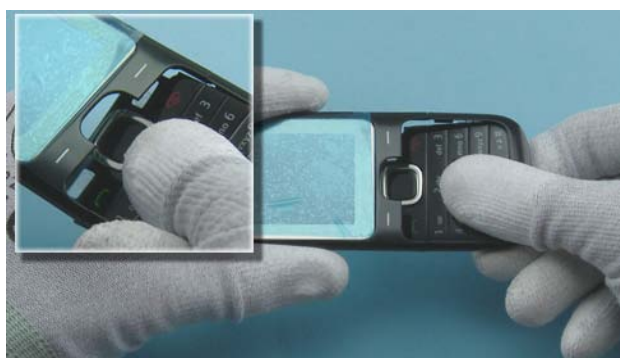
12) Push down to release the KEY MAT.
