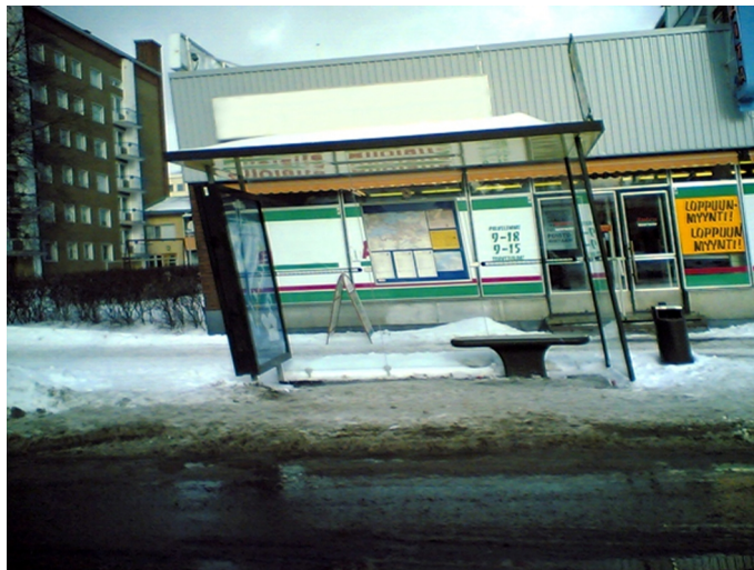
Figure 25 Near objects get skewed when taking images from a moving vehicle
