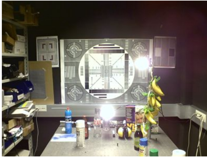
Figure 35 Image of point light sources taken with a clean protective window
