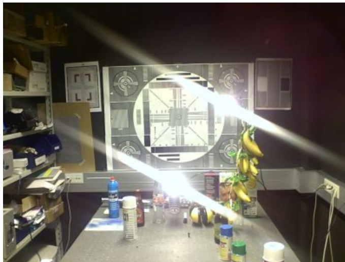
Figure 36 Image of point light sources taken with a dirty (fingerprint) protective window
