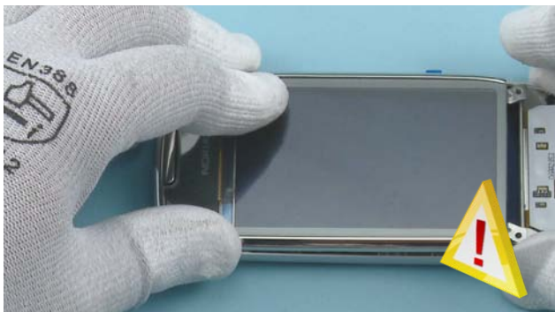
52) Turn over the A-COVER. Be careful not to damage the flex!
