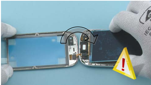
48) Turn over the DISPLAY. Be careful not to damage the flex!
