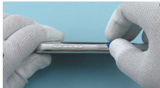
63) Finally, remove the LOCK KEY protective film.
