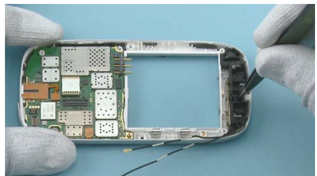
21) Place the MAIN ANTENNA with the tweezers.
