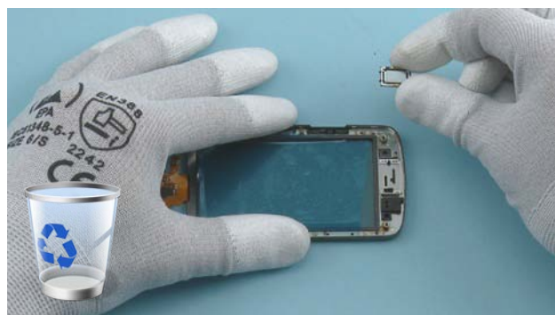
34) Remove the EARPIECE. Do not use it again. Discard it. Remove also the EARPIECE adhesive remains.
