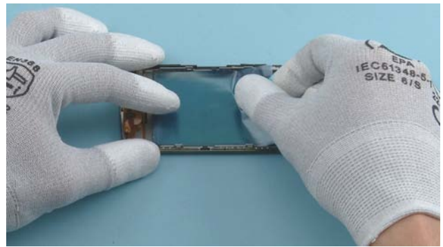
22) Protect the other side of the A-COVER with protective film.
