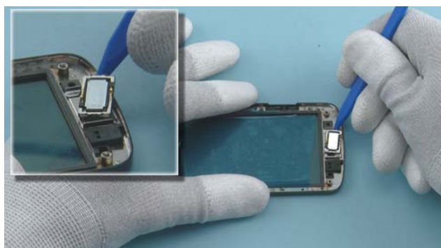
33) Use the sharp end of the SS-93 to release the EARPIECE.
