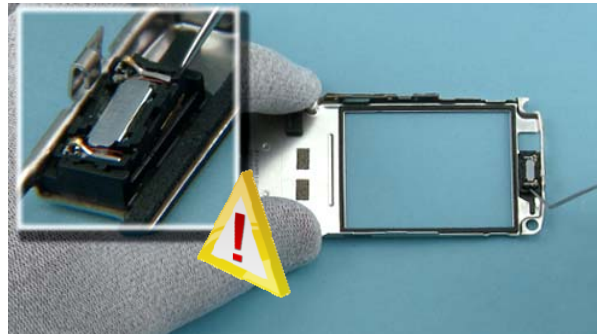
28) Use the dental tool to lift up the EARPIECE. Be aware of the sharp point of the dental tool – be careful not to injure yourself!
