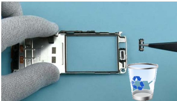
29) Remove the EARPIECE using tweezers. Do not use it again.
