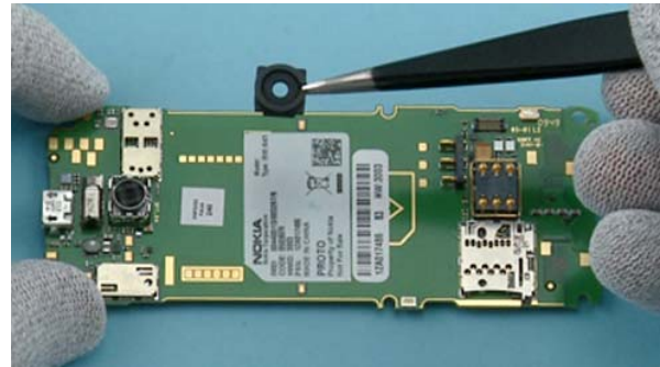
22) Use the tweezers to remove the CAMERA BOOT.
