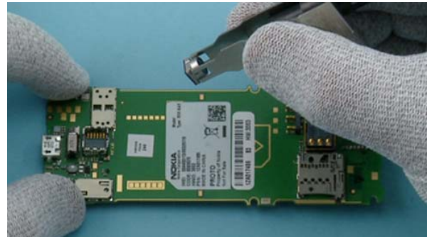
24) Lift up the SS-88 and remove the CAMERA.
