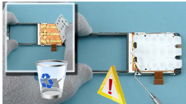
30) Use the dental tool to lift up one corner of the DOMESHEET ASSY. Peel off and remove the DOMESHEET ASSY. Do not use it again.
