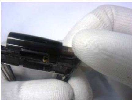
37. Remove the hinge.
