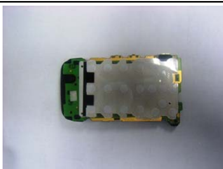
19. Antenna assembly completed.
