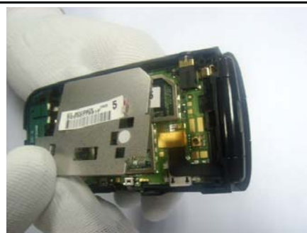
22. Assemble shielding case on MB.
