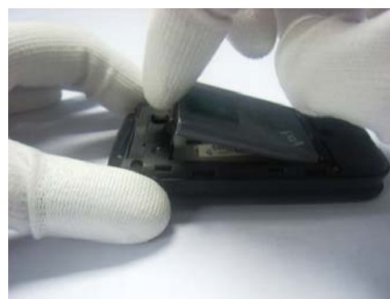
4. Lift and remove battery.
