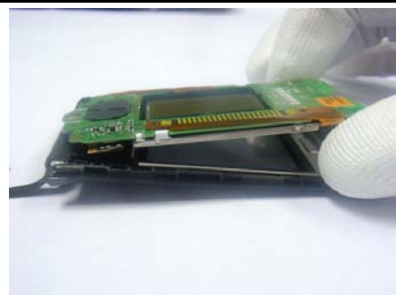
12. Assemble SB and A-Cover.
