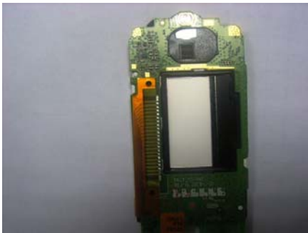
9. Assemble main LCM and SB.
