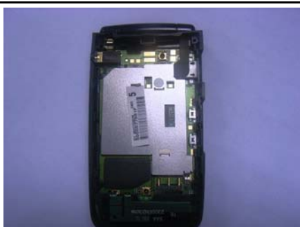
23. MB assembly completed.
