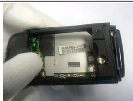
28. Assemble C-Cover and D-Cover.
