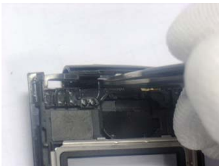
35. Remove Flash LED Lens.
