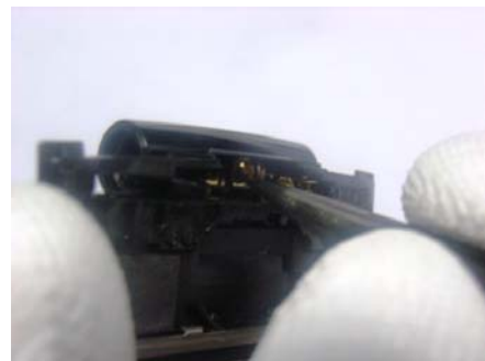
36. Push out the hinge.
