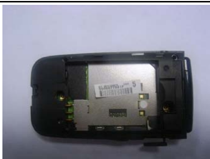
29. Reserve USB rubber hold for USB rubber inserts.
