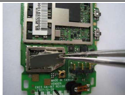
16. Open the shielding case.
