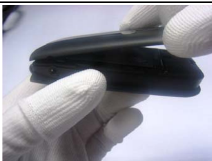
3. Push release and lift to remove battery cover.
