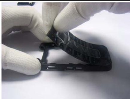
25. Pull and remove key pad.
