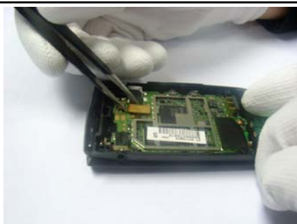
13. Open the FPC BTB connector.
