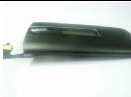
14. A-Cover and B-Cover assembly completed.
