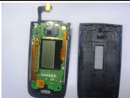
29. Disassemble A-Cover and B-Cover.
