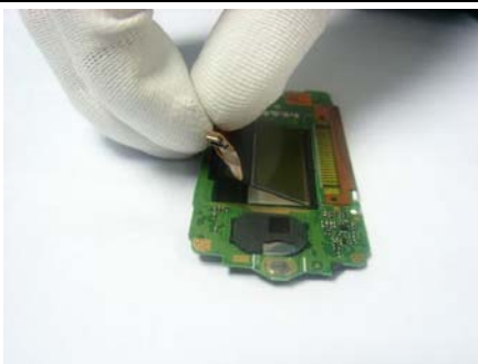
39. Take and remove sub LCM - 2.
