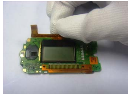
10. Assemble sub LCM.
