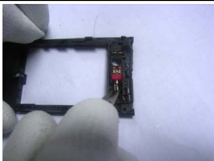
9. Remove the vibrator.
