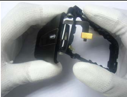
15. Insert FPC through C-Cover.
