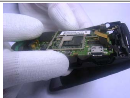
20. Assemble MB in C-Cover.
