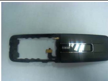
17. Assemble B-Cover and C-Cover completed.
