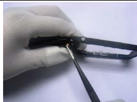
16. Push the hinge cam to housing
