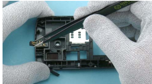
24) Remove the DC JACK with the tweezers.
