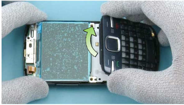
13) Lift up the KEYMAT ASSY from the top side as shown.
