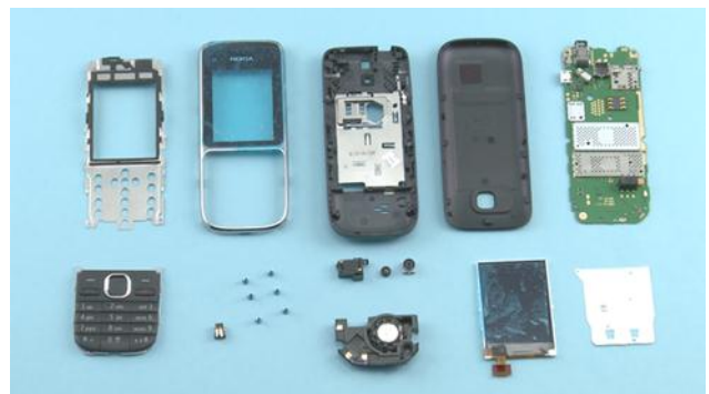
36) The Nokia C2-01 disassembly is now complete.
