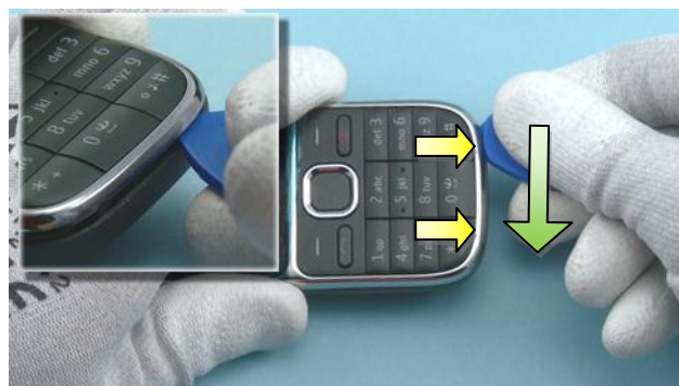
8) Slide the SRT-6 to the direction shown to release the clips on the bottom side of the device.
