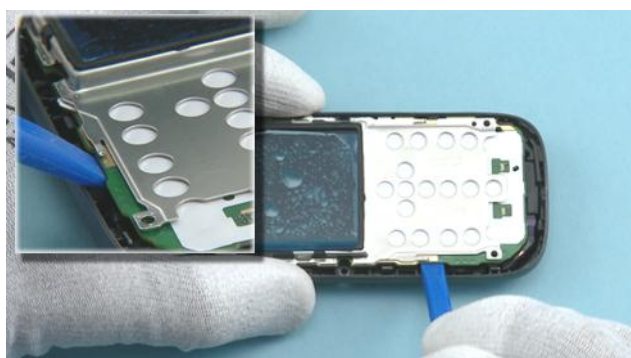
17) Use the SS-93 to release the other side of the ENGINE BOARD.
