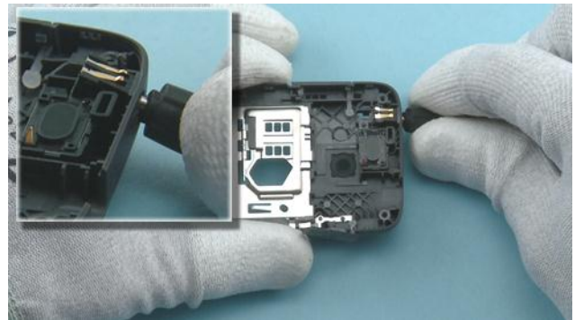
32) Use the DC PLUG to lever out the DC JACK.
