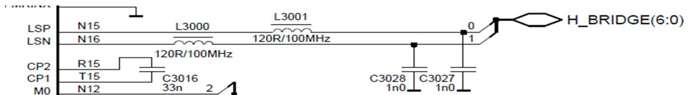
Figure 59 Speaker outputs with ferrite filters
