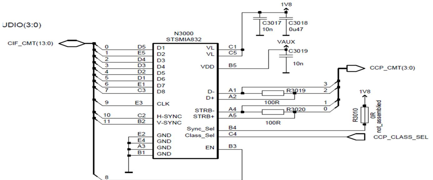
Figure 68 Camera de-serializer for serial camera module
