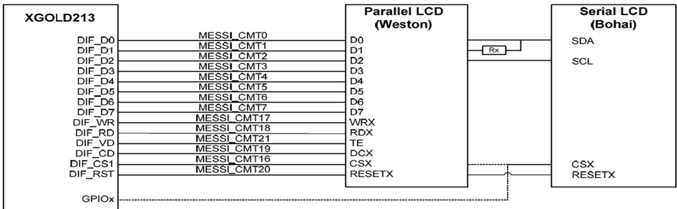
**Figure 62 Display interface (parallel and serial coexist)**
