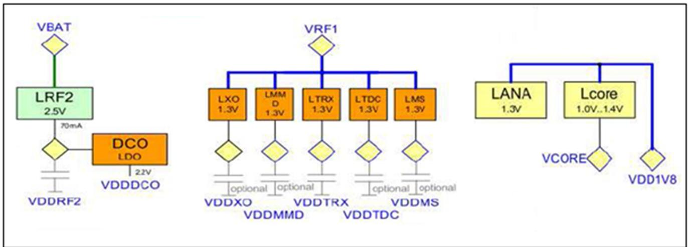
**Figure 72 Power concepts for X-GOLD213 RF sub-system**
