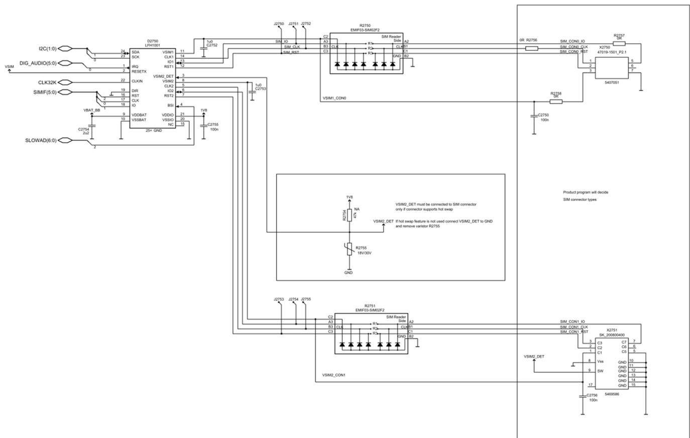
**Figure 65 Dual SIM using LFH1001**
