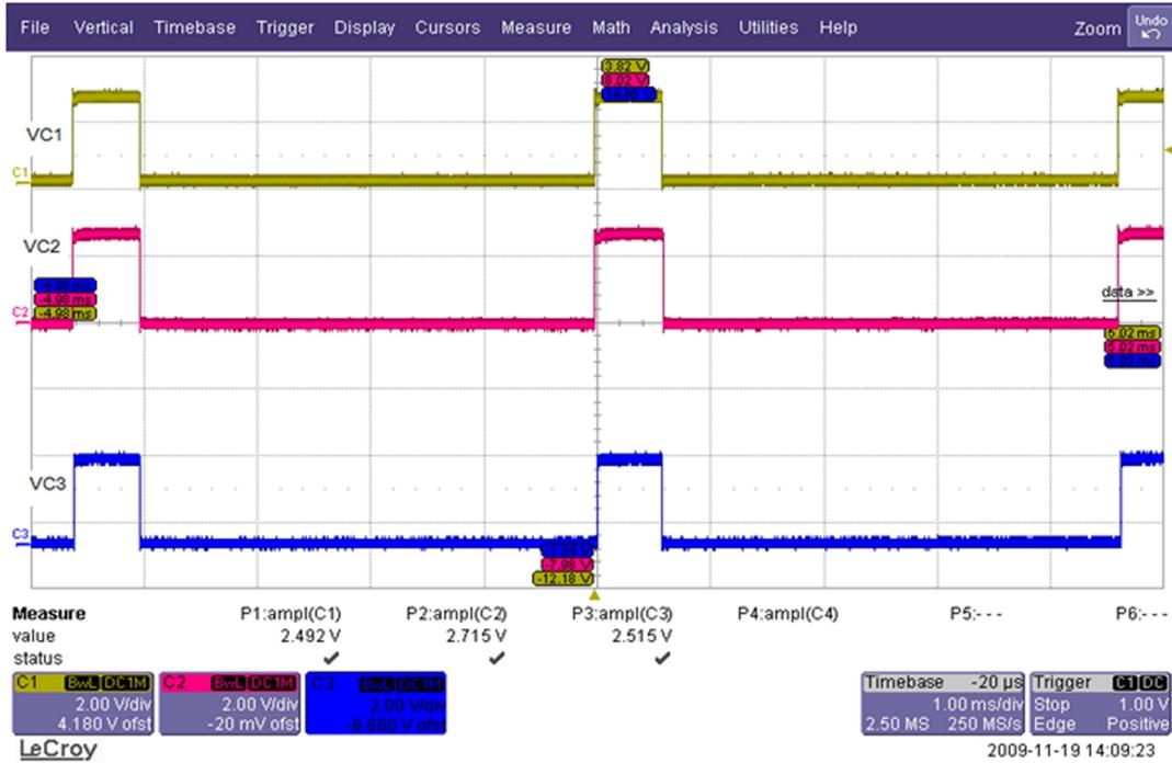
Figure 47 TX HB FEM logic waveform (C1:VC1; C2:VC2; C3:VC3)
