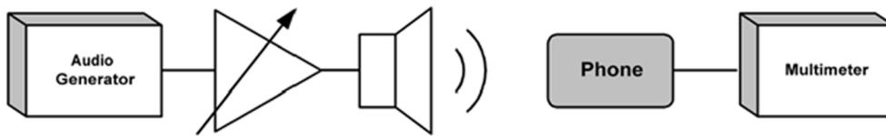
Figure 35 Test arrangement for external microphone
