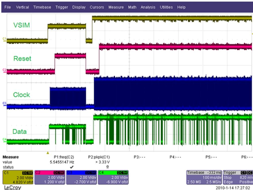
Figure 19 SIM voltages, normal startup at 3V
