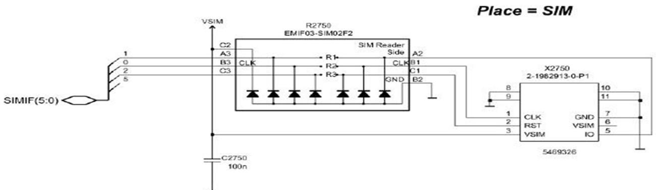
Figure 64 SIM card holder and signal protection
