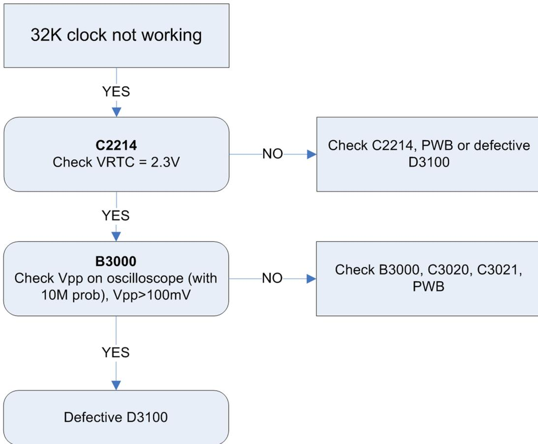
Figure 14 32 KHz RTC clock does not work
