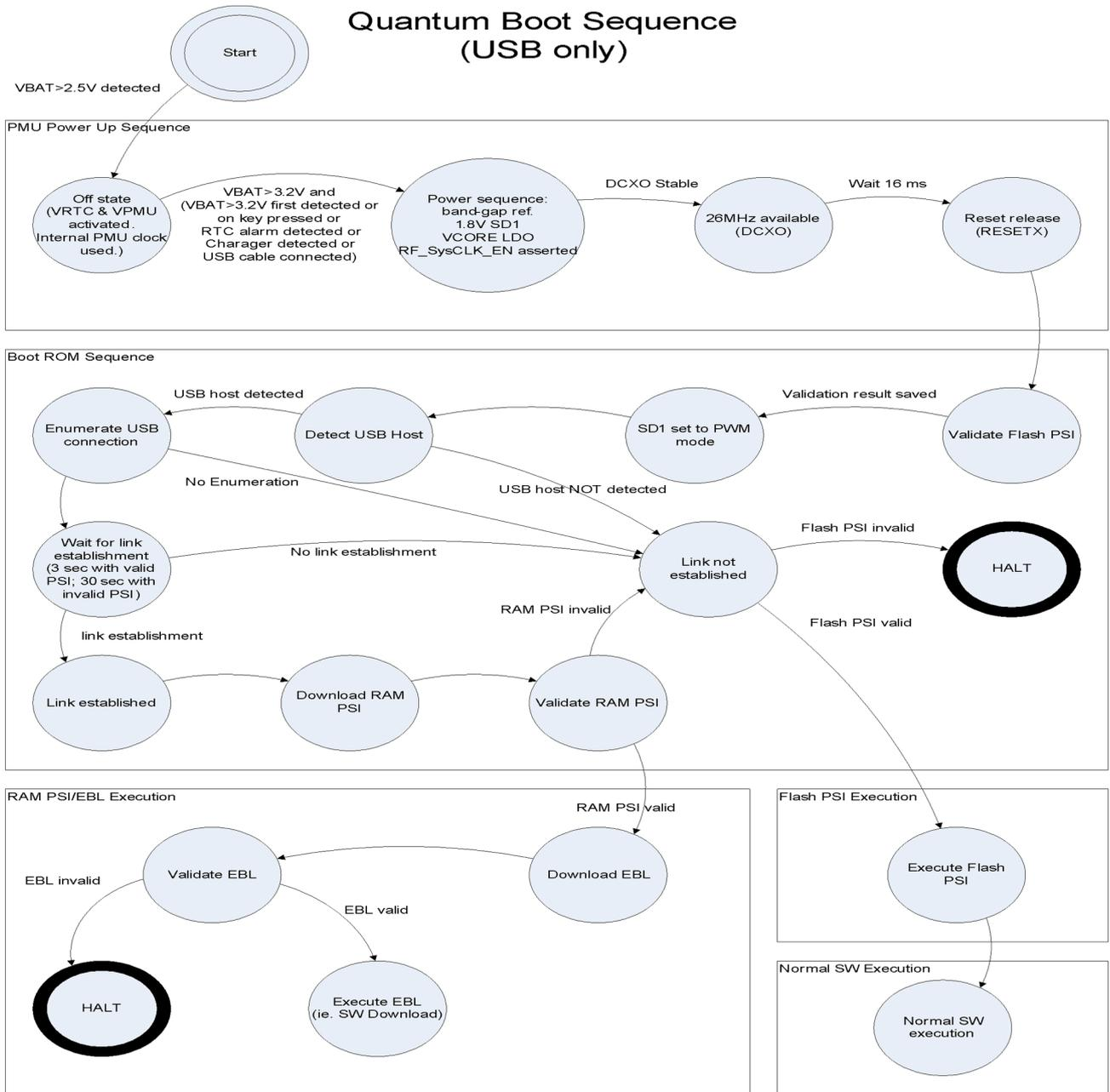
Figure 53 System startup, SW view
