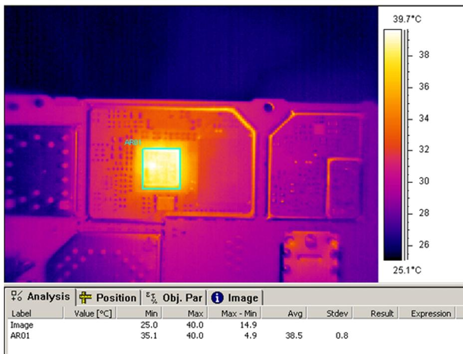
**Figure 9 IR picture showing component overheat**
