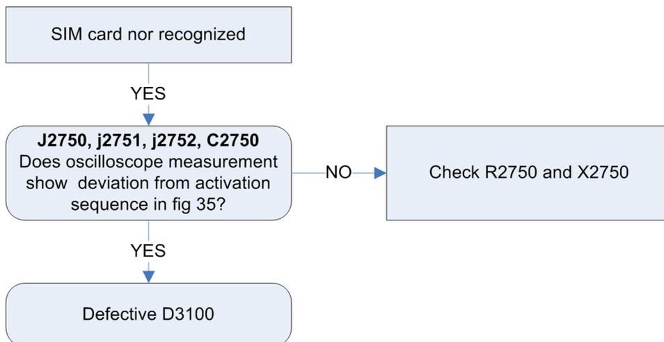
Figure 17 Cannot identify SIM card
