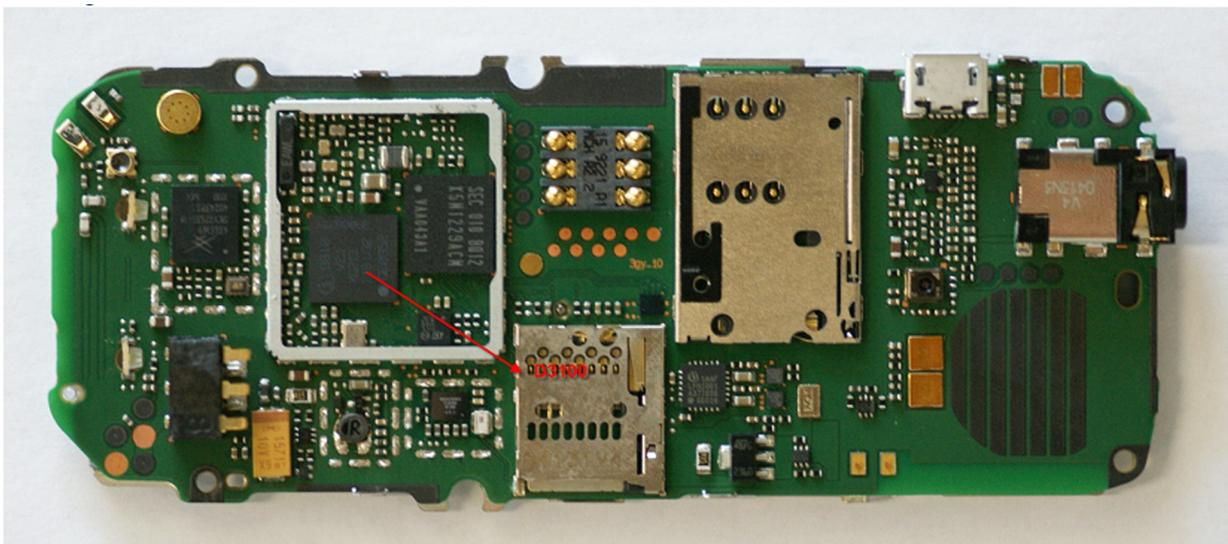
Figure 38 D3100 is the non-reworkable components on PWB
