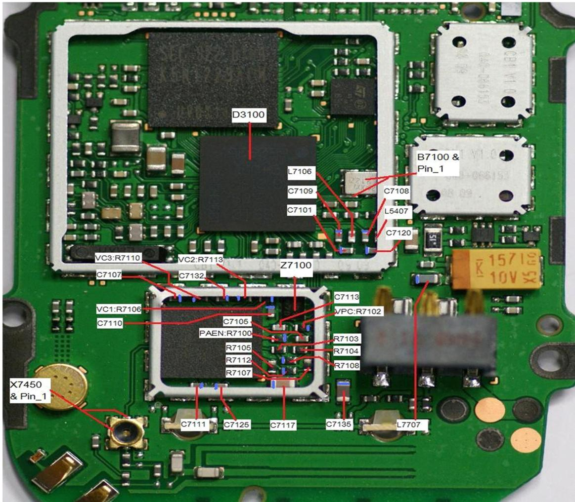
Figure 43 TX checkpoints and component overview (measurement point marked with blue)
