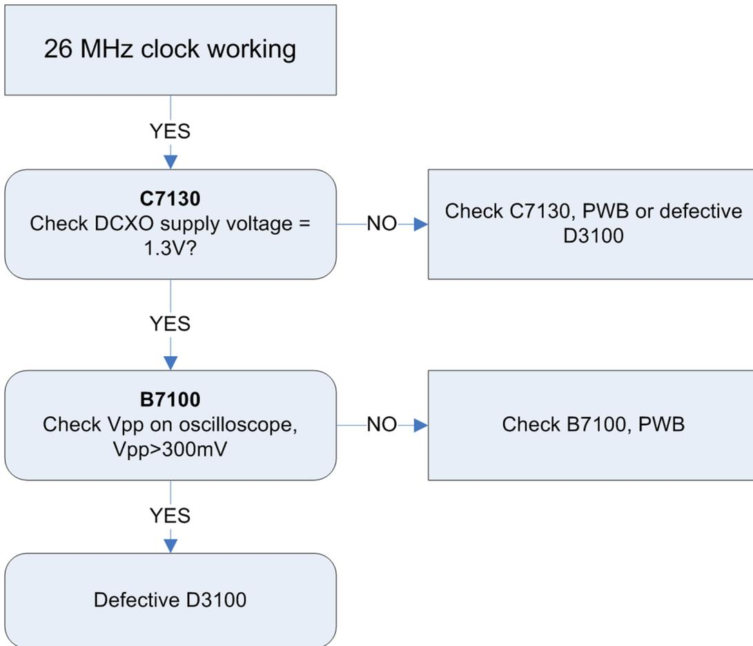
Figure 13 26 MHz Clock does not work
