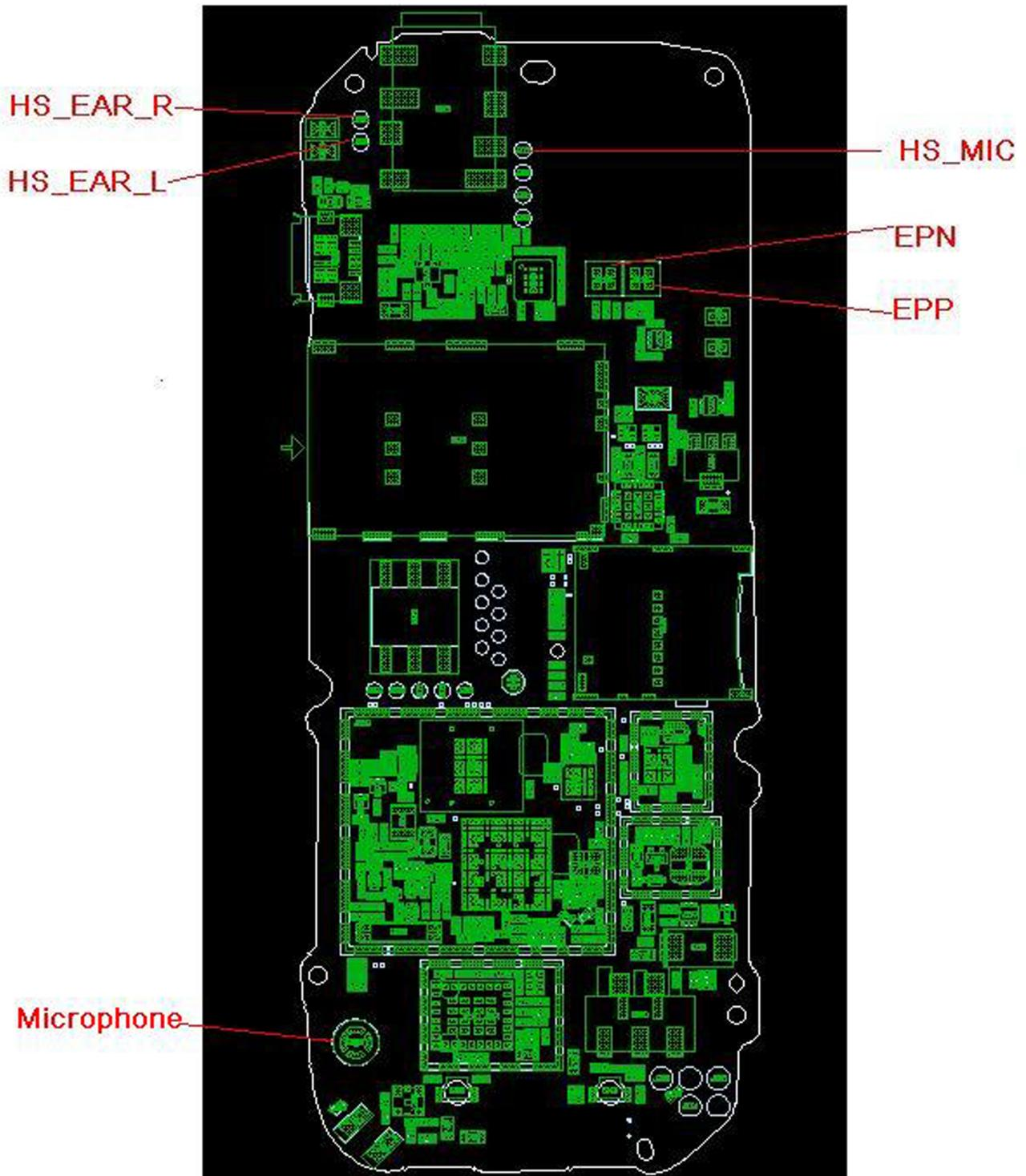
Figure 28 PWB audio test point
