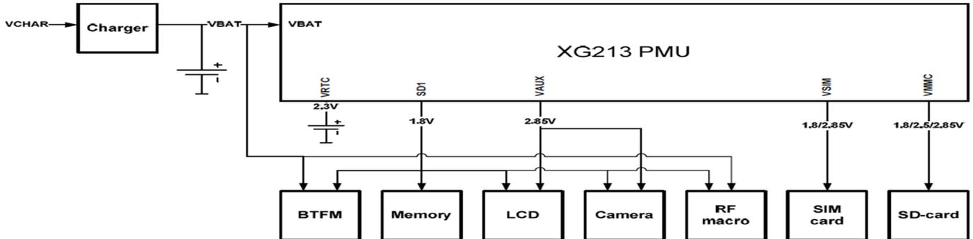
**Figure 55 Power supply distribution**
