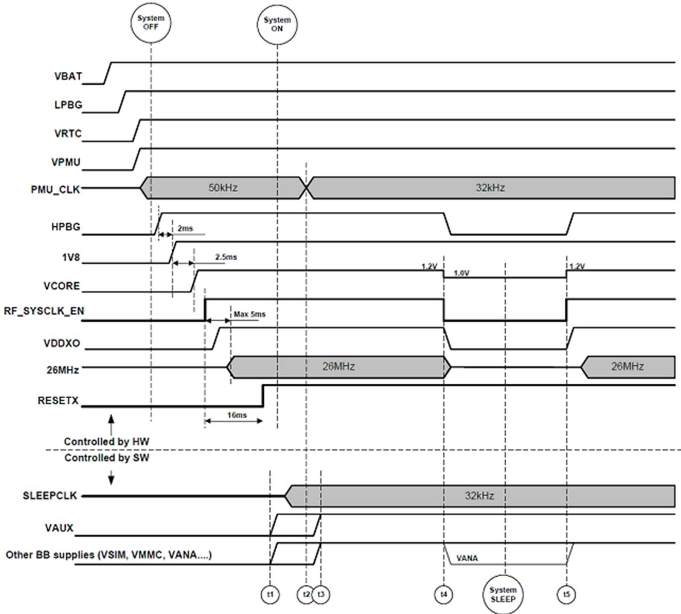
Figure 52 Power up timing and system sleep
