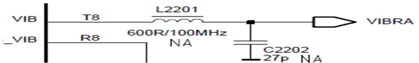
Figure 70 Vibrator circuits
