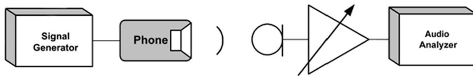
Figure 37 Test arrangement for headset speaker
