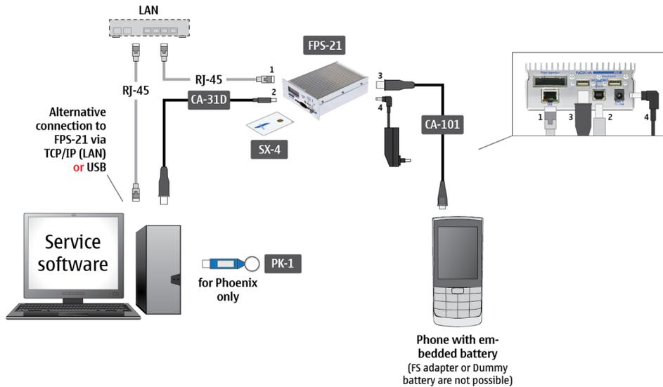
**Figure 3 Flashing, certificate restore and product code change**
