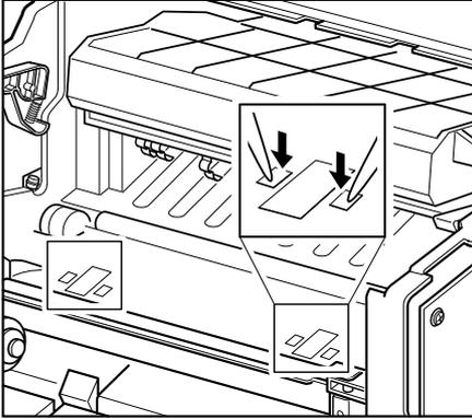
2. Turn the unit over again, and remove the actuator feed.
