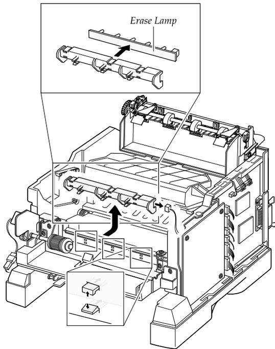
3. Remove three screws and raise the guide feed in the direction of arrow.
