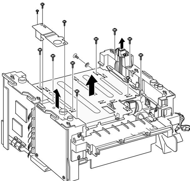
5. Unplug all connectors from the PCU shield, and remove the shield.
