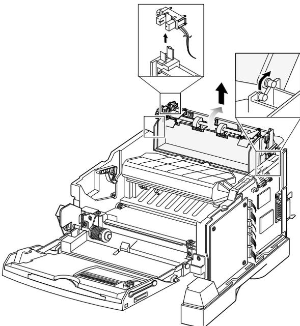
3. If you want to remove the roller shaft, unlatch both ends of the shaft and take it out.
