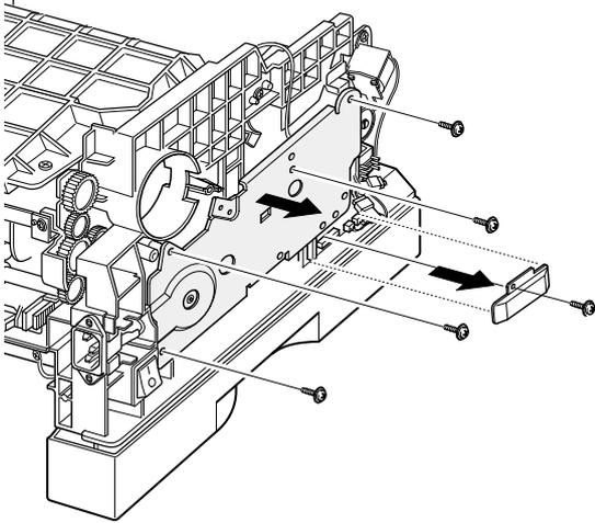
4. If you want to remove the step motor, remove four screws securing the step motor from the motor bracket and unplug two connector from the motor.
