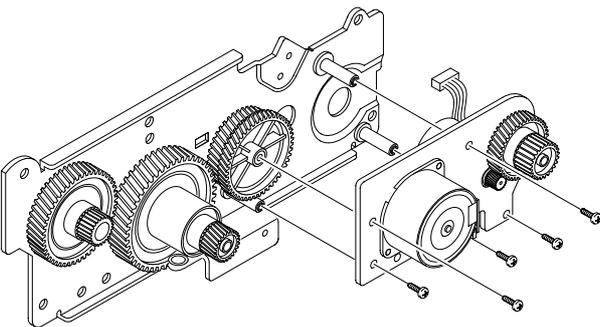
5. If you want to remove the motor joint PCB, remove two screws securing the motor joint PCB from the gear bracket and unplug one connector from the motor joint PCB.
