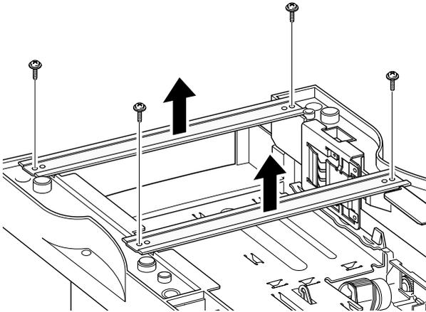
2. Remove three screws from the left base bracket, and take the bracket out.
