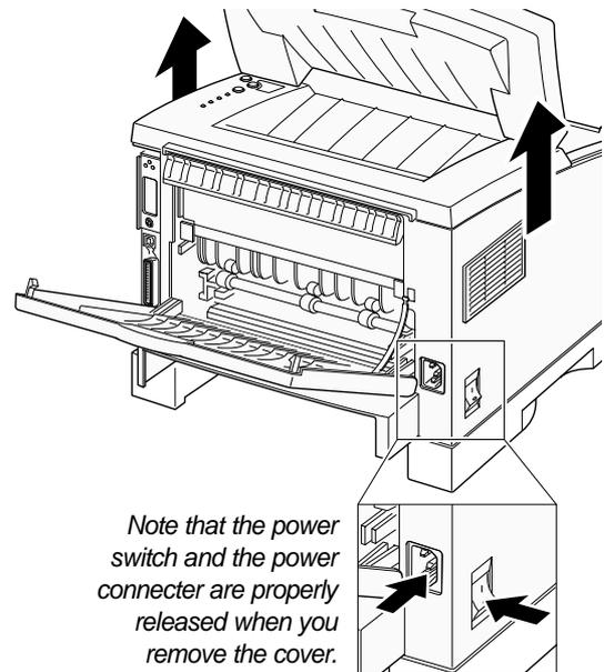
*Note that the power switch and the power connector are properly released when you remove the cover.*
