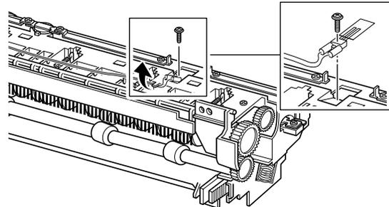
◆ To remove the halogen lamp from the fuser assembly :
