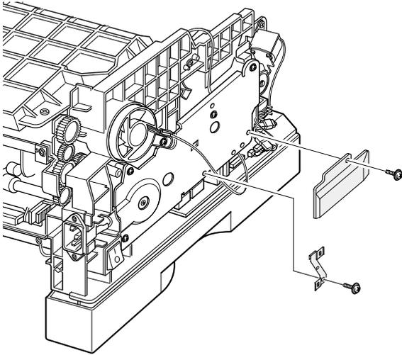
3. Remove one screw, and remove the fan. Then unplug one connector.
