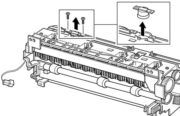
◆ To remove the thermistor from the fuser assembly :
