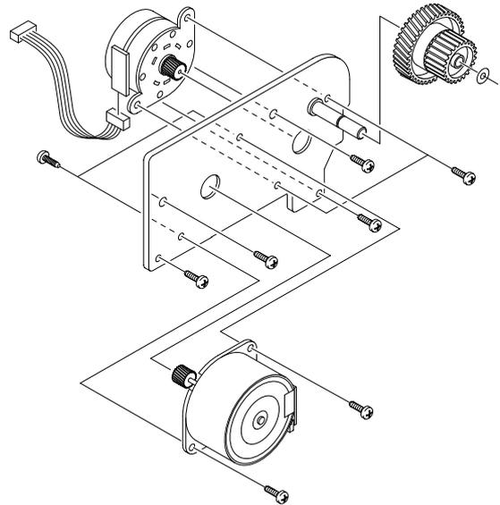
3. If you want to remove the motor assembly from the drive assembly, remove five screws securing the motor assembly to the gear bracket.
