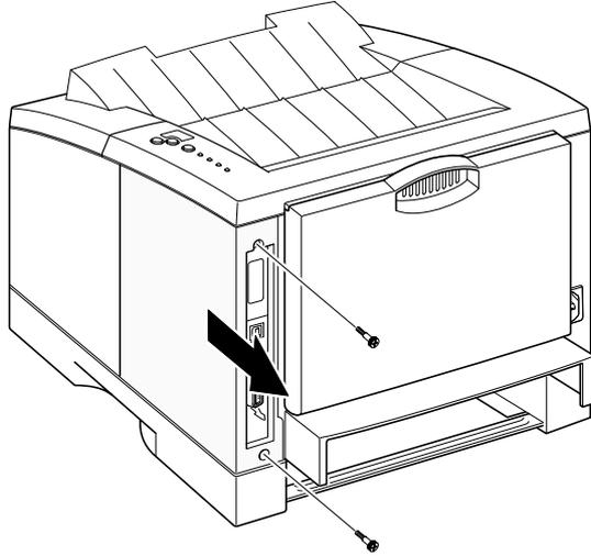
2. Remove five screws securing the board and unplug all connectors, and then take the controller board out of the printer.
