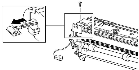
**Note** When you reassemble the halogen lamp, make sure that it is inserted into the slot properly.
