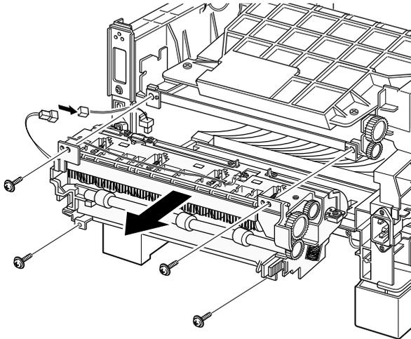
◆ To remove the thermostat from the fuser assembly
