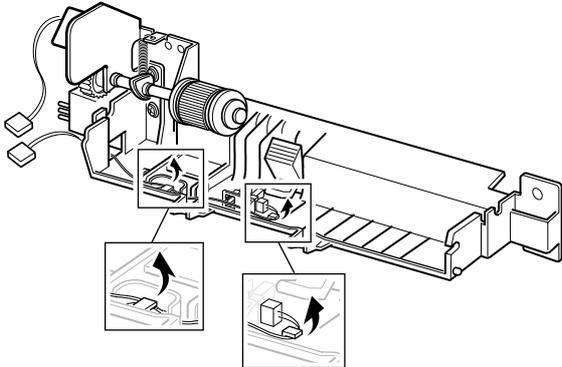
2. Raise the pickup holder in the direction of arrow.
