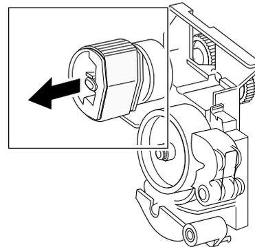
*Squeeze this tab to remove the rubber.*
