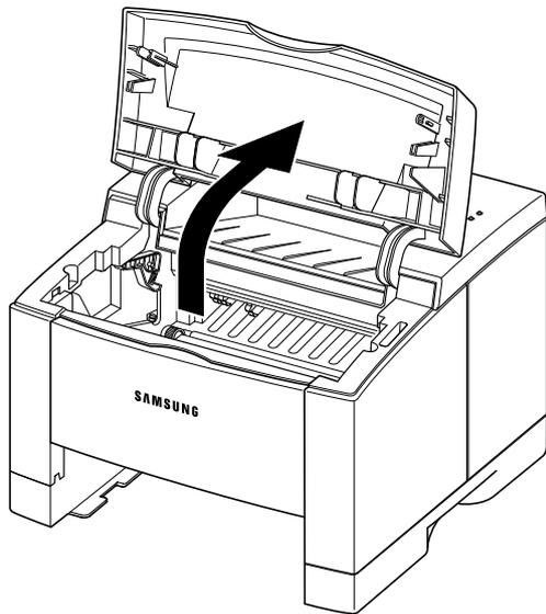
3. Hold the cap at the both end of the roller, then remove the roller.
