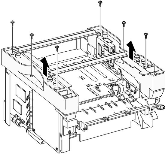
4. While you push the latch to release the PCU shield, take the PCU shield out of the printer.
