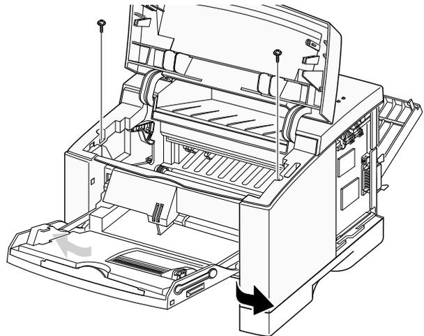
6. Slide the main cover upward, out of the printer.
