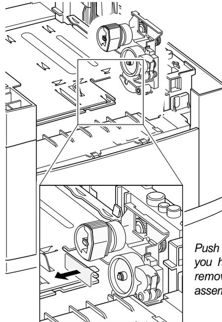
*Push the solenoid if you have difficulty to remove the pickup assembly.*
