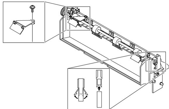
4. If you want to remove the exit roller, squeeze the bottom of the roller and take it out.
