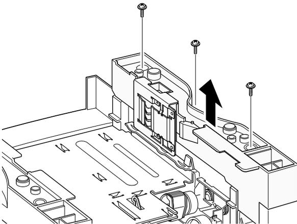
3. Remove four screws securing the pickup assembly.
