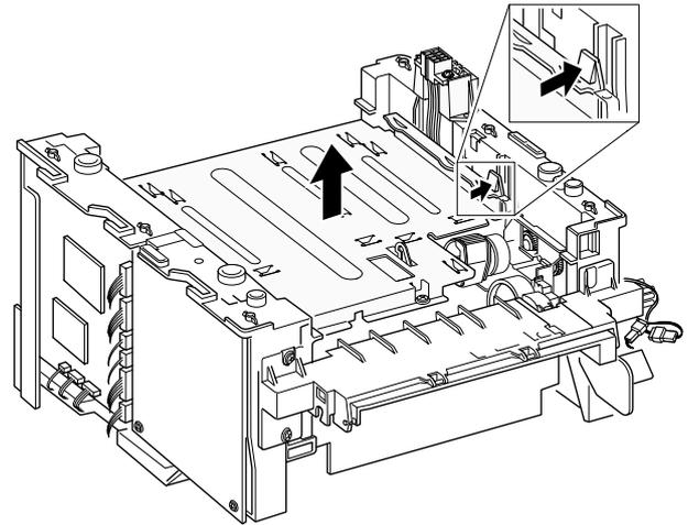
3. Remove eight screws securing the PCU shield and remove two screws securing the SCF connector, and then take the PCU shield out of the printer.
