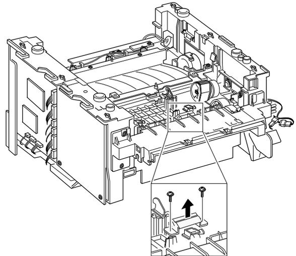
◆ To replace the fuser sensor :
