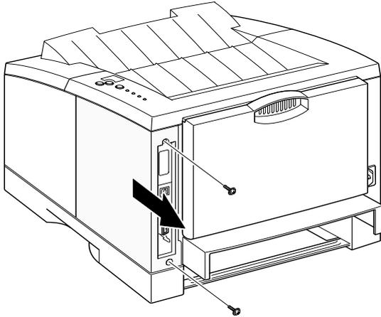
2. Remove two screws at the back of the printer and unplug one connector from the board, then open the rear cover.
