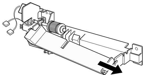
◆ To replace the Paper Empty (PE) sensor :
