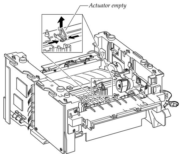
◆ To replace the actuator feed
