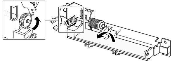
2. Remove the spring , then release the right end of the plate.
