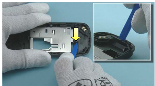
24) Use the sharp end of the SS-93 to release the ANTENNA MODULE clip and then use the flat end of the SS-93 to release the bottom end of the ANTENNA MODULE.
