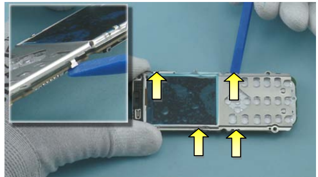
26) Release the four clips holding the UI SHIELDING with the SS-93.
