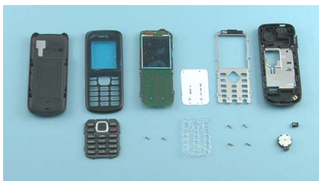
33) The Nokia C1-02 disassembly is now complete.
