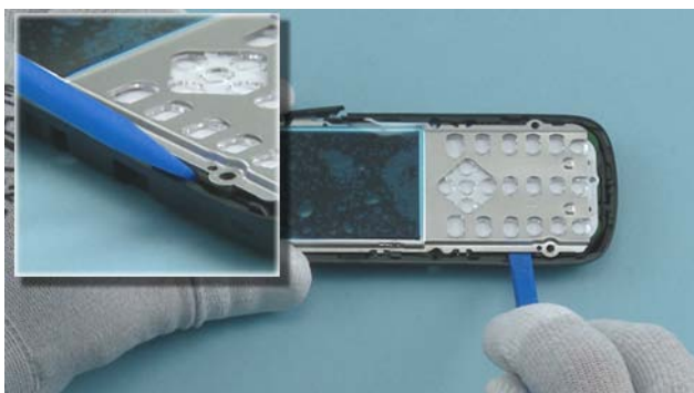
17) Release also the other side with the SS-93.
