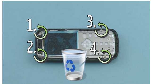
14) Unscrew the four Torx+ size 6 screws. Do not use them again. Discard them.
