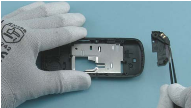
25) Remove the ANTENNA MODULE with the tweezers.
