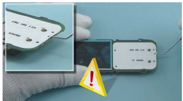
30) Use the dental tool to release the DOMESHEET. Be careful not to injure yourself with the sharp end of the dental tool!
