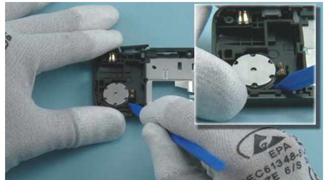
20) Use the sharp end of the SS-93 to release the EARPIECE / SPEAKER / VIBRA.
