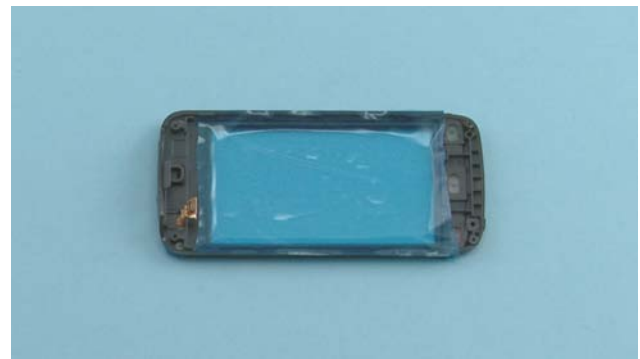
22. Protect also the TOUCH PANEL from the inside with protective film.
