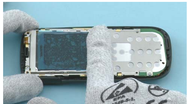
10) Protect the LCD with a protective film.
