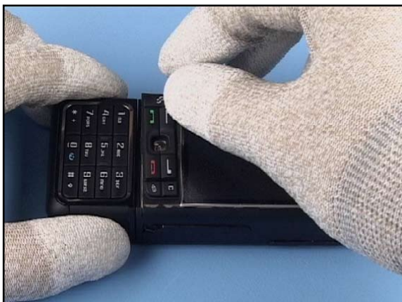
29. Insert the KEYMAT ASSEMBLY SYMBIAN.
