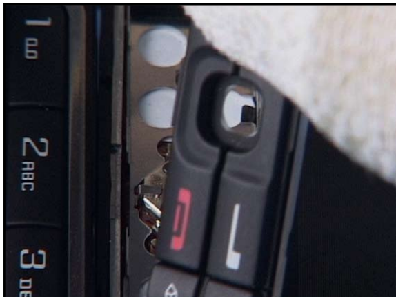
7. Remove the KEYMAT ASSEMBLY SYMBIAN.
