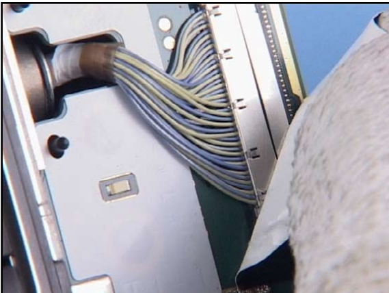
9. Peel up the COAX CABLE SUPPORT TAPE
