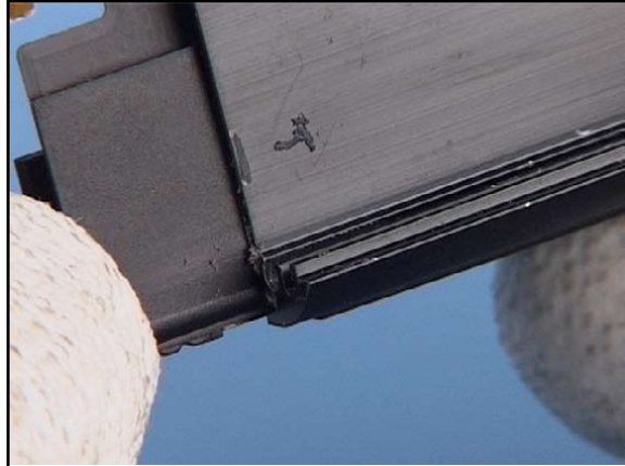
2. Shift the MAIN FLEX ASSEMBLY into the UPPER FRAME ALUMINIUM.
