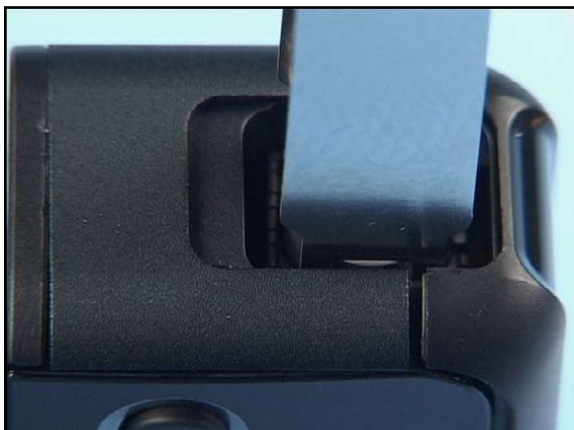
23. Place the camera into its housing.
