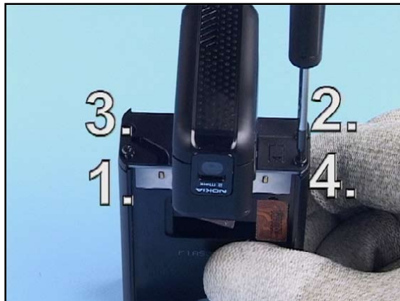
22. Unscrew the 4 screws in the order shown.
