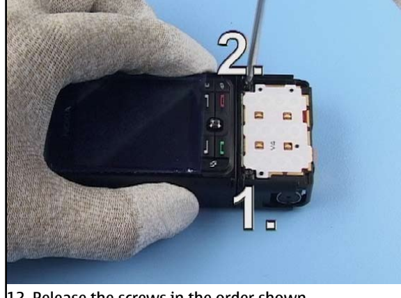
12. Release the screws in the order shown.
