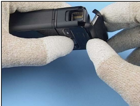
20. Fix all the parts while placing the LOWER CAP COVER.
