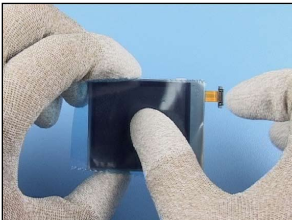
13. Cover the display with a protective film.
