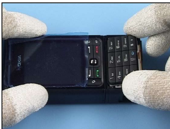
18. Insert the KEMAT ASSY NUMERIC and fix the snaps.
