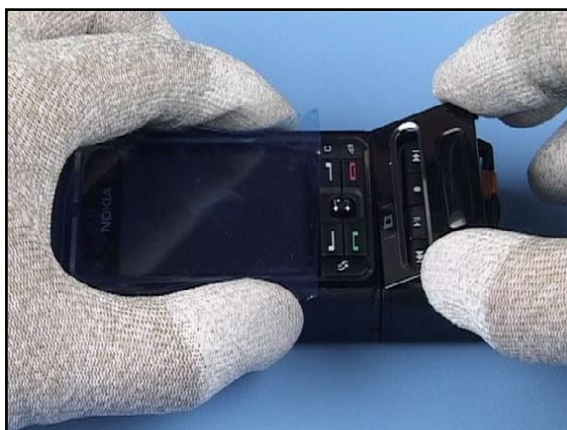
16. Insert the LOWER BACK COVER and fix the snaps.
