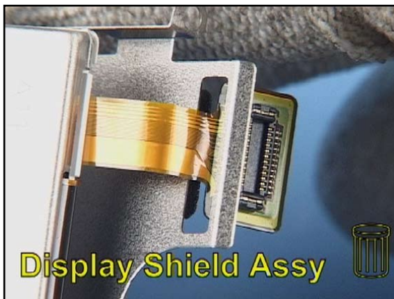
12. Carefully slot through the flex connector. Always use a new DISPLAY SHIELD ASSEMBLY when reassembling.
