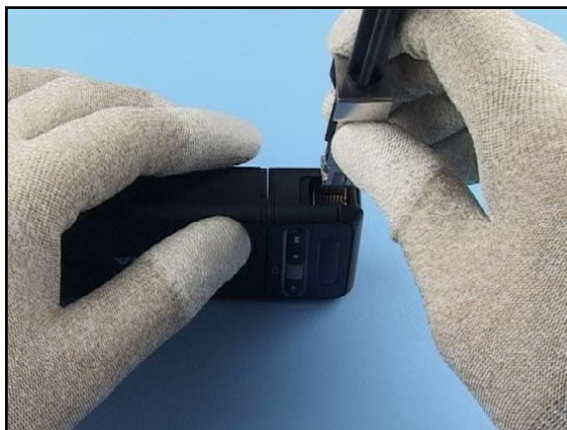
22. Grip the camera with the SS-45.
