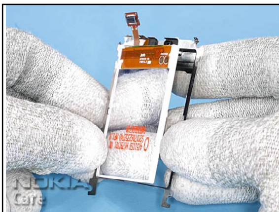
16. Separate the DISPLAY from the UI-SHIELD.
