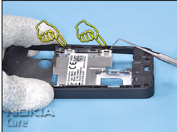
20. First unlock the metal clips of the LABEL COVER ASSY on the shown side.
