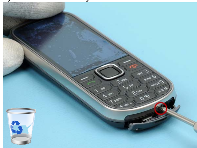
6) Unscrew the SCREW with Torx 6+.
