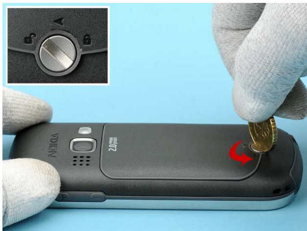
1) Use a coin to unlock the C-COVER ASSY in the direction shown.
