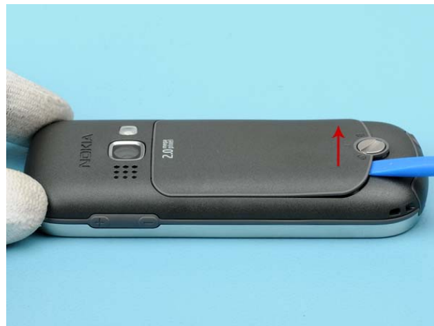
2) Lift up the C-COVER ASSY using SS-93.
