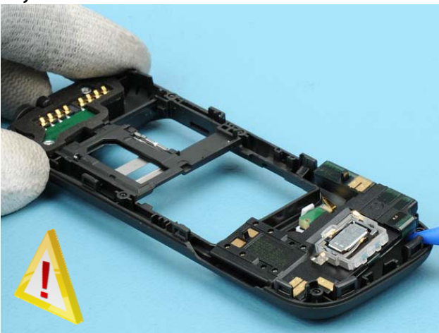
25) Carefully remove the ANTENNA MODULE ASSY using SS-93.
