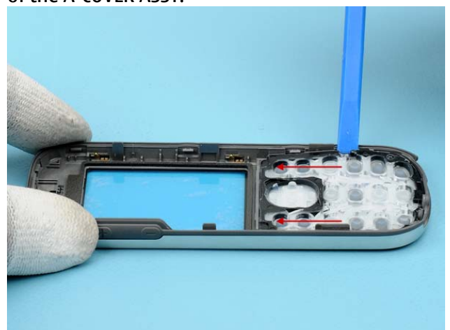
12) Lift up the KEYPAD with SS-93 from both sides.
