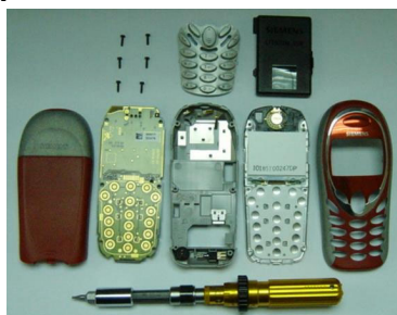
Fully disassembled A55
