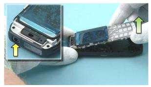
16) Lift up the bottom end of the LIGHT SWAP PACKAGE to release the AV jack.
