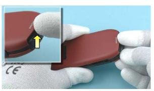
4) Use the opening notch to release the B-COVER.
