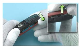
7) Then release both top side corners of the A-COVER 8) Remove the A-COVER ASSEMBLY. ASSEMBLY.
