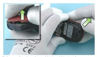
6) Start releasing the A-COVER ASSEMBLY by releasing both of the bottom corners as shown.
