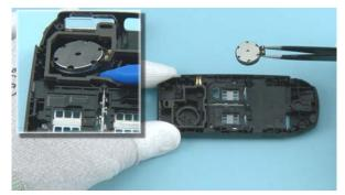
18) Lift up the SPEAKER with the sharp end of the SS-93 and remove it with the tweezers.
