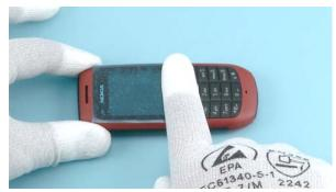
3) Protect the A-COVER ASSEMBLY window with a protective film.
