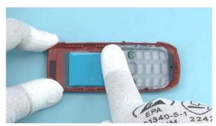
10) Also protect the other side of the A-COVER ASSEMBLY window with protective film.
