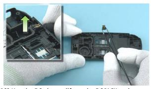
19) Use the DC plug to lift up the DC JACK and remove it with the tweezers.
