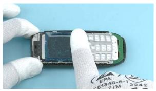
9) Protect the LCD with protective film.
