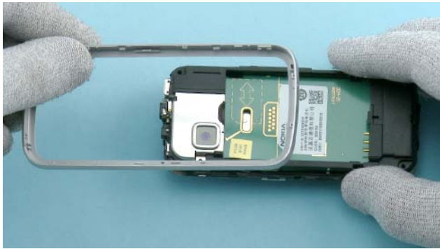
13) The A-COVER can now be separated.
