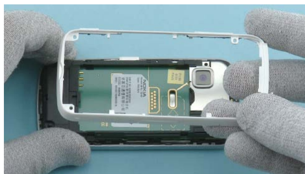
8) Release also the snaps on the other side with the SRT-6. Remove the SIDE BAND ASSY.
