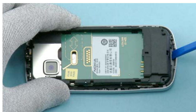
12) Then release the remaining clips on both sides of the phone.
