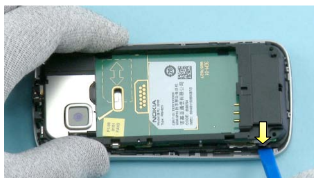
10) To remove the A-COVER, first release the clip from the bottom corner with the SS-93.
