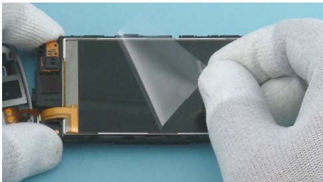
17) Remove the protective film from the LCD.
