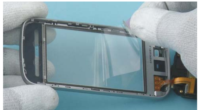
18) Remove the protective film from the TOUCH PANEL ASSY and..
