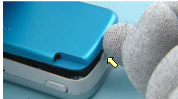
4) Use the opening notch to release the BATTERY COVER.
