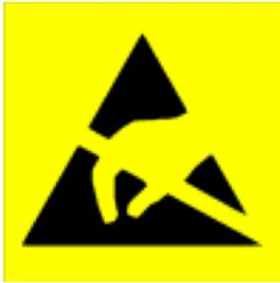
Any product of which the covers are removed must be handled with ESD protection. The SIM card can be replaced without ESD protection if the product is otherwise ready for use.
