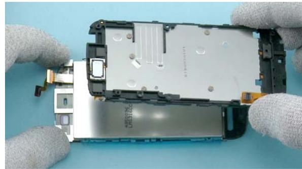
32) Remove the LCD FRAME ASSY.
