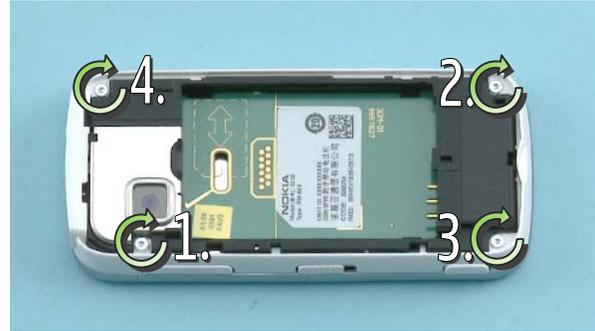
2) Tighten the screws to the torque of 17 Ncm in the order shown.
