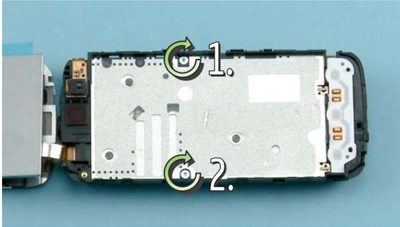
1) Tighten the 2 screws to the torque of 16 Ncm in the order shown.
