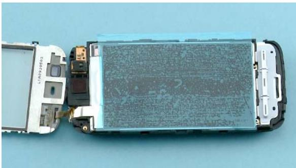
15) Protect the LCD with a protective film.
