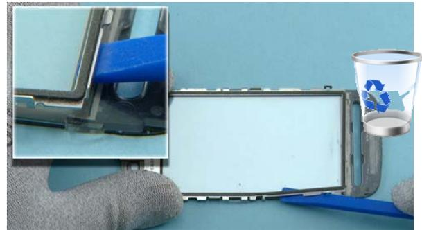
40) Use the SS-93 to detach the TOUCH FRAME ASSY from the TOUCH PANEL ASSY. TOUCH FRAME ASSY and TOUCH PANEL ASSY can now be separated. Do not use the TOUCH FRAME ASSY again. Discard it.
