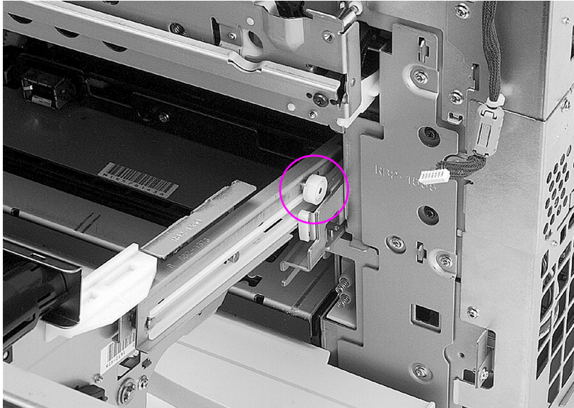
Figure 6-10 ITB drawer (middle drawer) removal and replacement
