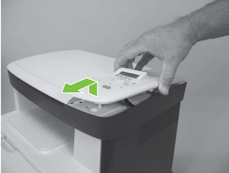
Figure 6-6 Remove the control-panel (2 of 3; base model)
