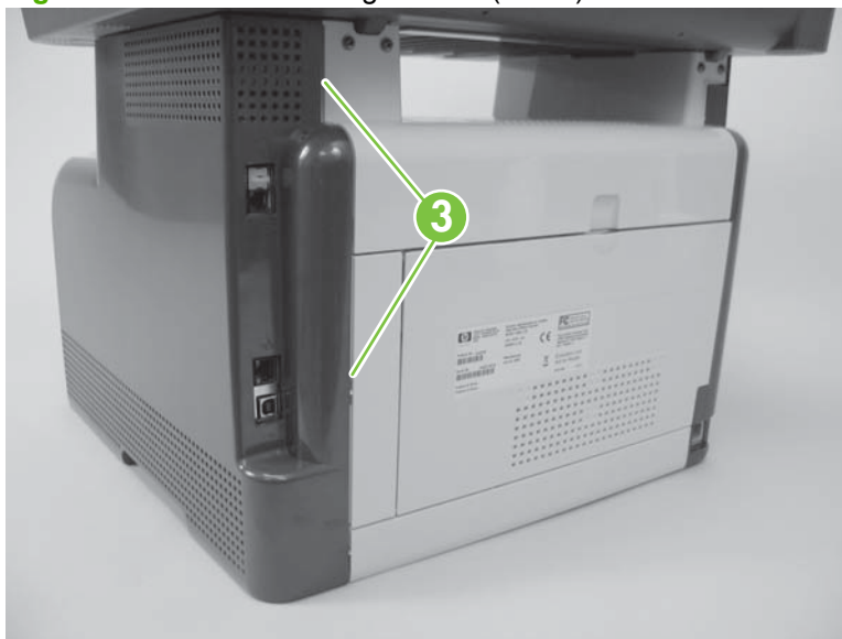
Figure 6-38 Remove the right cover (4 of 5)
