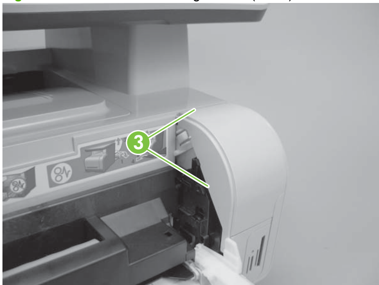
Figure 6-45 Remove the front-right cover (2 of 3)
