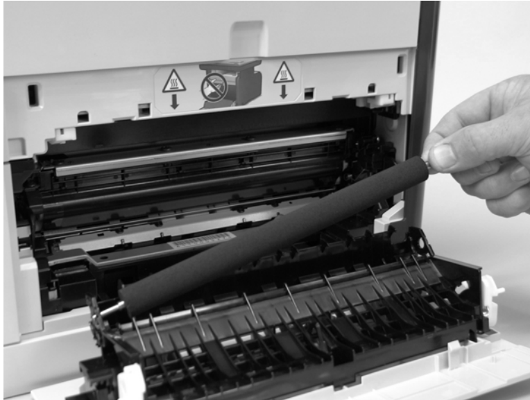
Figure 6-19 Remove the transfer roller (3 of 3)
