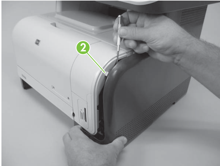
Figure 6-37 Remove the right cover (3 of 5)
