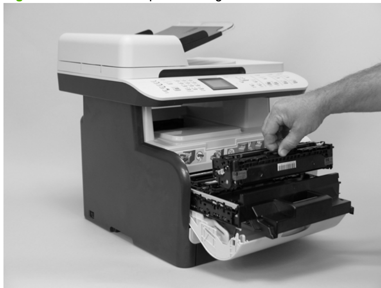
Figure 6-3 Remove the print cartridge
