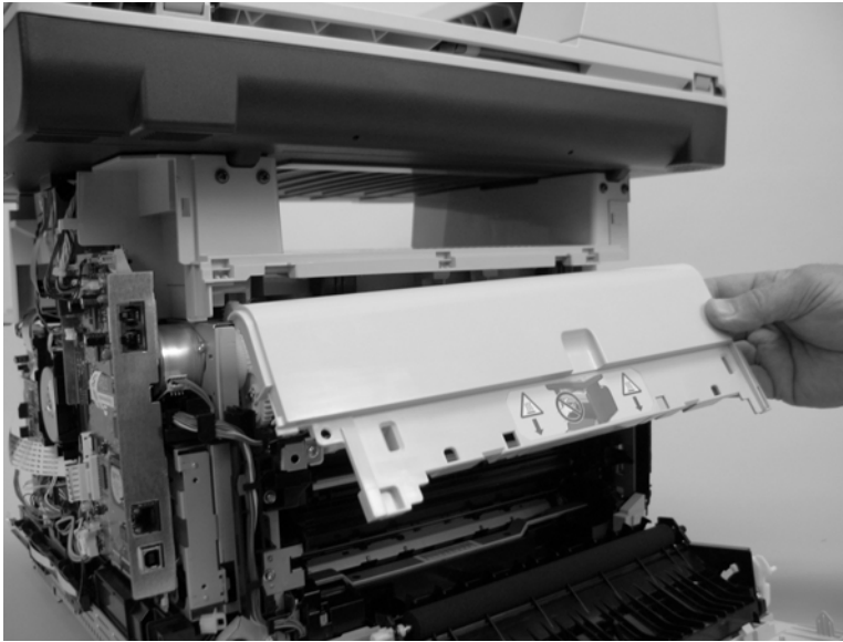
Figure 6-54 Remove the rear-upper cover (2 of 2)
