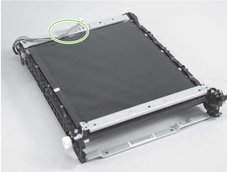
Figure 6-81 Reinstall the ITB (2 of 2)
