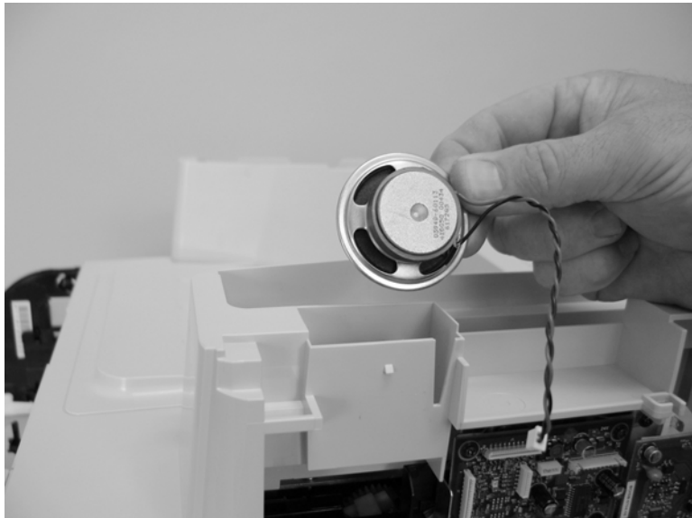
Figure 6-74 Remove the speaker (2 of 2)
