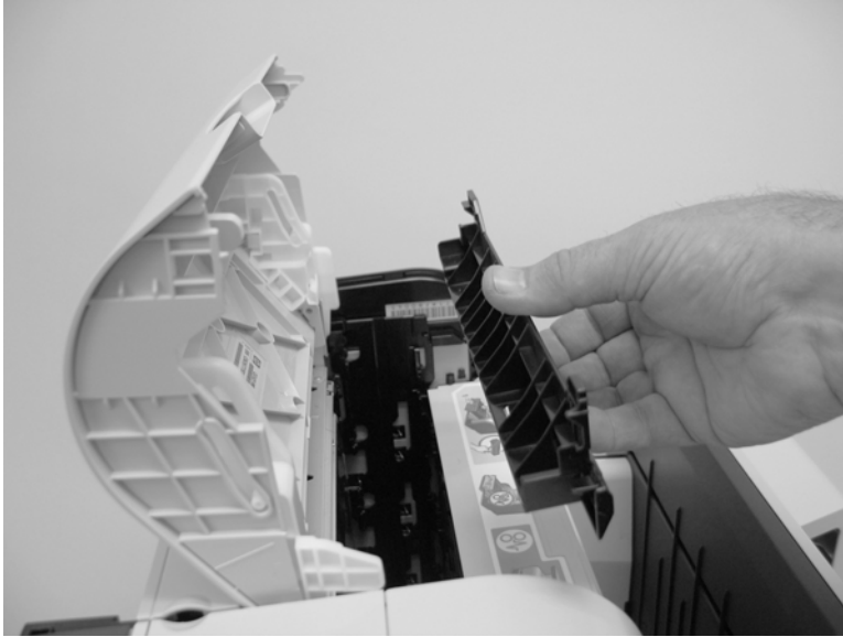
Figure 6-28 Remove the front door and front-lower cover (7 of 13)
