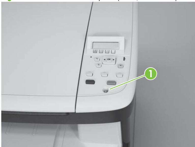
Figure 6-5 Remove the control-panel (1 of 3; base model)
