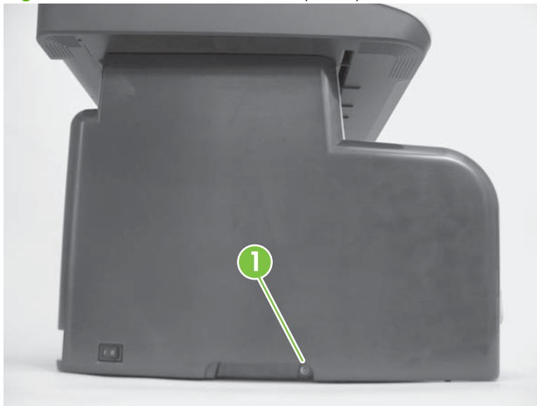
Figure 6-40 Remove the left cover (1 of 4)
