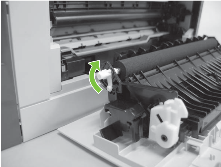
Figure 6-17 Remove the transfer roller (1 of 3)
