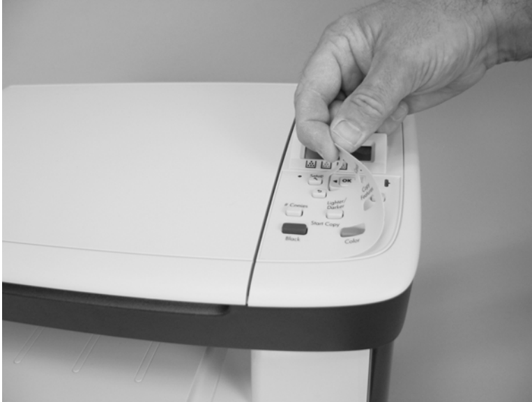
Figure 6-4 Remove the control-panel overlay (base model)
