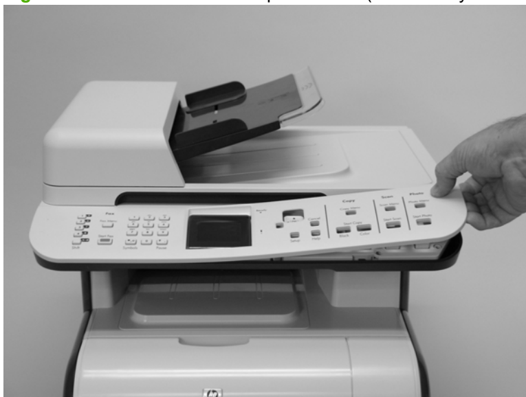
Figure 6-8 Remove the control-panel bezel (fax/memory-card models)
