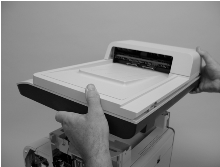
Figure 6-62 Remove the scanner assembly (4 of 4)
