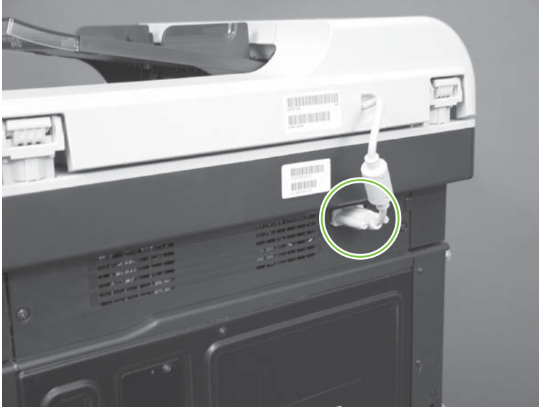
Figure 6-46 Remove the ADF assembly (1 of 4)
