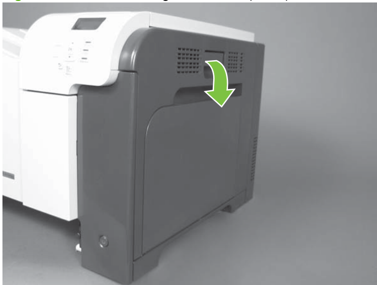
Figure 6-77 Remove the right-rear cover (1 of 3)
