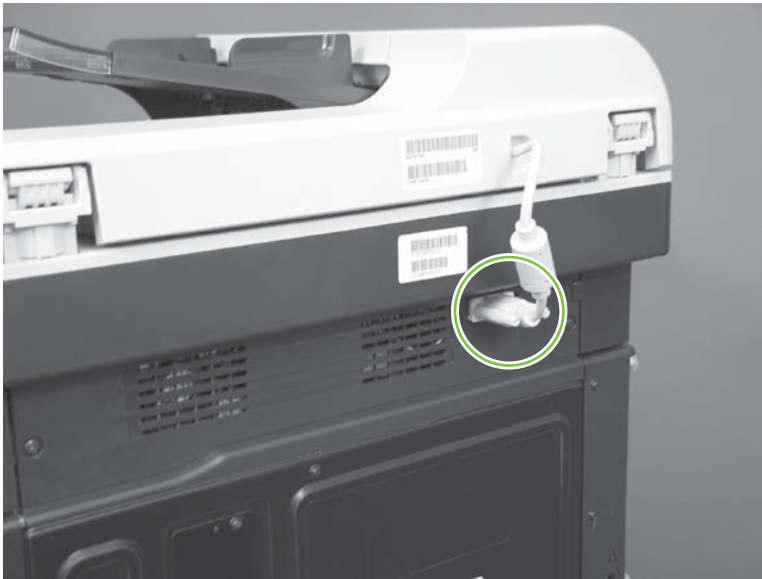
Figure 6-85 Remove the rear-upper cover (1 of 4)
