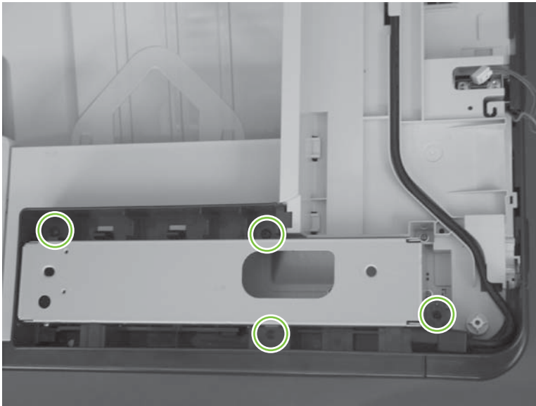
Figure 6-124 Remove the right-top cover (1 of 5)
