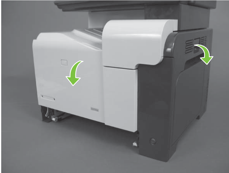
Figure 6-65 Remove the front-upper cover (1 of 4)
