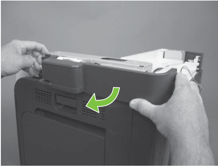
Figure 6-117 Remove the front stapler cover and right-side stapler cover (10 of 13)
