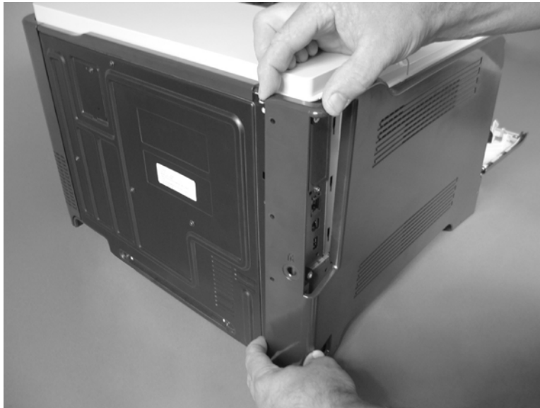
Figure 6-81 Remove the left cover (2 of 5)
