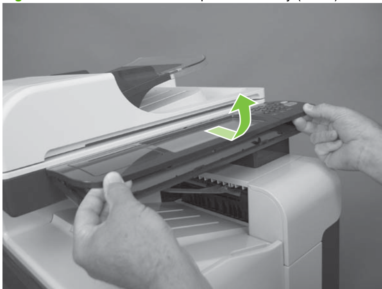
Figure 6-59 Remove the control-panel assembly (2 of 3)
