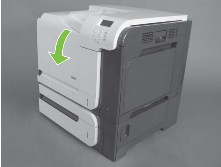
Figure 6-10 Remove the toner-collection unit (1 of 4)
