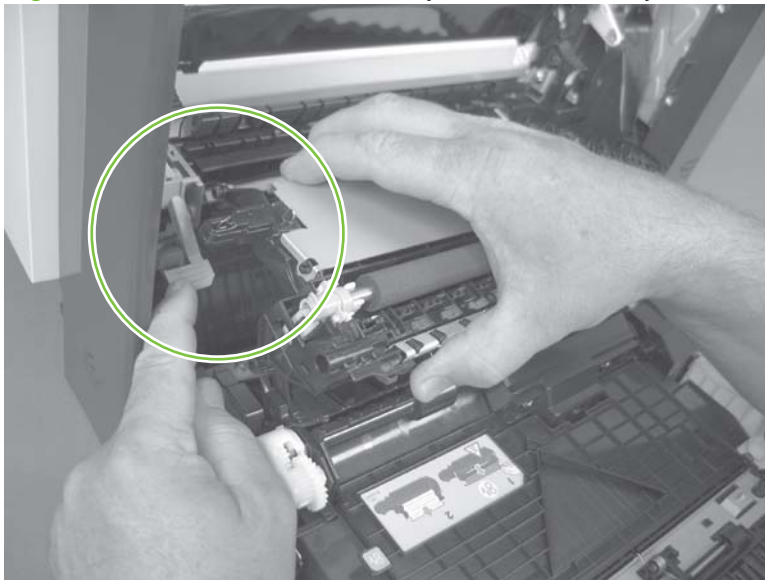
Figure 6-40 Reinstall the secondary transfer assembly
