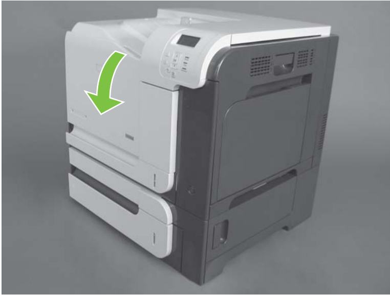
Figure 6-5 Remove the print cartridge (1 of 2)
