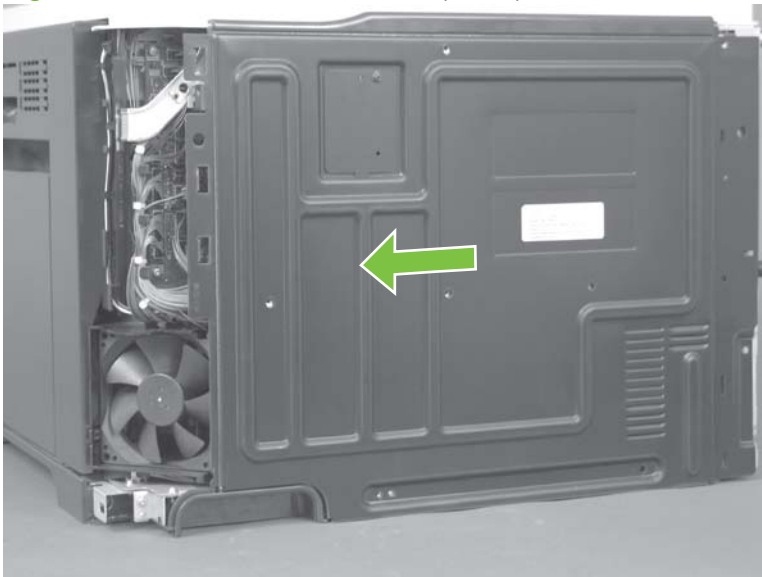
Figure 6-90 Remove the rear cover (2 of 2)
