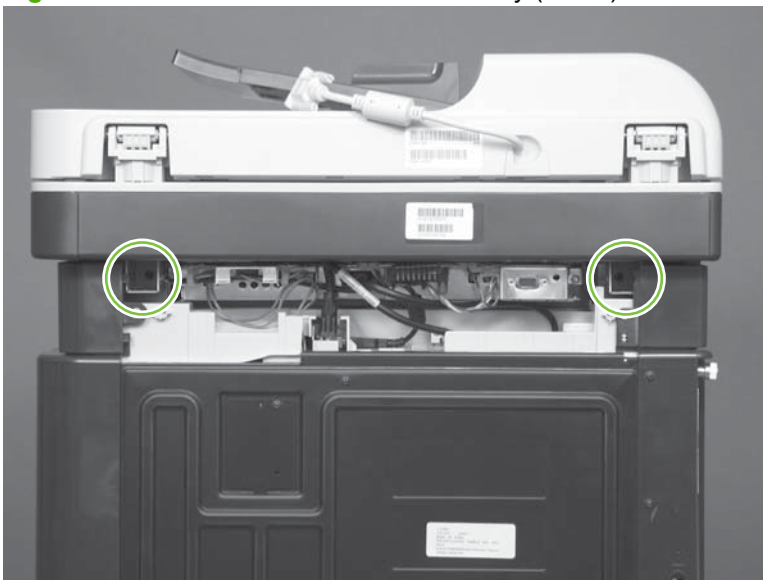
Figure 6-98 Remove the scanner assembly (2 of 6)
