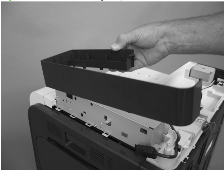
Figure 6-128 Remove the right-top cover (5 of 5)
