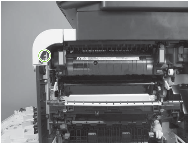
Figure 6-66 Remove the front-upper cover (2 of 4)
