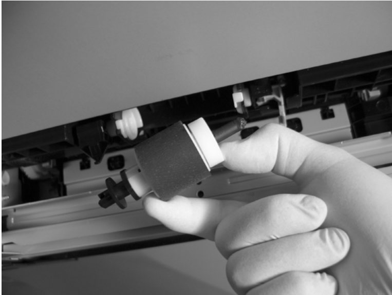
Figure 6-29 Remove the pickup roller (Tray 2) (4 of 4)
