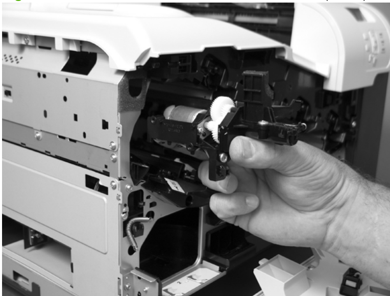
Figure 6-185 Remove the residual-toner-feed motor (7 of 7)
