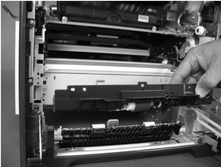
Figure 6-230 Remove the cassette-pickup assembly (3 of 3)
