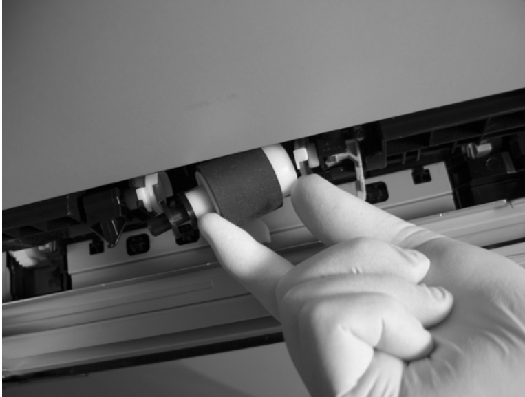
Figure 6-28 Remove the pickup roller (Tray 2) (3 of 4)
