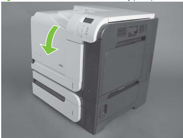
Figure 6-44 Remove the front-door assembly (1 of 2)
