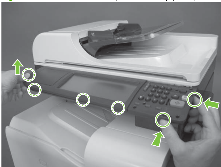
Figure 6-58 Remove the control-panel assembly (1 of 3)
