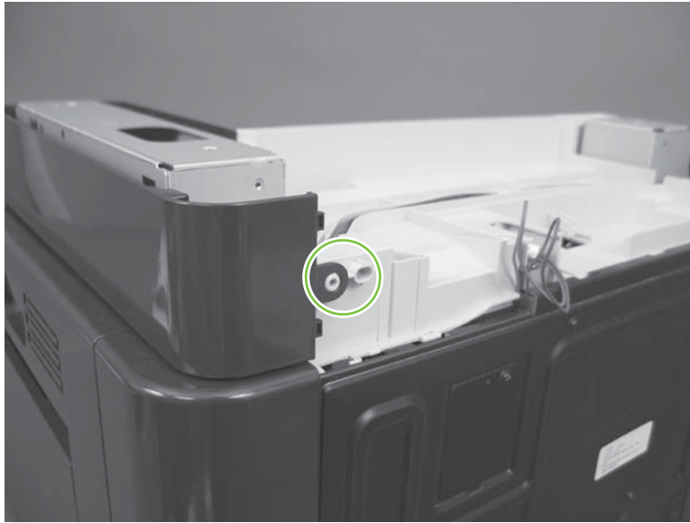
Figure 6-125 Remove the right-top cover (2 of 5)
