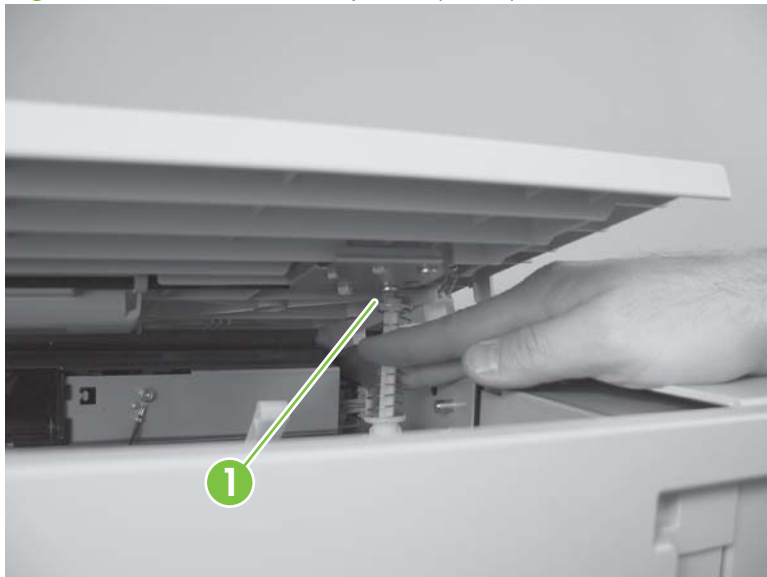
Figure 8-150 Remove the top door (2 of 3)
