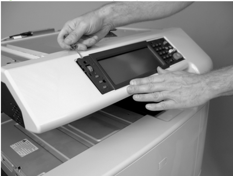
Figure 6-163 Remove control panel (2 of 3)
