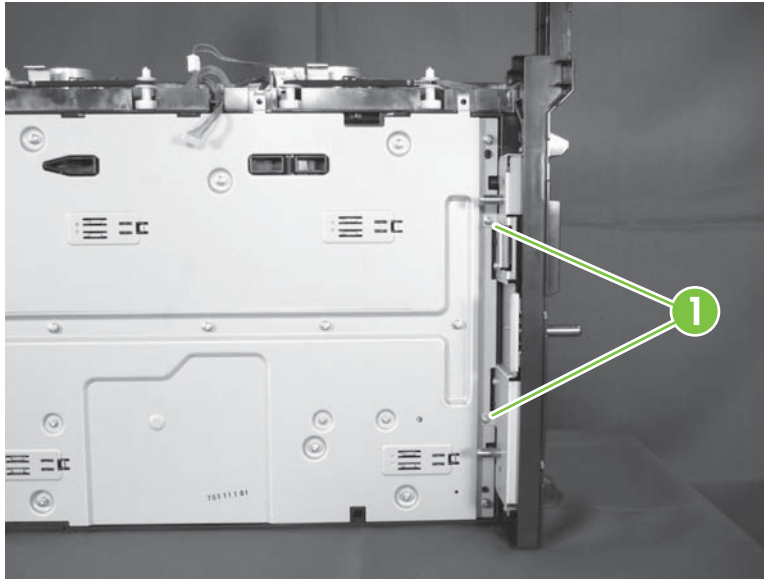
Figure 8-124 Remove the finisher lock-assembly (3 of 4)
