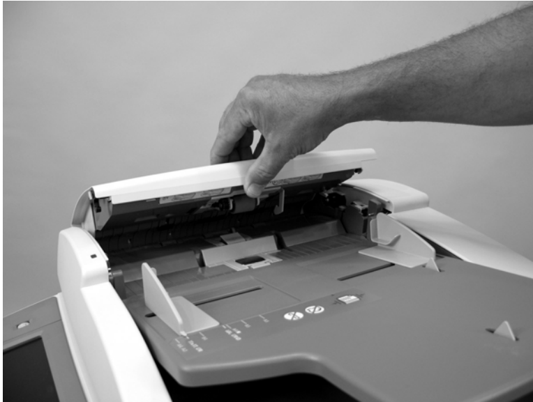
Figure 6-213 Remove the ADF separation floor assembly (1 of 4)
