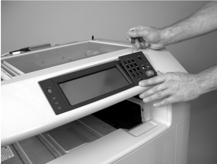
Figure 6-163 Remove control panel (2 of 3)
