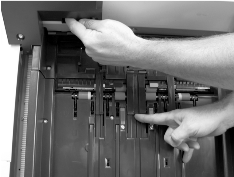
Figure 8-199 Remove output-bin 1 (3 of 3)
