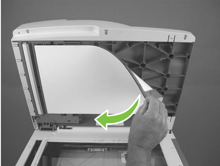
Figure 6-228 Remove the ADF white backing (1 of 4)
