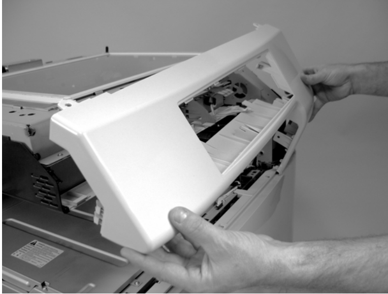
Figure 6-166 Remove front cover (2 of 2)
