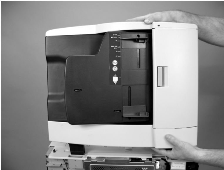
Figure 6-210 Remove the ADF assembly (4 of 4)
