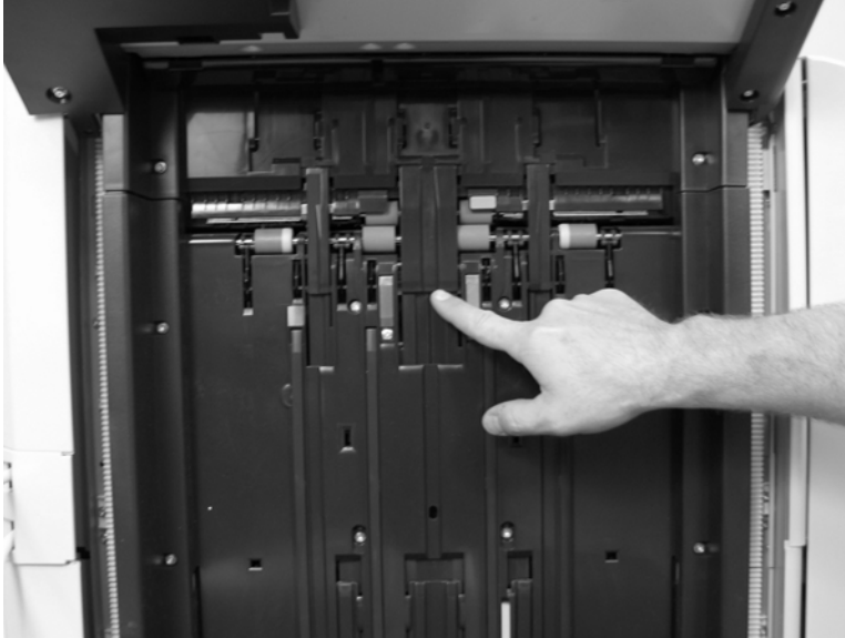
Figure 8-153 Move output bins (1 of 3)
