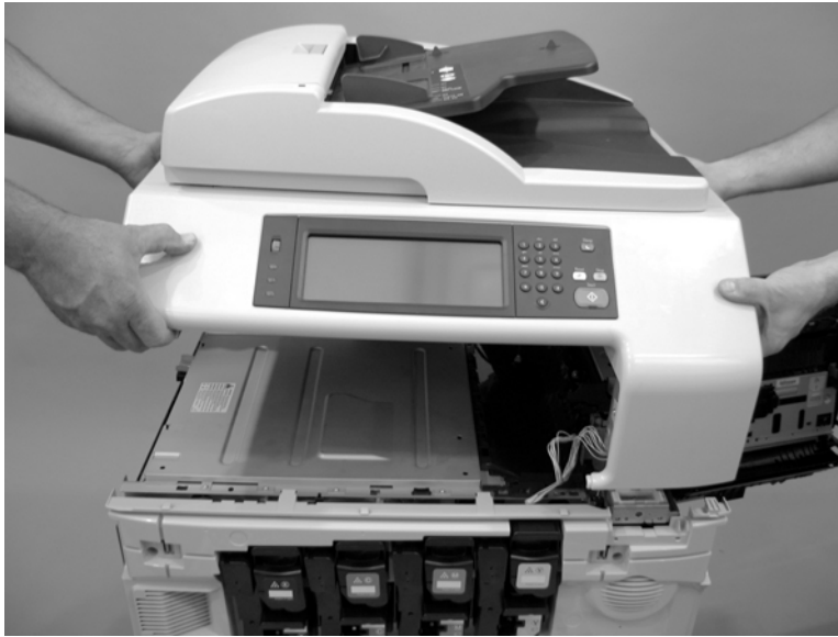
Figure 6-158 Remove optical scanner (6 of 7)
