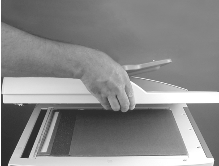
Figure 6-230 Remove the ADF white backing (3 of 4)
