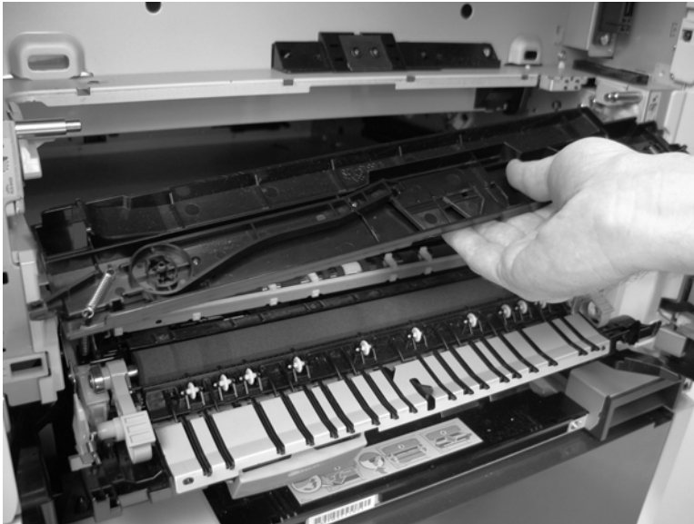
Figure 6-125 Remove the ITB duct (2 of 2)
