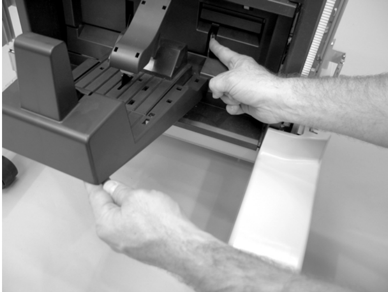
Figure 8-205 Remove booklet-delivery output bin (1 of 2)
