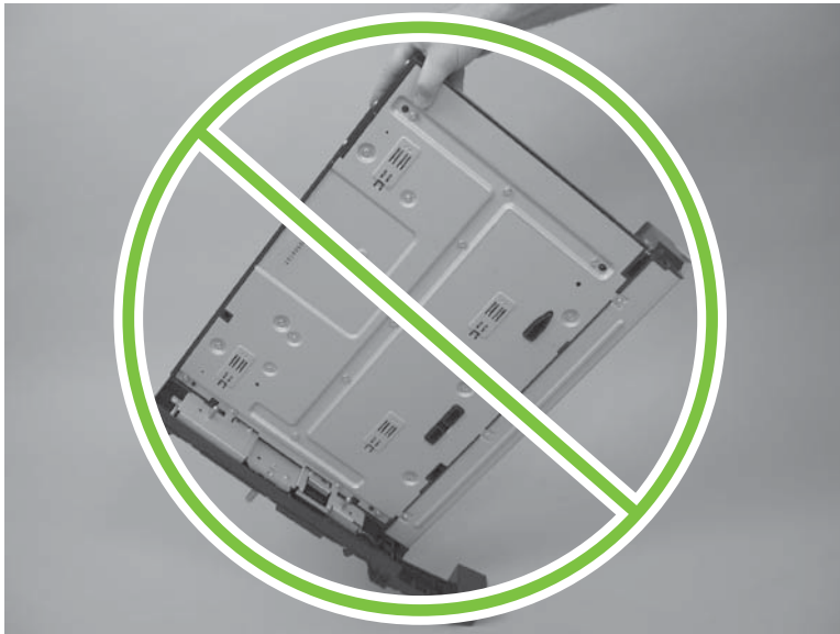
Figure 8-101 Incorrect placement of the IPTU (2 of 2)
