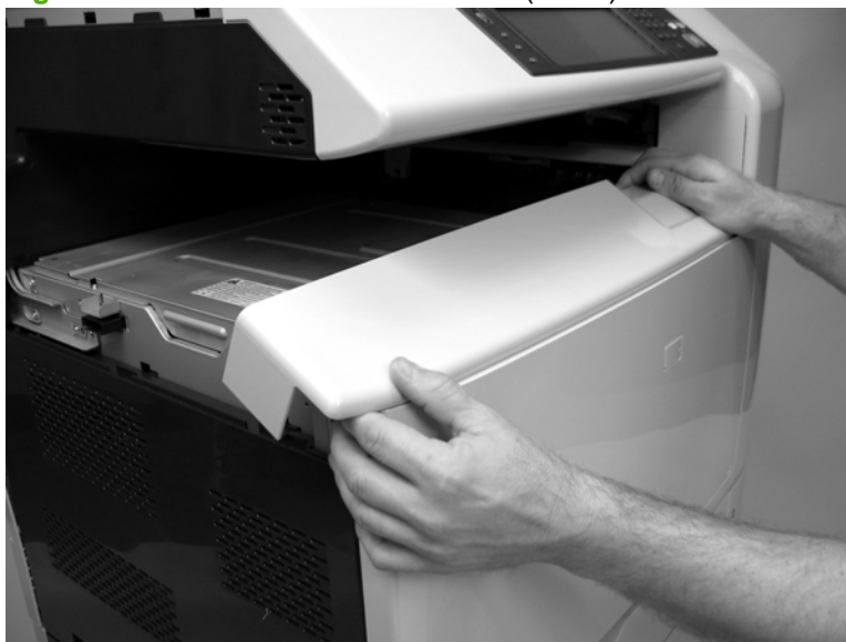
Figure 6-81 Remove front lower cover (2 of 2)
