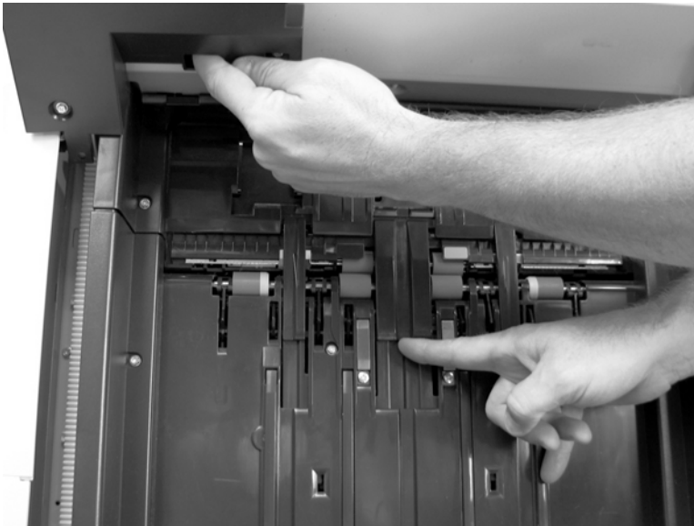
Figure 8-202 Remove output-bin 2 (3 of 3)
