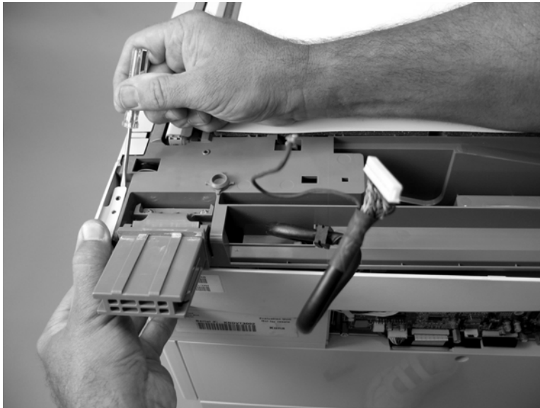
Figure 6-239 Remove the ADF rear end cover (4 of 5)
