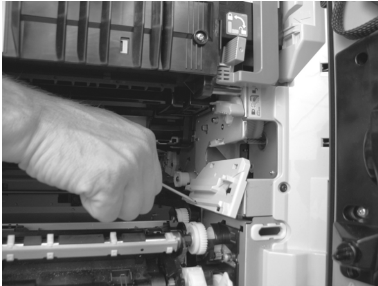
Figure 6-2 Remove the secondary transfer unit (1 of 9)
