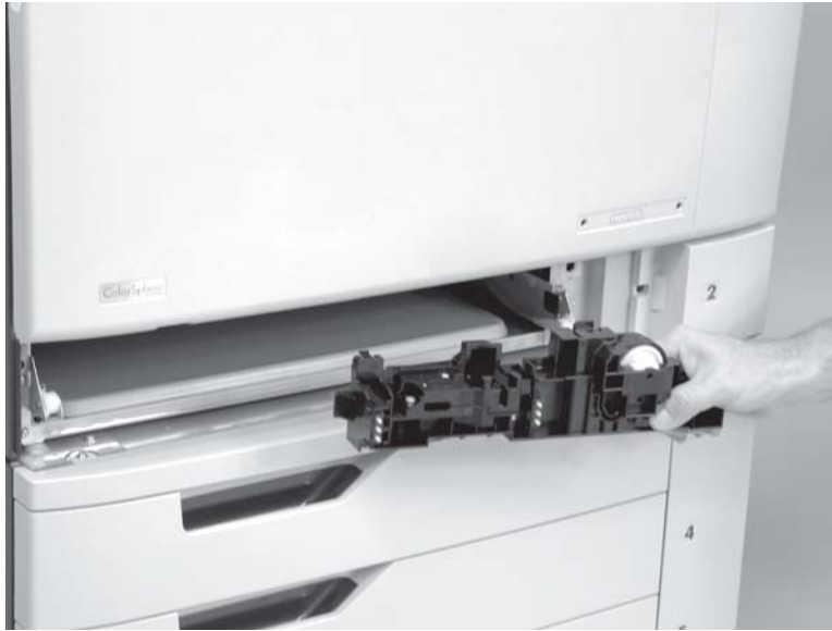
Figure 6-29 Remove the lifter-drive unit (2 of 2)
