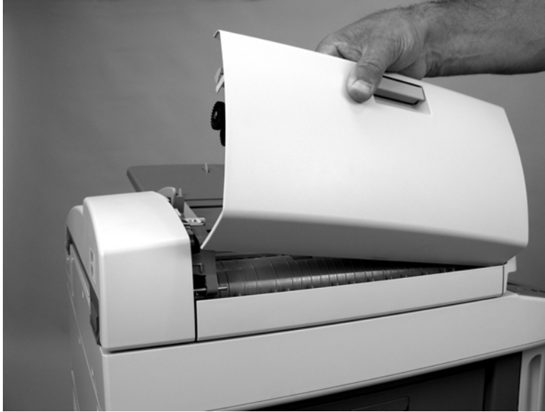
Figure 6-221 Remove the ADF jam cover (3 of 3)
