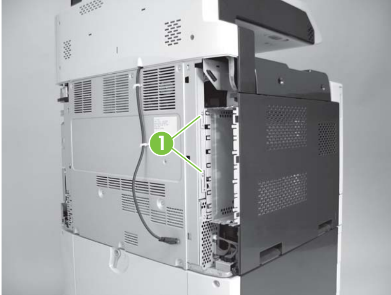
Figure 6-22 Remove rear cover (1 of 2)
