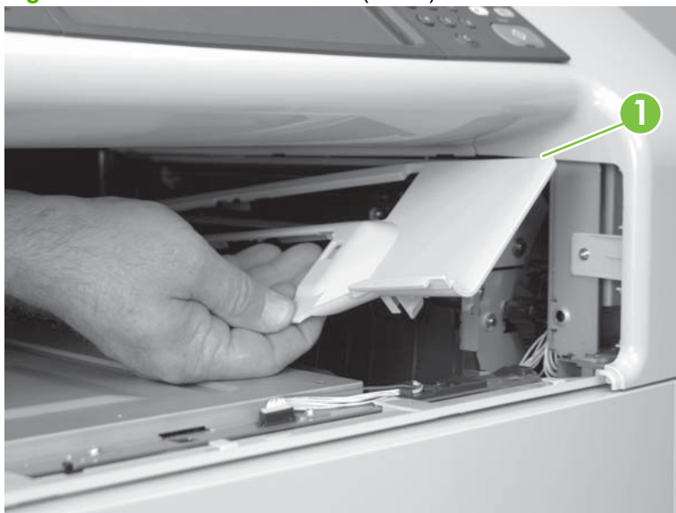
Figure 6-85 Remove inner cover (4 of 4)
