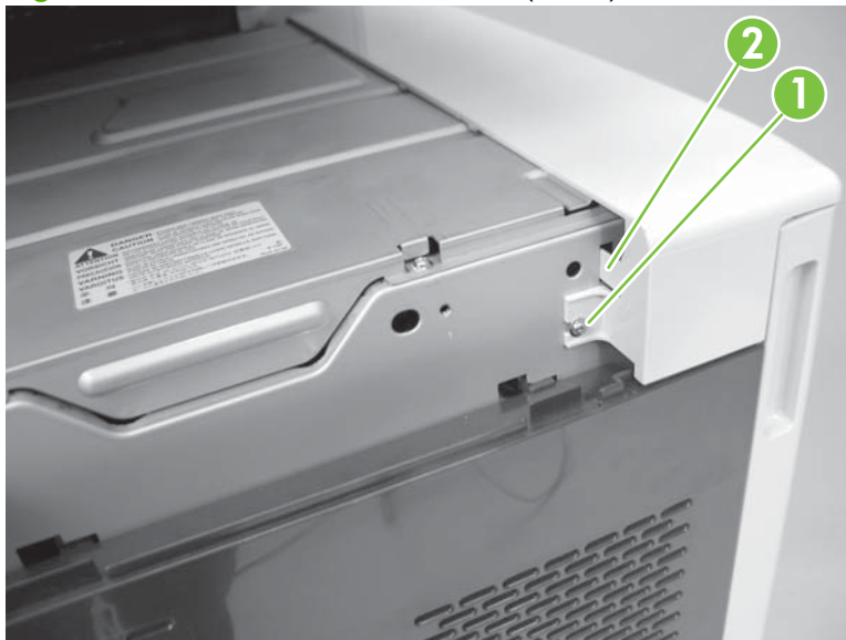
Figure 6-80 Remove front lower cover (1 of 2)
