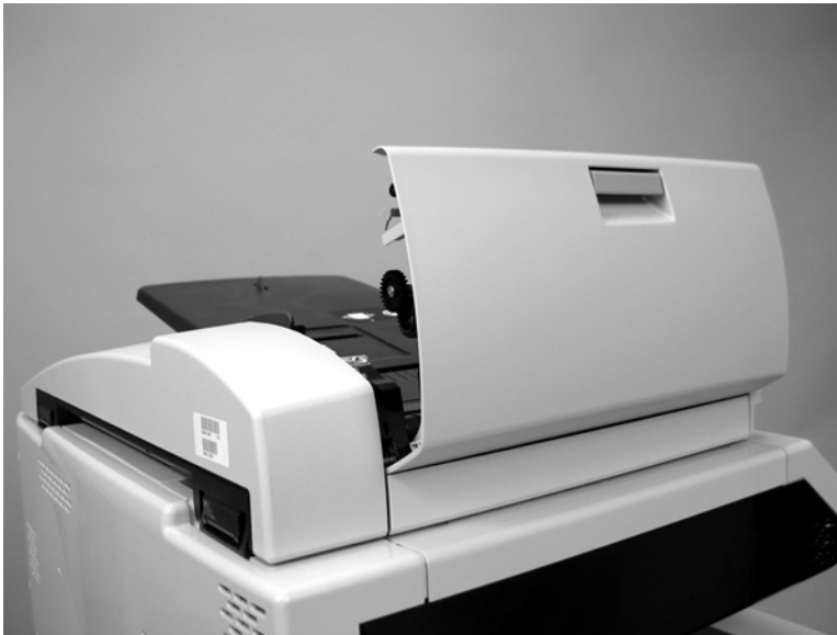
Figure 6-219 Remove the ADF jam cover (1 of 3)
