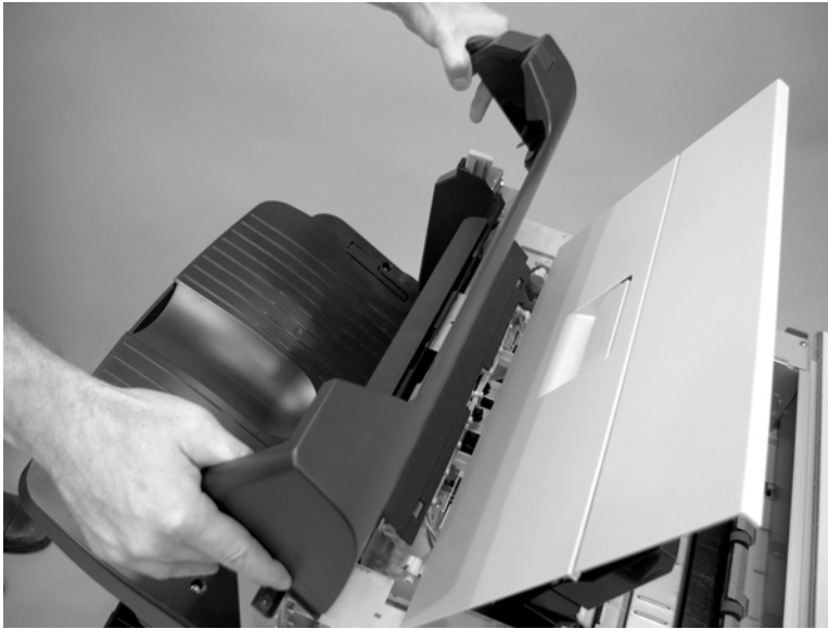
Figure 8-147 Remove the left-upper cover (2 of 3)
