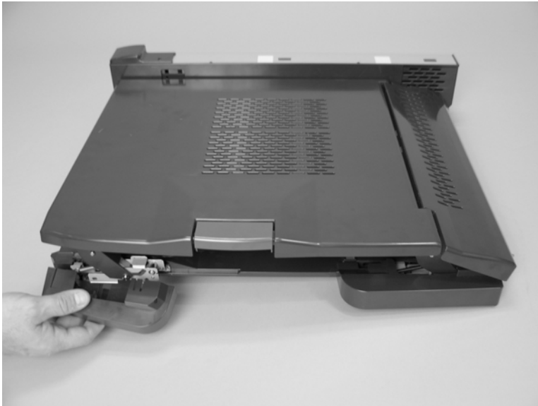
Figure 8-103 Remove upper guide assembly (2 of 5)
