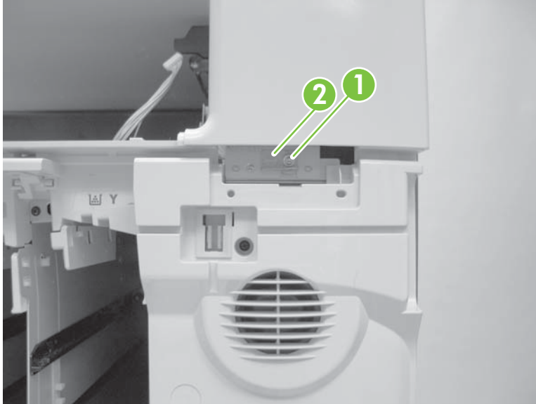
Figure 6-154 Remove optical scanner (2 of 7)
