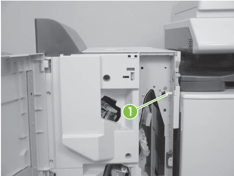
Figure 8-132 Remove output accessory (2 of 5)
