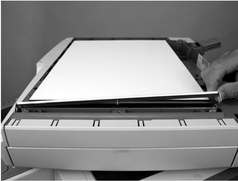
Figure 6-225 Remove the ADF float assembly (3 of 5)
