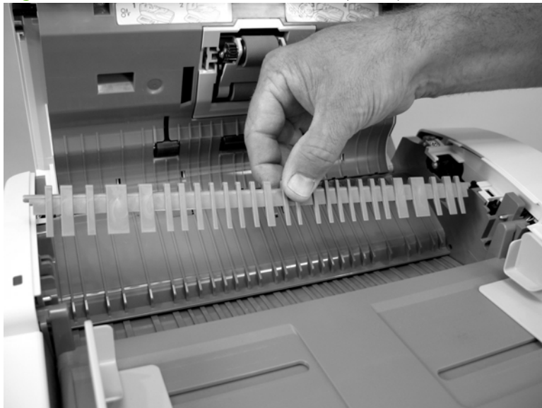
Figure 6-218 Remove the ADF diverter (2 of 2)
