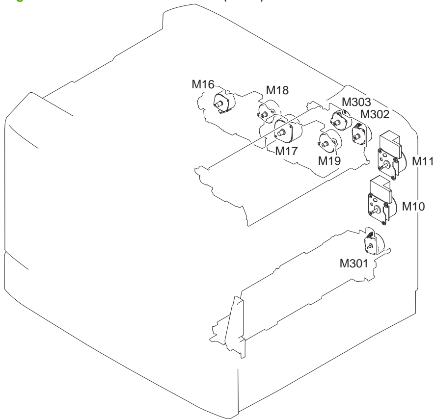
Figure 7-42 Product motor locations (2 of 2)
