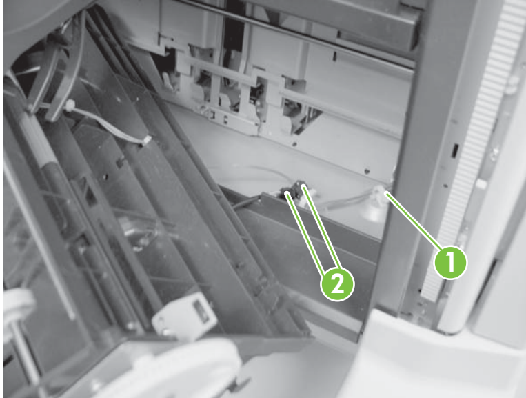
Figure 8-209 Remove the saddle delivery output bin (3 of 3)
