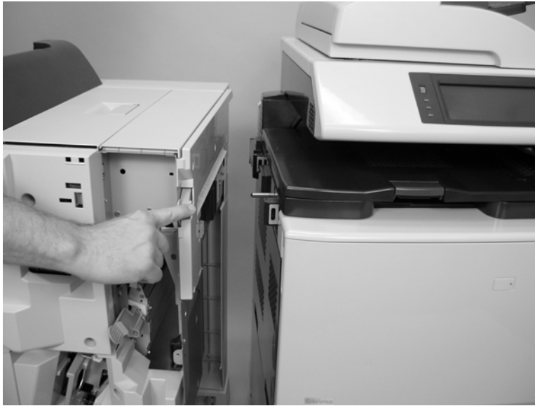
Figure 8-133 Remove output accessory (3 of 5)
