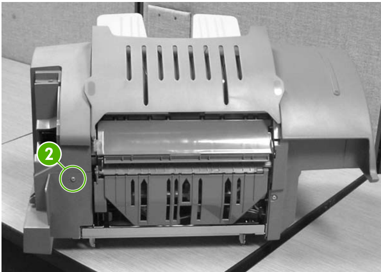
Figure 6-186 Remove the left cover (2 of 2)
