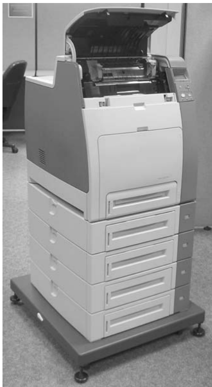
Figure 6-34 Remove the top cover (2 of 7)
