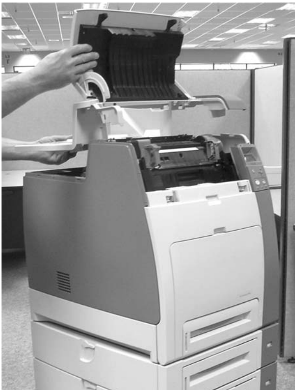
Figure 6-39 Remove the top cover (7 of 7)
