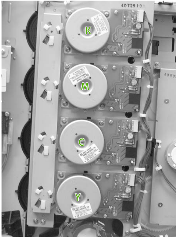
Figure 6-79 Reinstall the main drive assembly (16 of 16)
