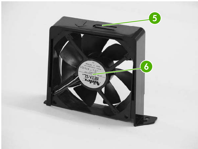
Figure 6-132 Remove the upper exhaust fan (2 of 3)
