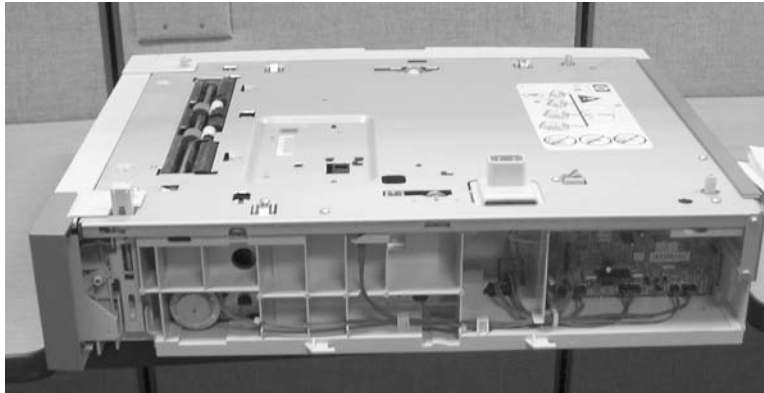
Figure 6-162 Remove the right cover (2 of 2)
