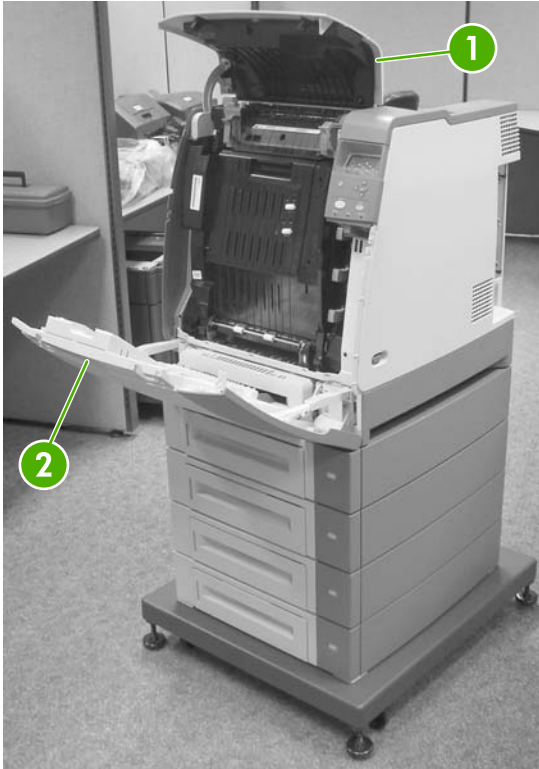
Figure 6-24 Remove the front cover (1 of 6)
