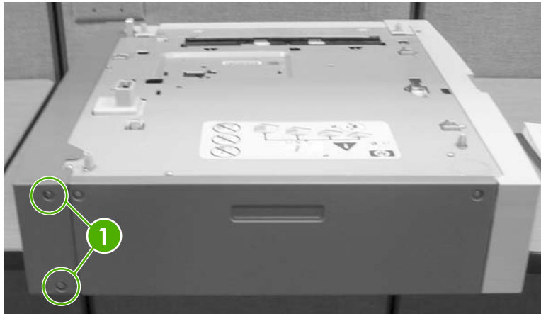
Figure 6-161 Remove the right cover (1 of 2)
