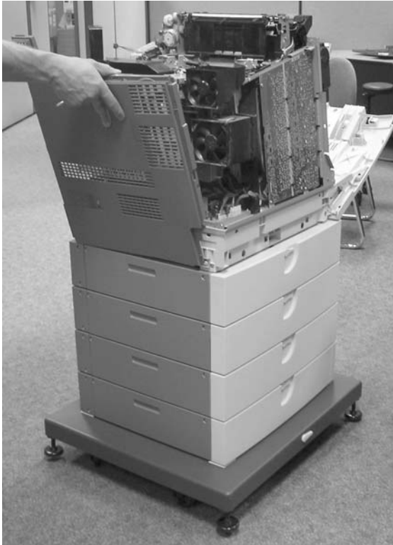
Figure 6-48 Remove the rear cover
