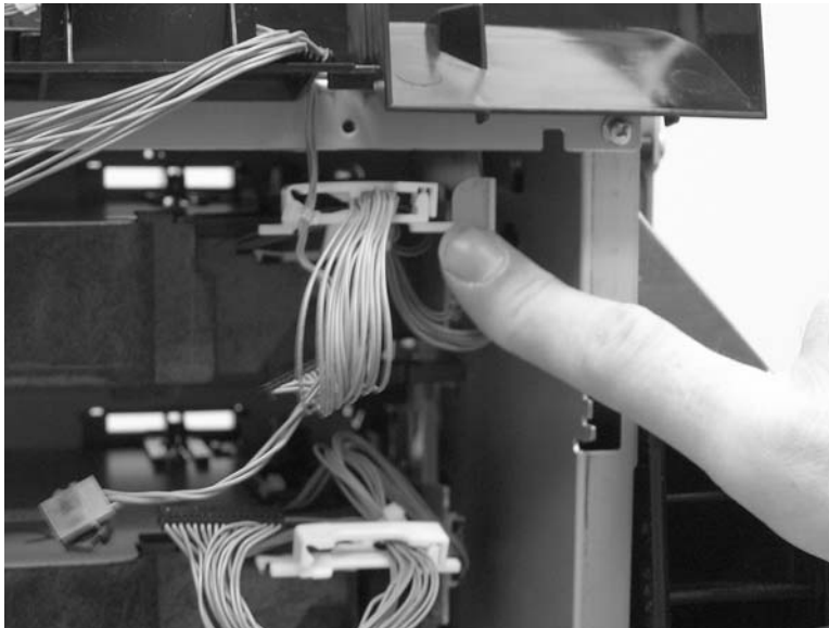
Figure 6-114 Remove the laser/scanner assembly (12 of 17)
