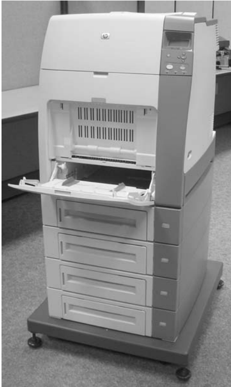
Figure 6-17 Remove the multipurpose tray (1 of 7)
