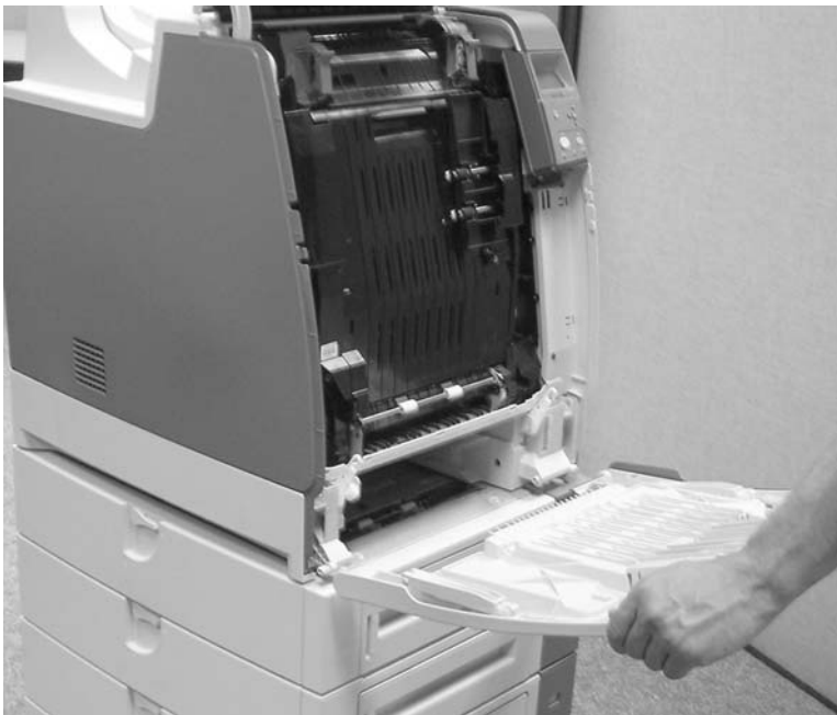
Figure 6-29 Remove the front cover (6 of 6)
