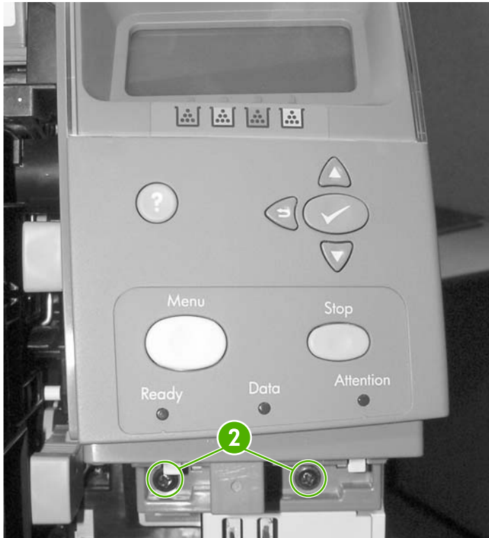
Figure 6-50 Remove the control panel (2 of 3)
