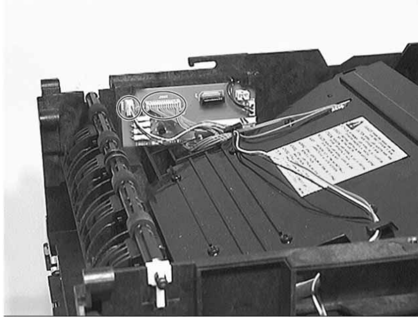
Figure 7-96 Disconnecting Laser Scanner's and Fan's Power Cable
