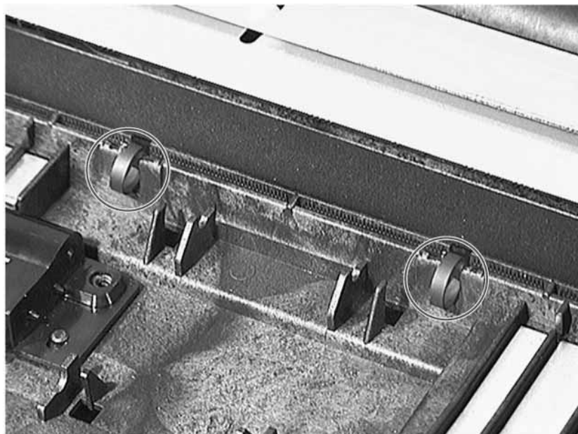
Figure 7-67 Installing the A-1 Belt and Roller
