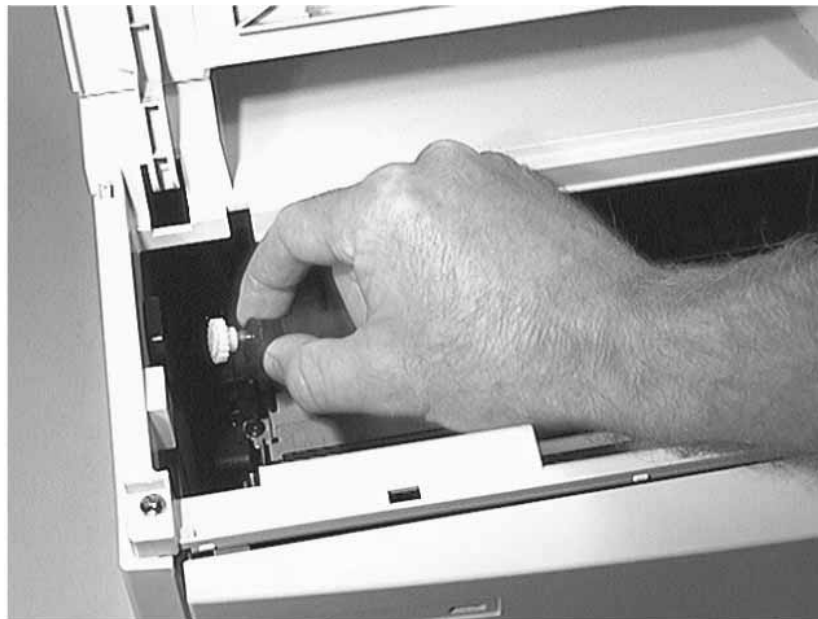
Figure 7-6 Removing the Transfer Roller (2 of 2)
