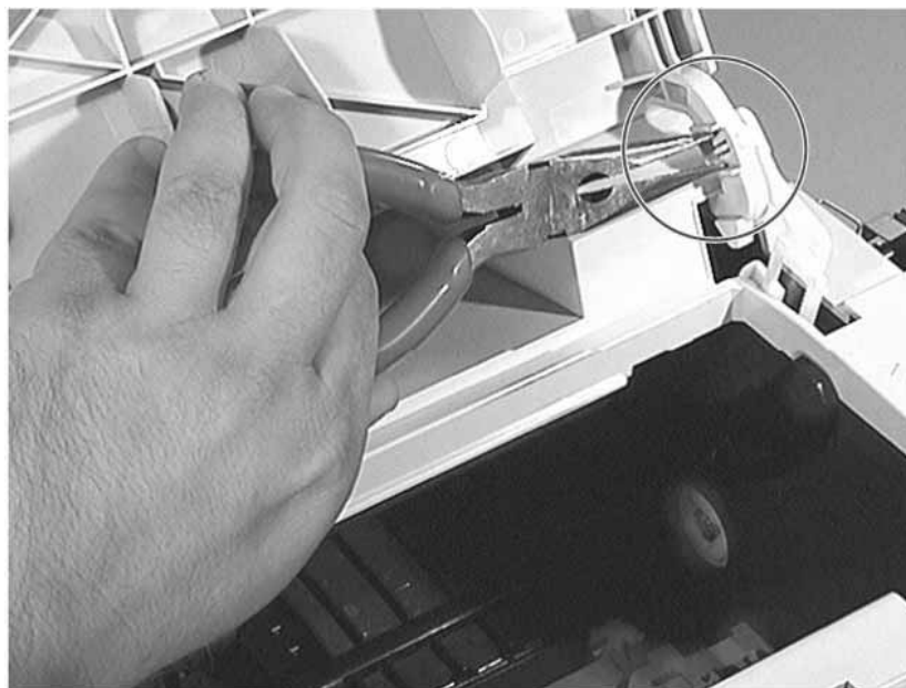
Figure 7-51 Releasing Swing Arm from Toner Cartridge Door
