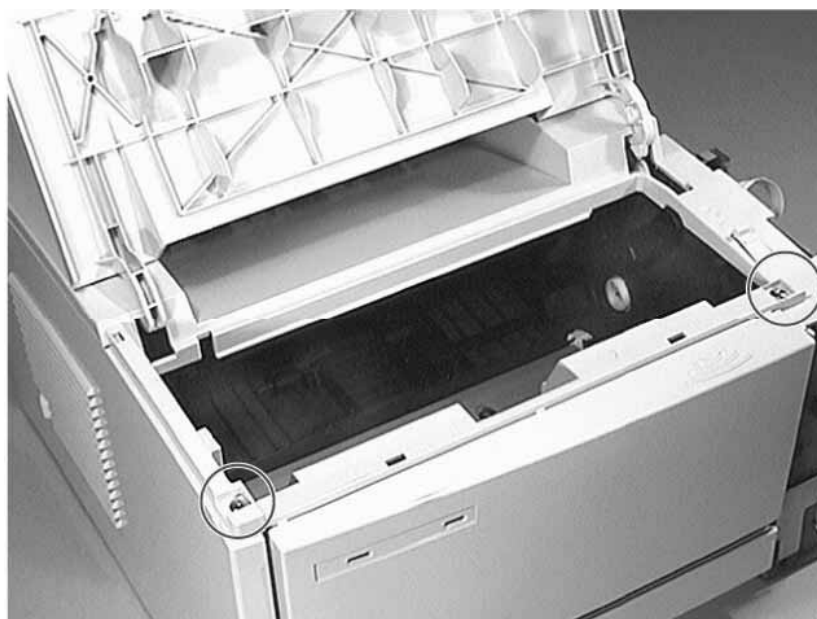
Figure 7-52 Removing Screws from the Top Cover (1 of 2)
