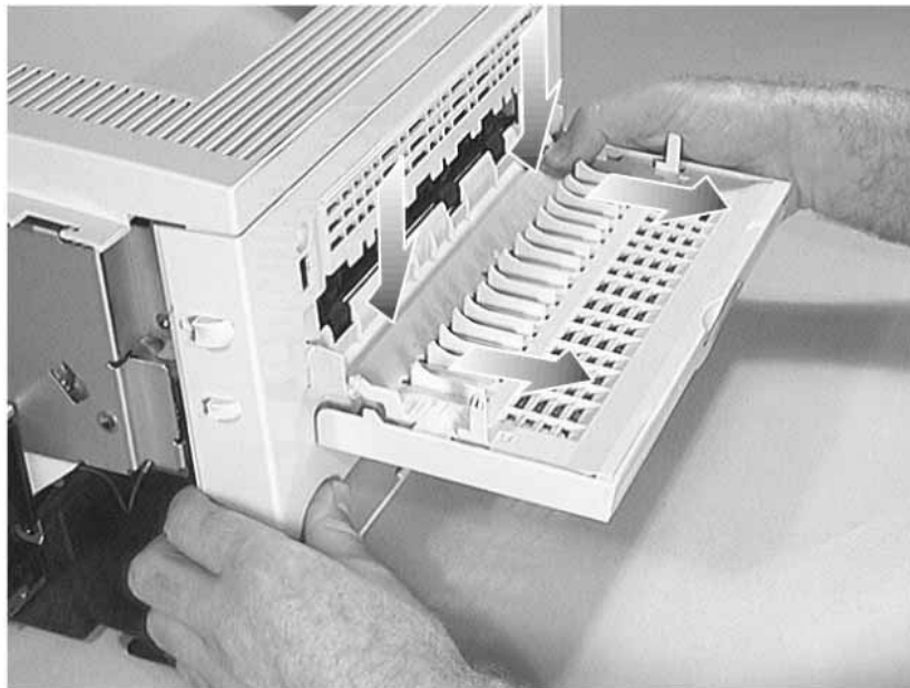
Figure 7-33 Removing the Rear Cover
