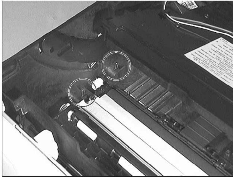
Figure 7-121 DC Bias Voltage Contacts (Leaf Springs)
