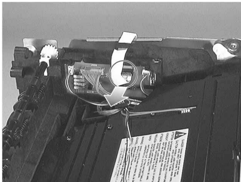
Figure 7-61 Disconnecting Power Cables
